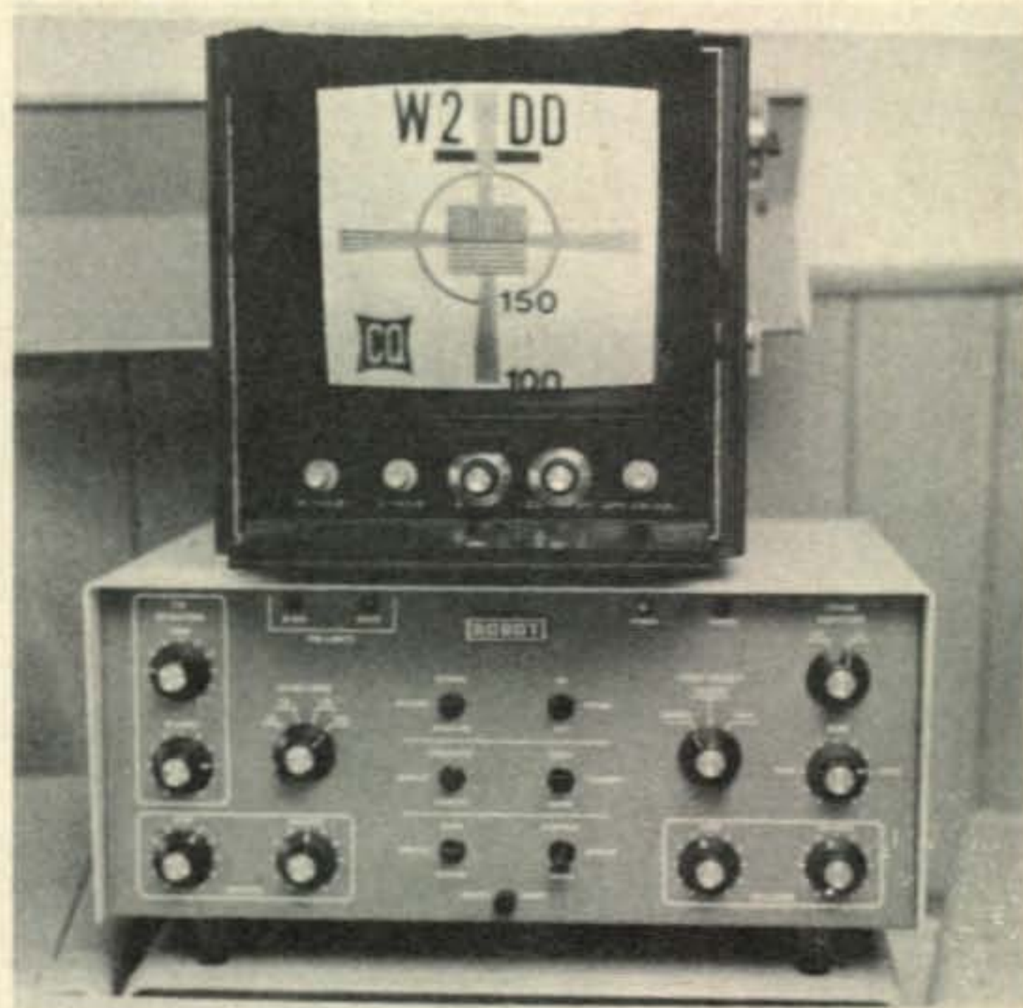
The image obtained using the Robot Model 300 and a resolution chart at W2DD.
