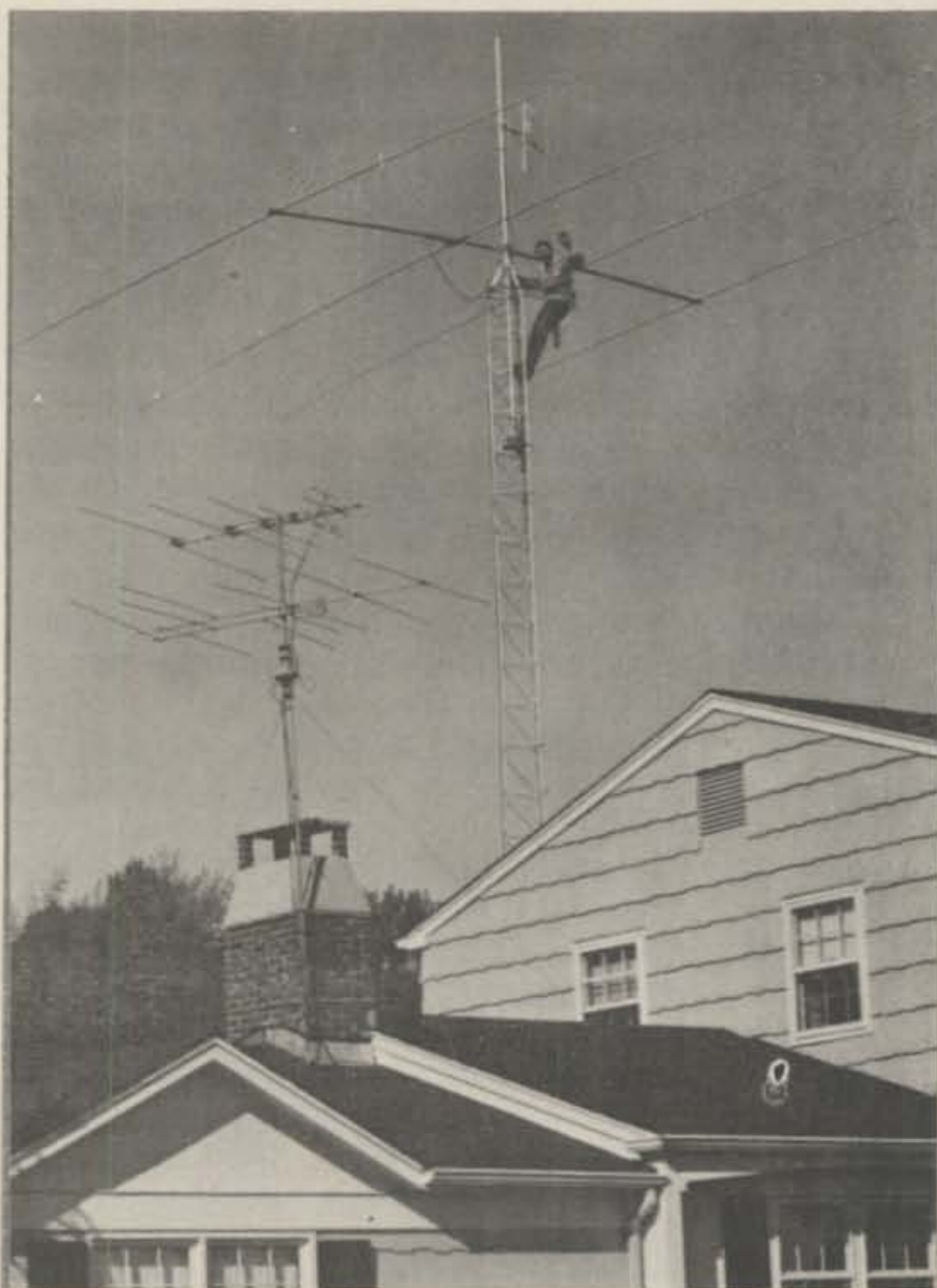
The antenna at W2GRR—four elements on 20 meters at about 40 ft. It isn't much, considering some of the aluminum the big-gun KW's push to 100 ft. or more! Like the Old Man said: "it's the man at the key that counts!"
