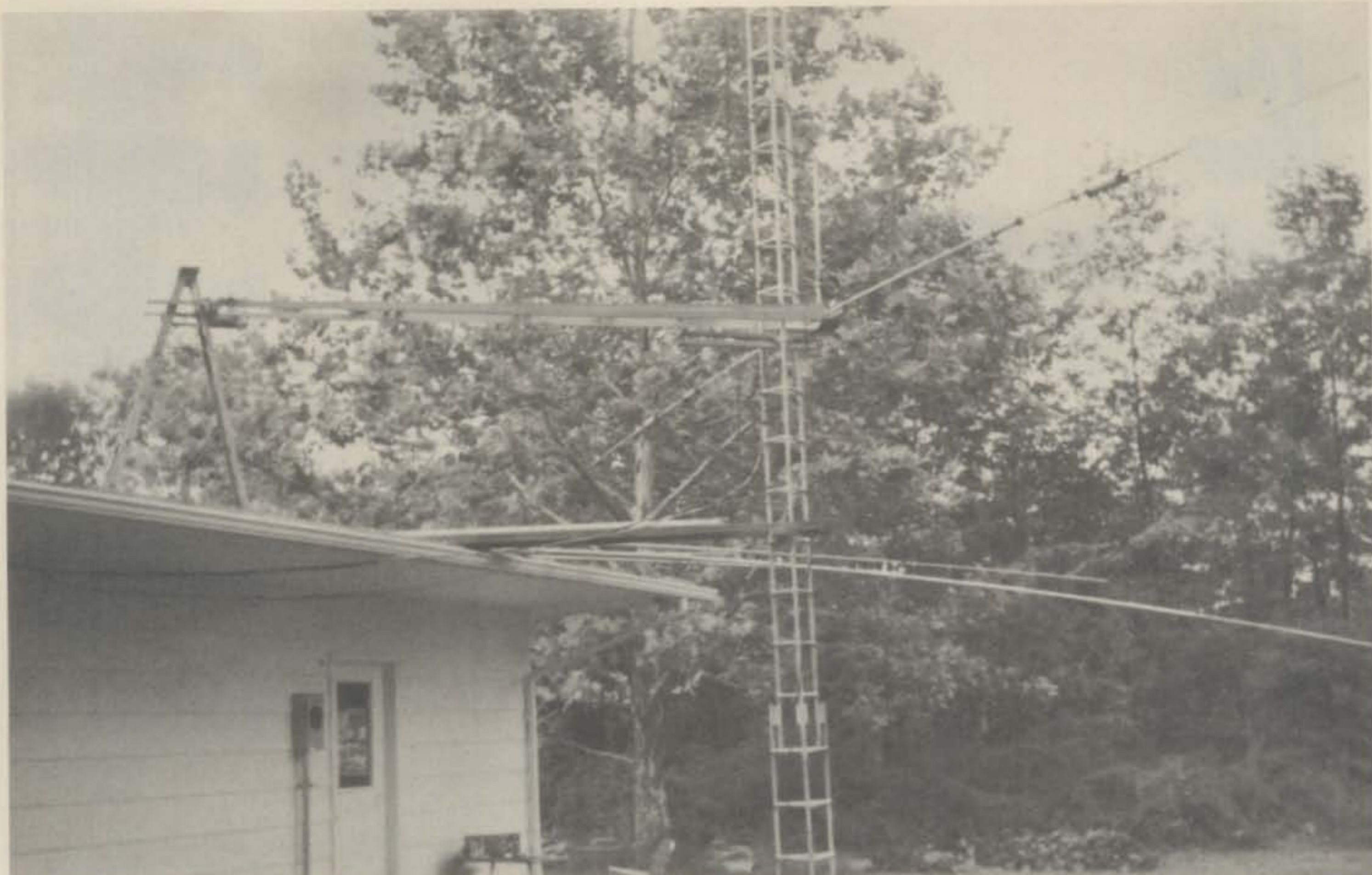
The experimental transmitting antenna setup used at W9LT. Elements for the various bands were placed atop the trellis section extending between the tower and the house. The receiving antenna was a dipole located 750 feet away.
