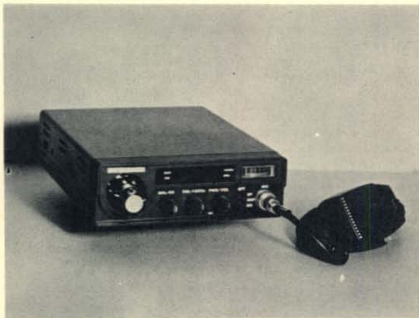
The Tempo VHF/ONE 2 meter f.m. transceiver offers s.s.b. operation with the addition of an optional adaptor. The rig is fully synthesized and uses an LED display for frequency readout. (Photos by Sandra K. Paul)
