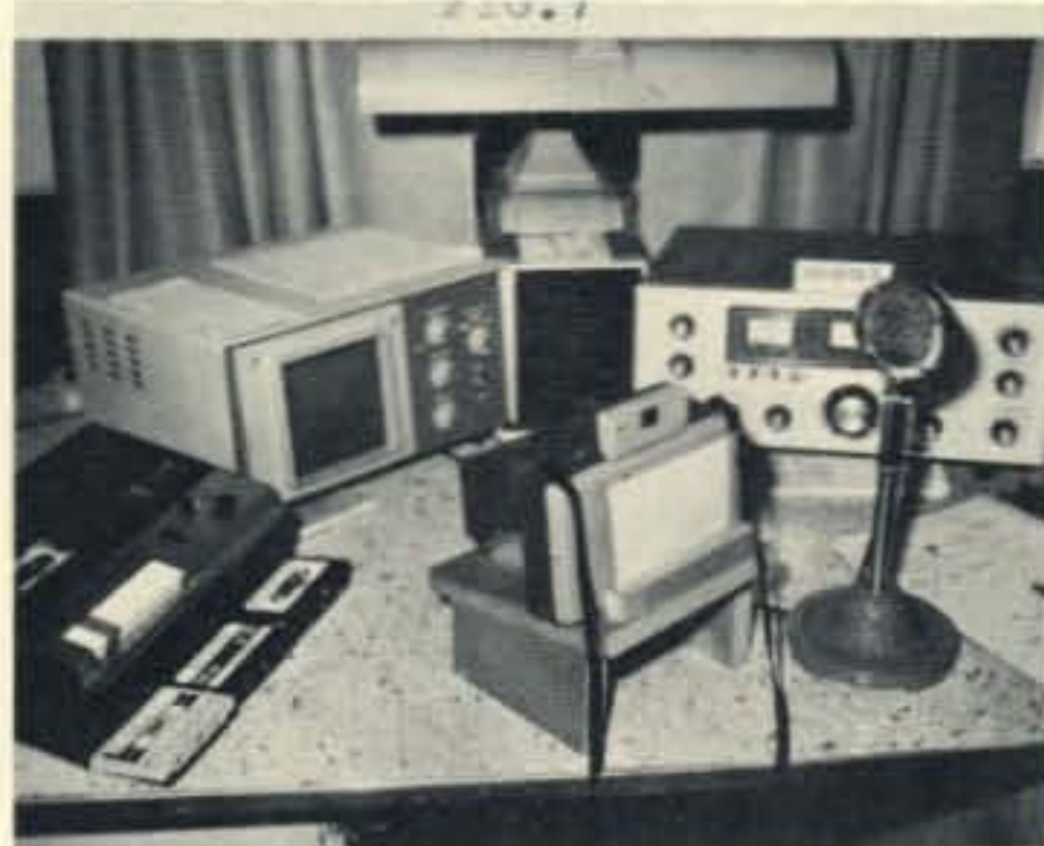
Fig. 7—W8QZ's station, showing home-brew camera mount used in photographing SSTV monitor screen.
