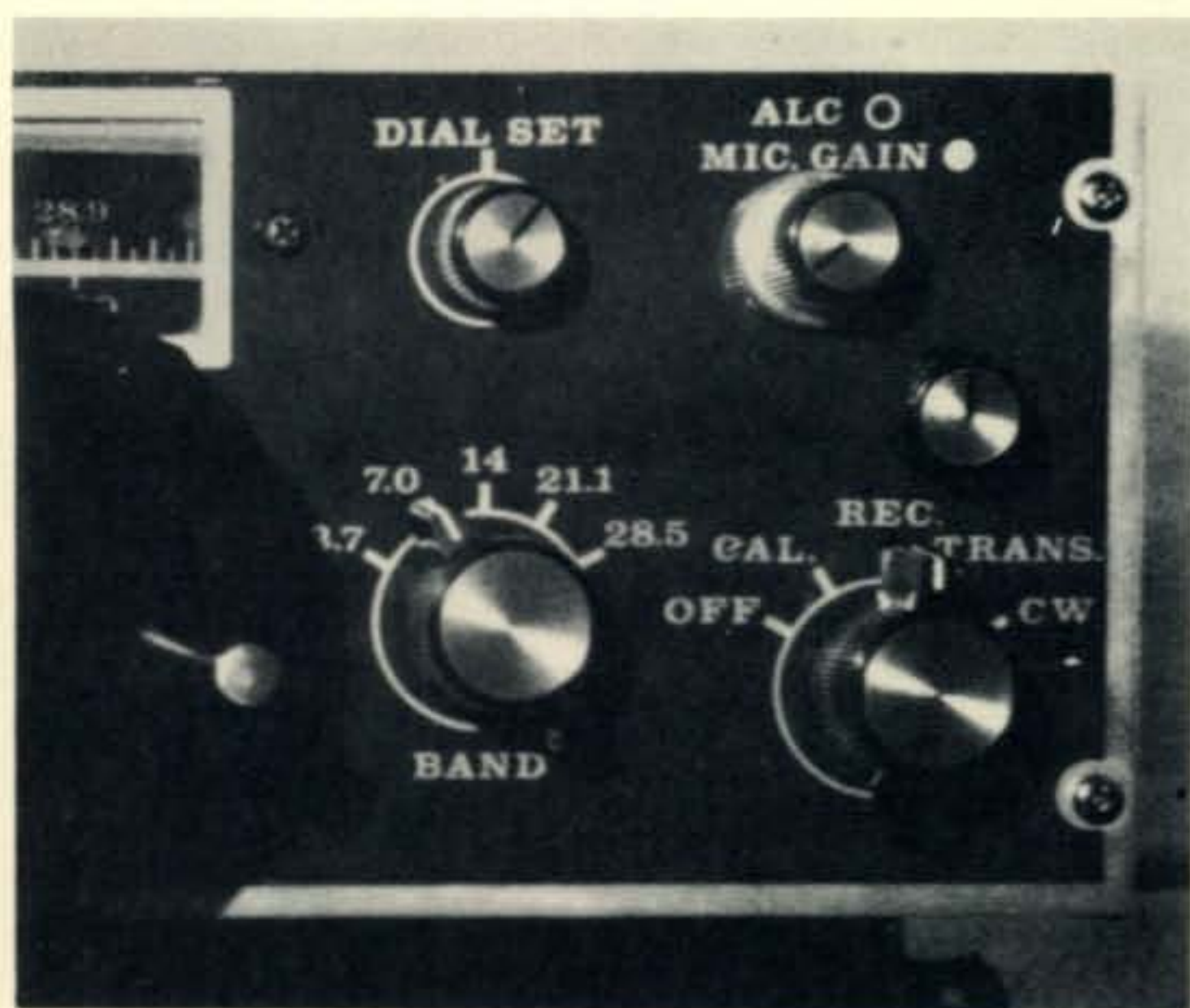
Receiver Incremental Tuning control knob fits nicely into the front panel layout of this Atlas 210, just above the Mode switch.
