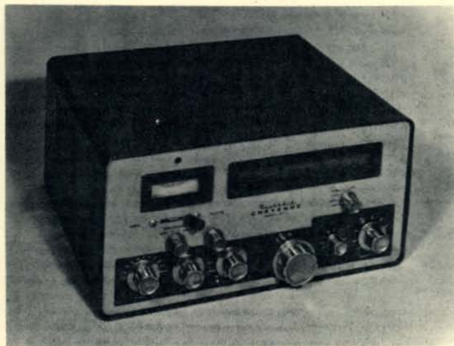
Overall view of the modified Cheyenne shows no changes except the addition of the Drive Level control to the right of the Spotting switch and below the word "Plate."
