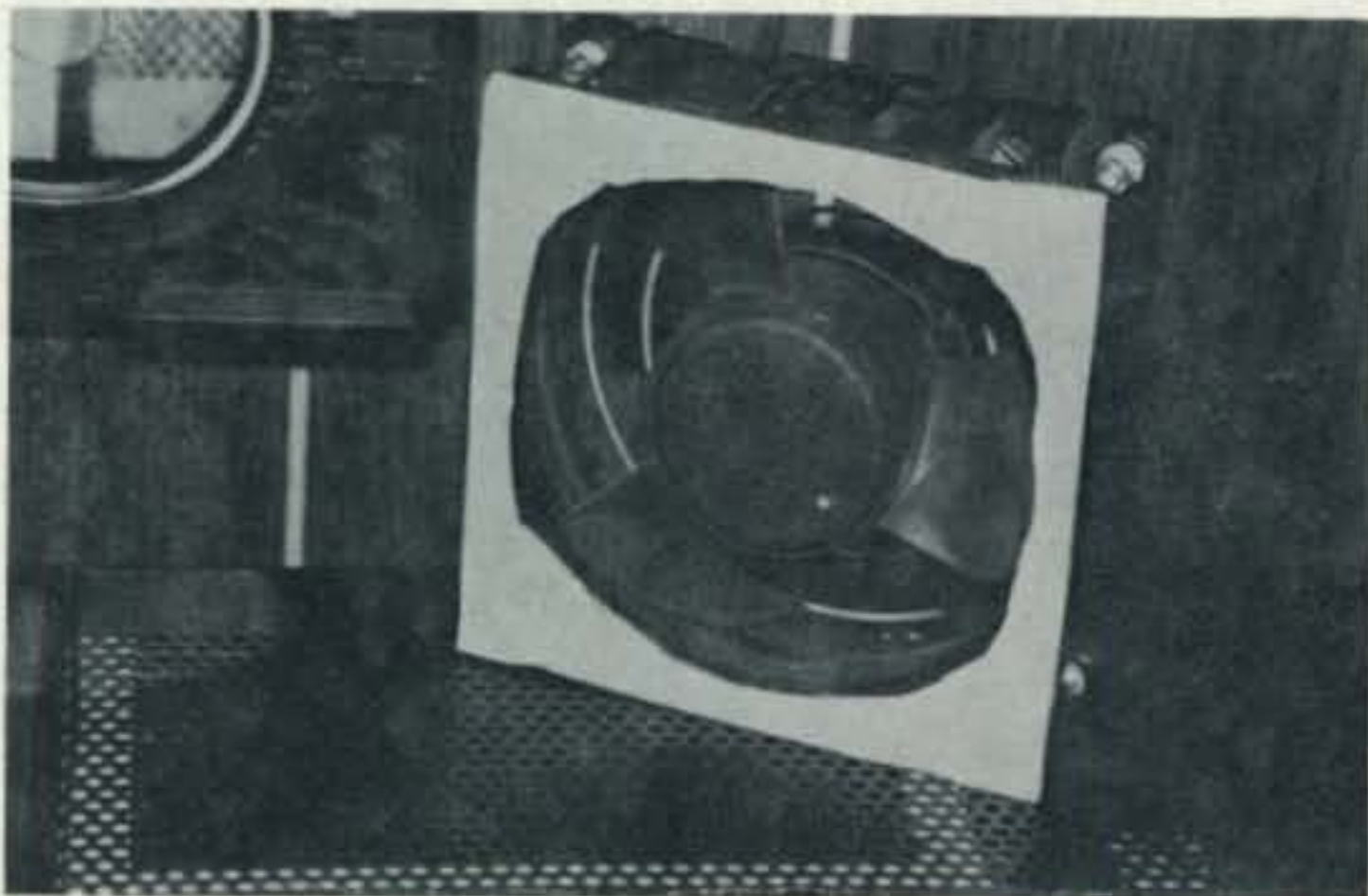
Self-adhesive foam applied to the rim of the muffin-type fan provides air seal.
