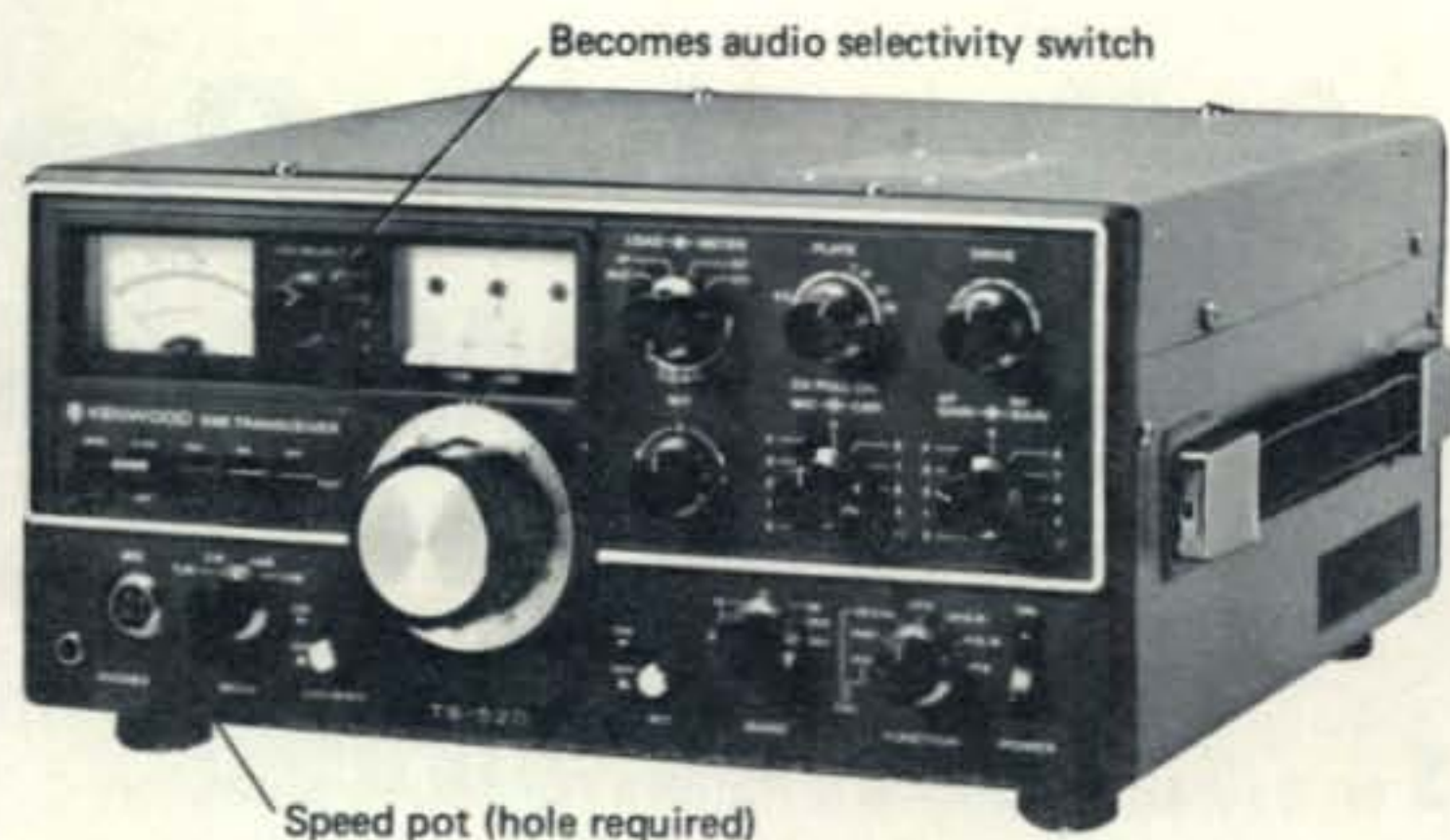
Front view of the TS-520 showing the location of the Speed pot for the Curtis 8043 IC keyer.
