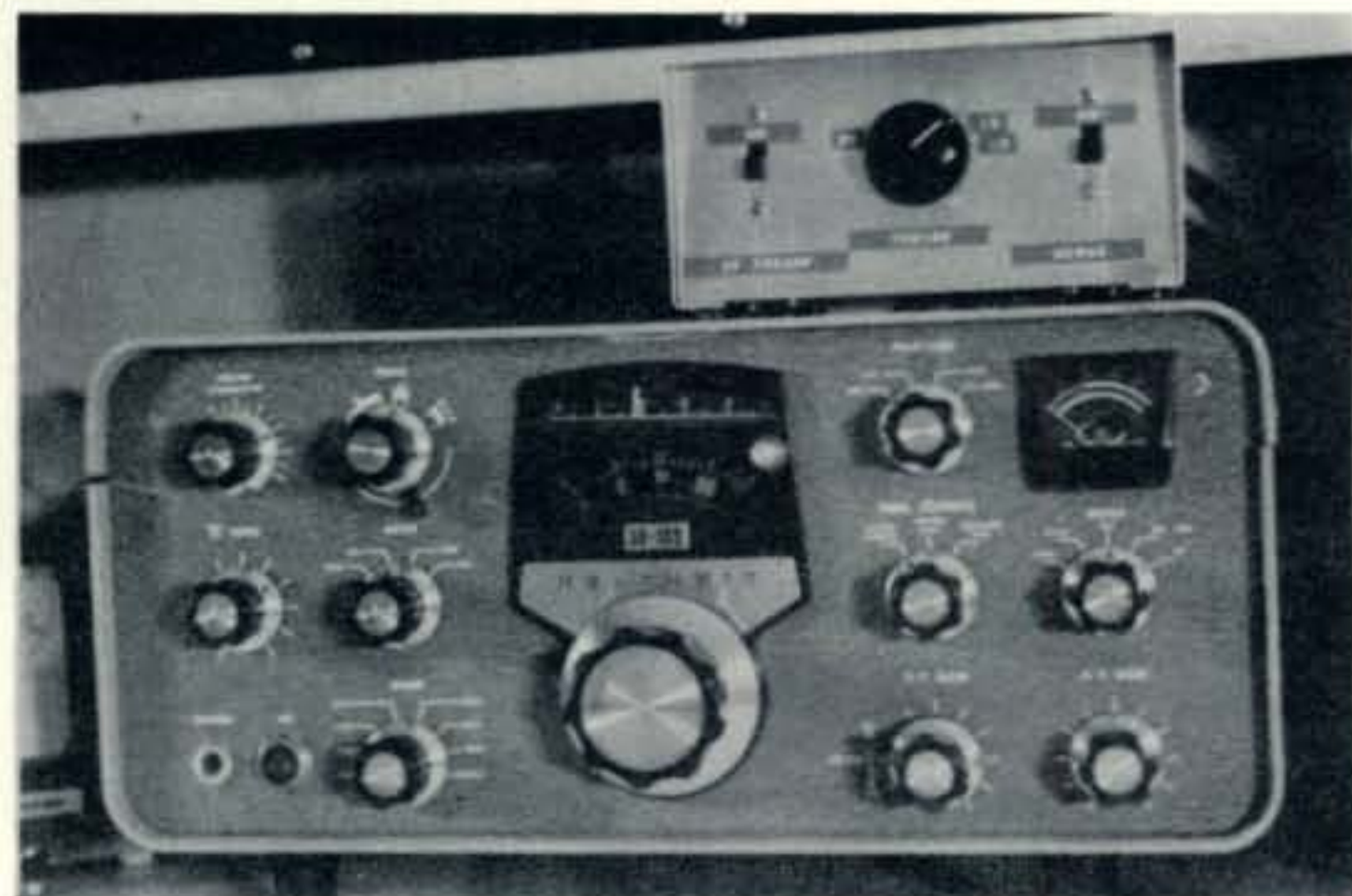
The author's receiver preamp sits above the SB-102 at the shack of W2GQK. Front panel controls consist of two slide switches for Preamp In-Out (both must be operated together), and a Tuning control to peak the single tuned circuit.
