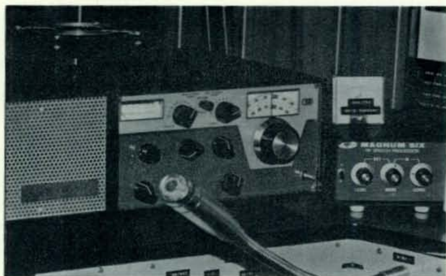
An exciter grid current meter sits atop the Magnum Six RF Speech Processor. The muffin-type cooling fan can be seen on the T-4XB.
