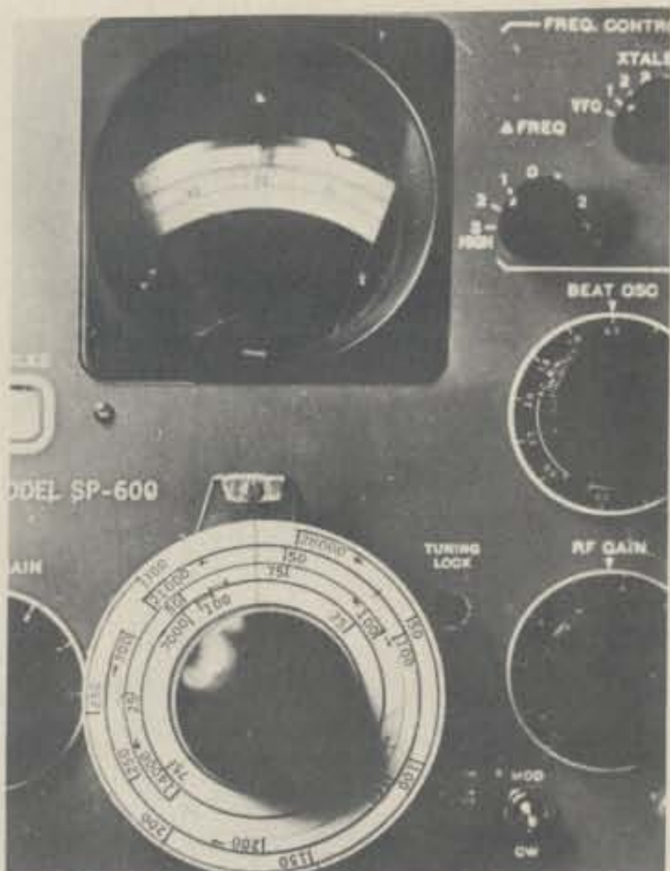
The new calibrated dial is now in place and you're ready to go.
