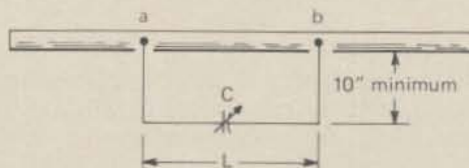
Fig. 1—Representative half-wave dipole or driven element of parasitic beam designed for two frequency operation. Capacitor C in conjunction with the inductance L between points a-b provides a resonance from 0.5 to 1.0 octave above the fundamental frequency. Connections to the capacitor are made with tubing of 1/4-inch to 1/2-inch diameter for a tubing element of 1 1/4-inch diameter. For 14 MHz, the distance a-b is about 7 feet and capacitor C is about 90 pF.
