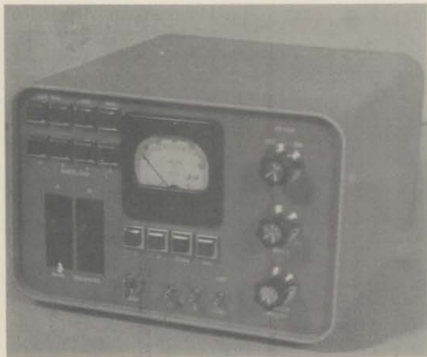
The author's a.c. control center. The cabinet and knobs were purchased from Heathkit to match his existing Heathkit equipment. Complete control details are given in the text.
