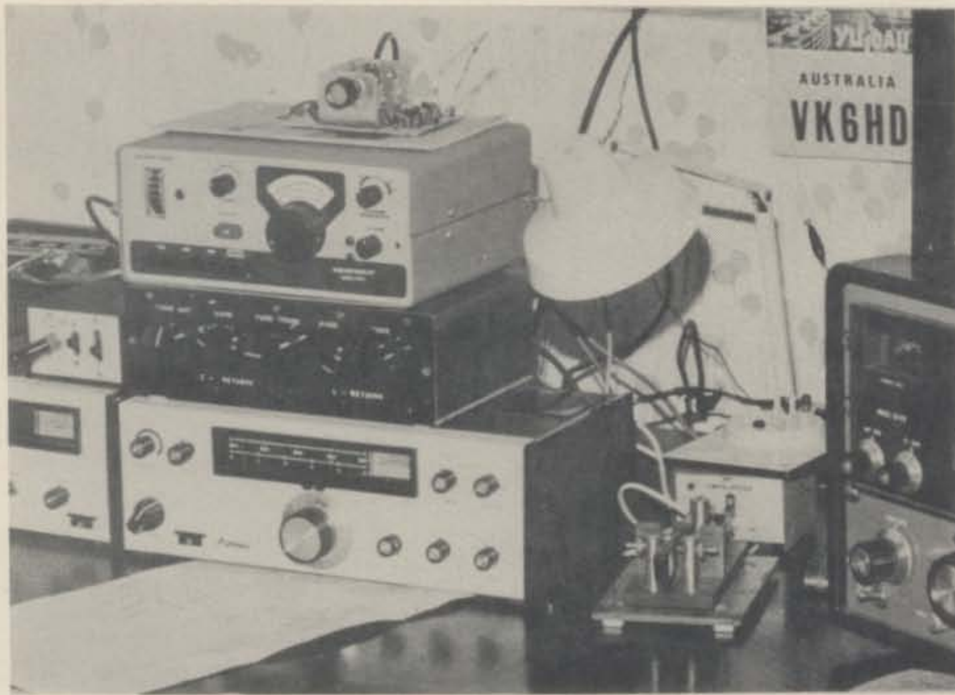
The QRPp position at W4AWS. The Argo and linear (left, partially shown), topped by a Z-L network universal antenna transmatch. The receiver section of the HW-7 is helped by Art's homebrew preselector sitting on the HW-7. Art was the southern-most check-in (except for a KP4) on the 80 meter QRPp Net during the winter-spring of 1974-75. He used a 40 meter dipole fed thru the L-network transmatch with good results. He had severe static problems most of the time, but managed to copy many of us.
