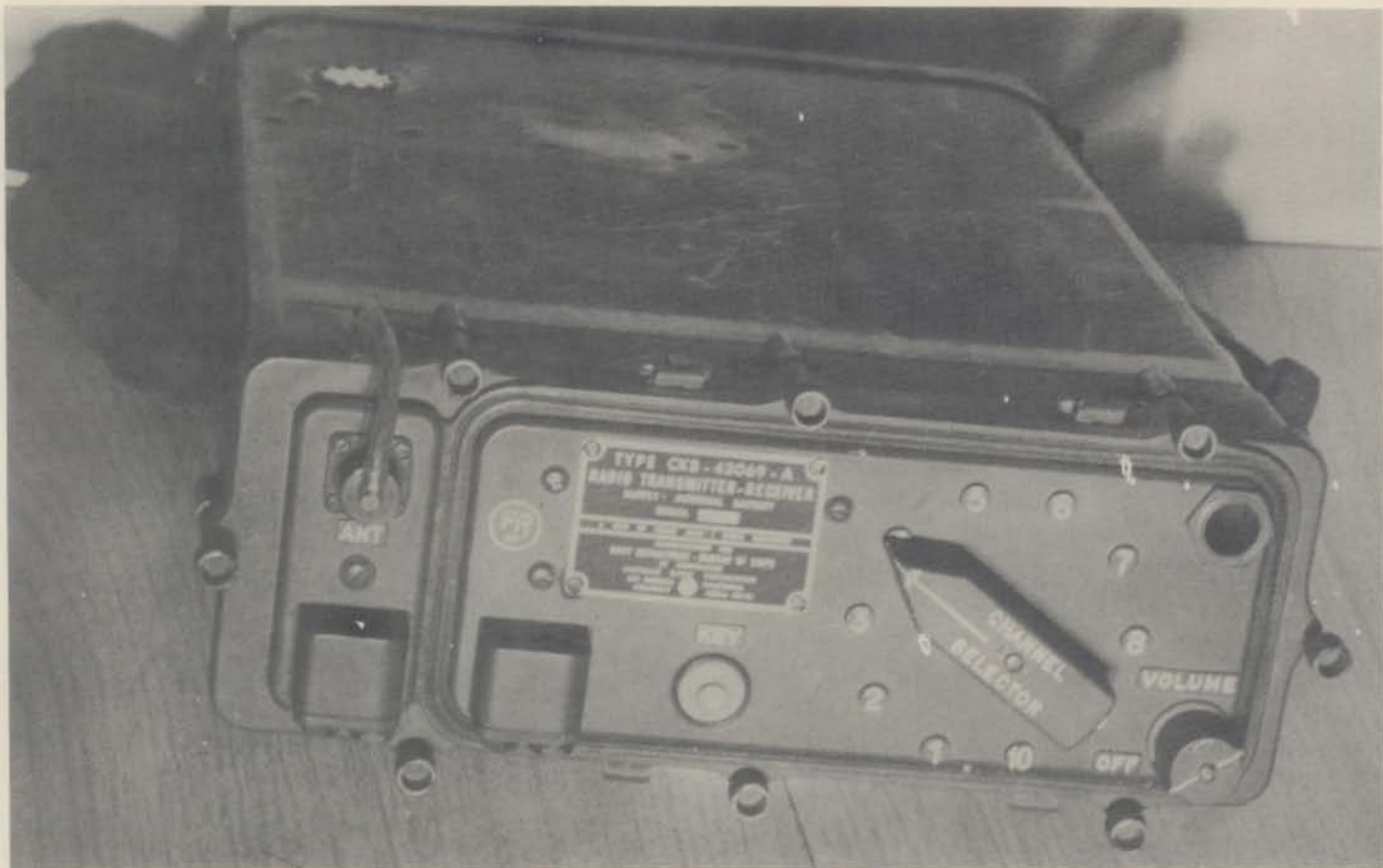
The MAW walkie-talkie. This set has ten pre set crystal controlled channels in the range of 115-156 MHz. No modification of the r.f. circuits is needed to put it on 2 meters.
