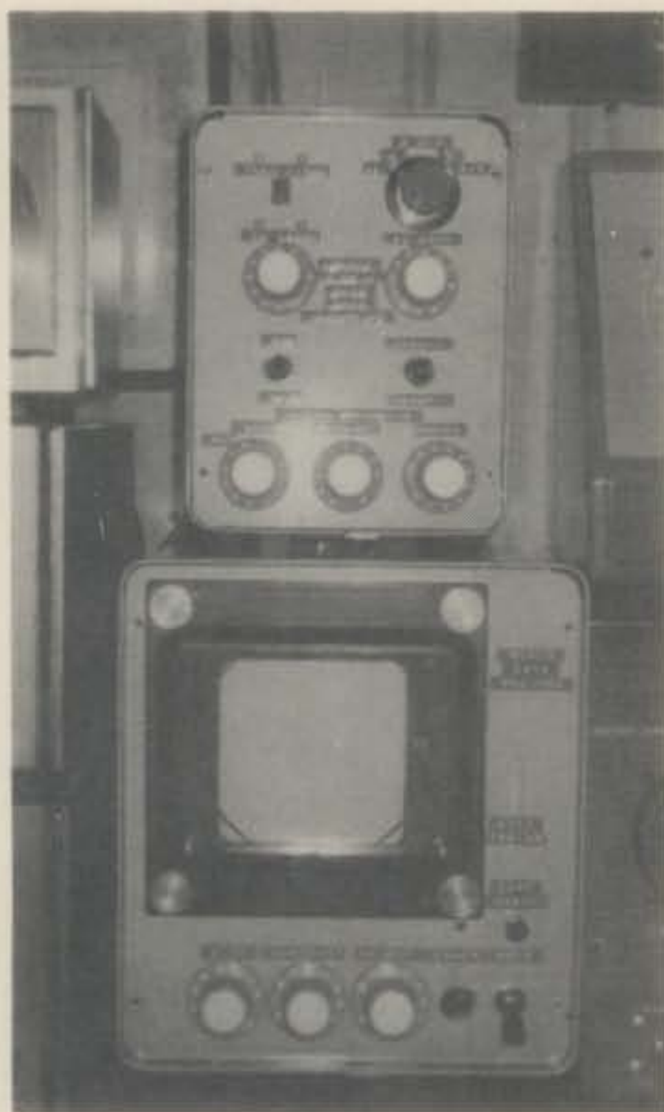
Front view of direct view storage tube monitor constructed by W5DFU.
