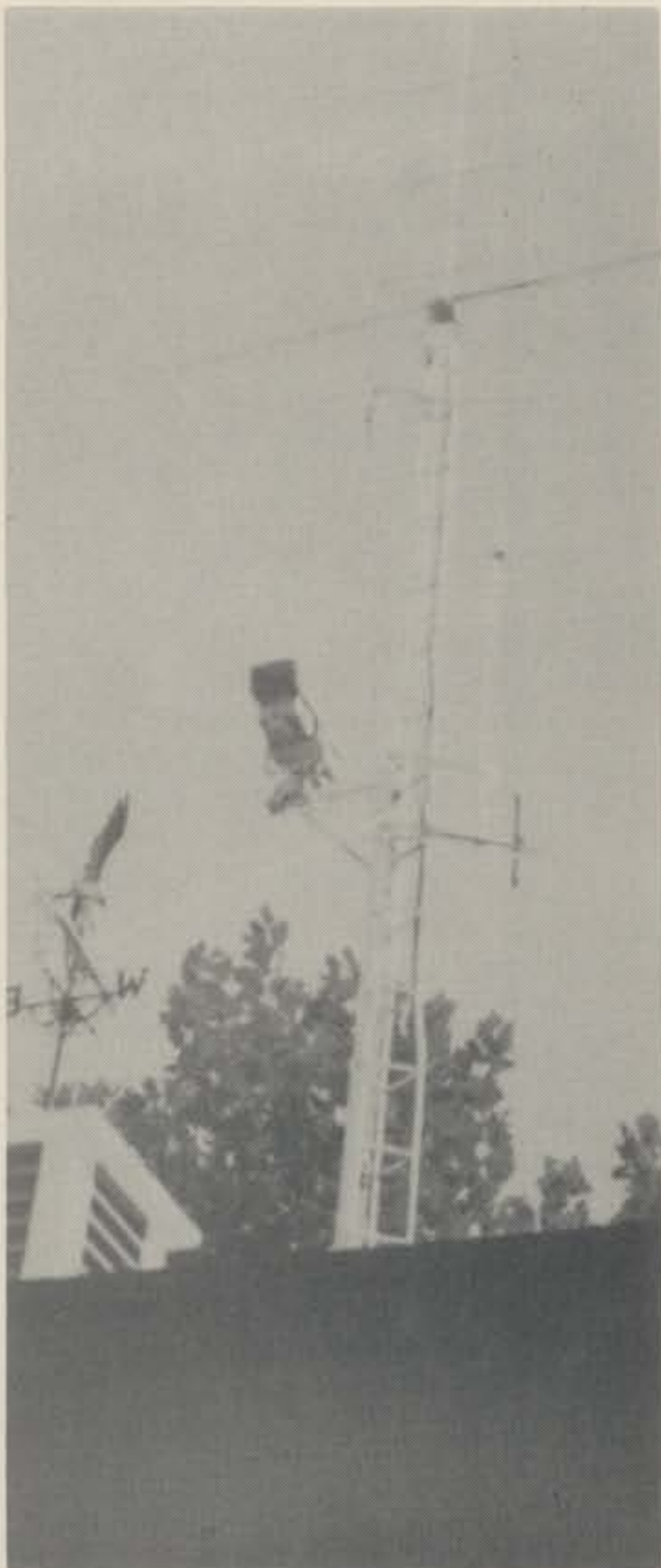
Remote operated fast scan camera used by W5DFU for weather watch project.
