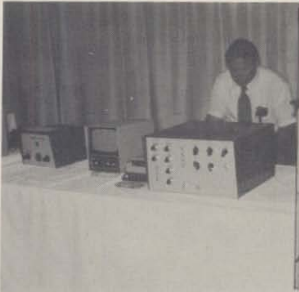
Scan converter designed and built by Dr. George Steber, WB9LVI. George believes in a minimum number of controls.
