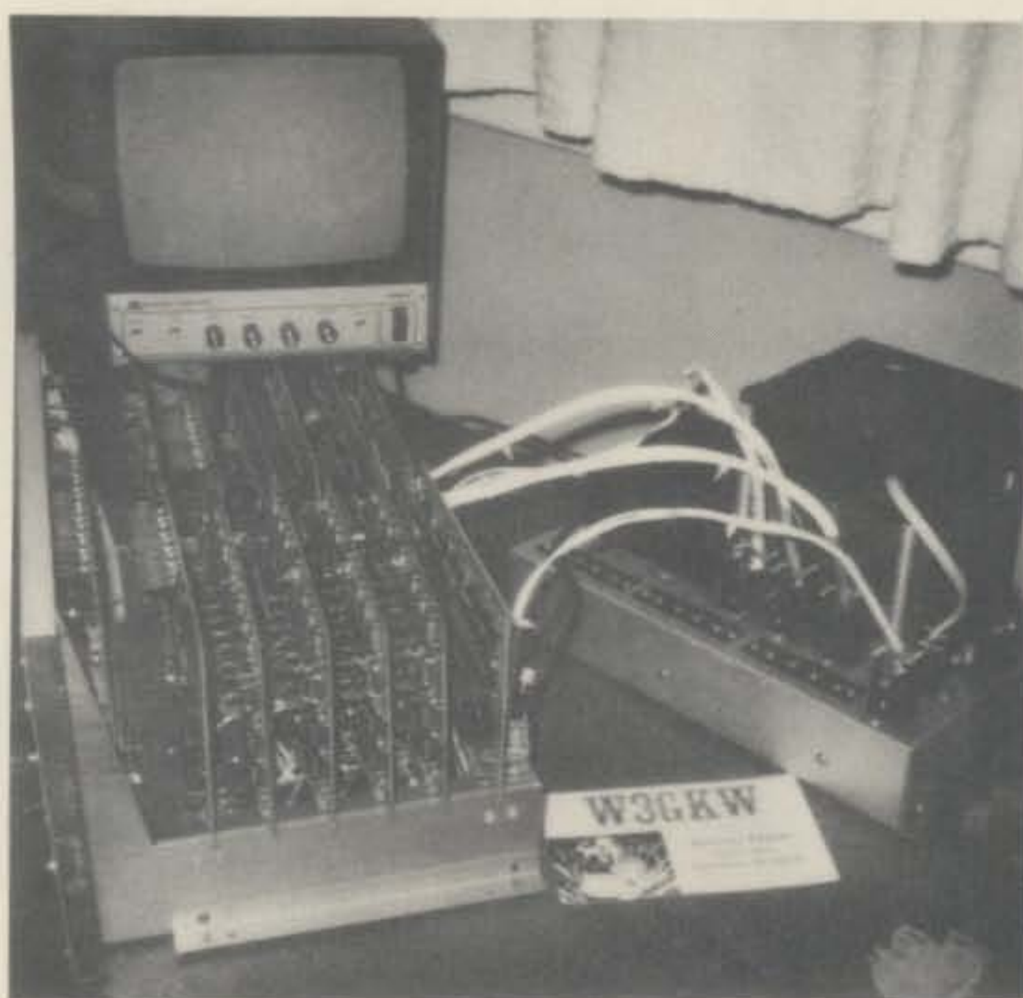
W3GKW chose to separate "the works" and the power supplies, as seen in this "exposed plumbing" view.
