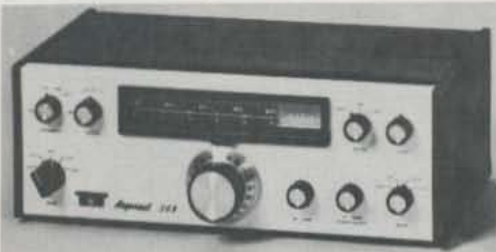
Argonaut 509. 3.5 to 30 MHz, 5 watt s.s.b./c.w. transceiver. Solid state, permability tuned, instant band change, built-in s.w.r. bridge, S-meter, and internal speaker. WWV, direct frequency readout, and receiver offset tuning. $329.00 Ten-Tec , Sevierville, Tennessee, 37862.
