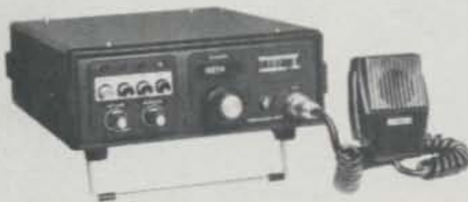
Yaesu 200R. 200 channel synthesized f.m. transceiver. 144-146 MHz or 146-148 MHz. Power output 1 or 10 watts. Built-in tone burst oscillator. Priority channel. Automatic VSWR protection. Selectable \pm 600 kHz transmitter offset. $449.00. At dealers.
