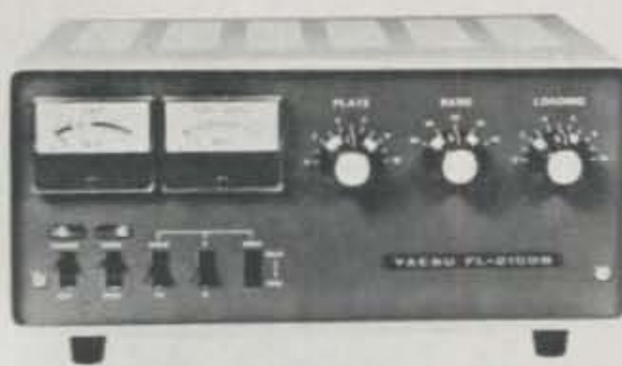
Yaesu FL2100B. 80 to 10-meter linear amplifier. Conservative 1200 watts p.e.p. input on all bands. 117 to 234 v.a.c. operation. Built-in s.w.r. meter. Tubes biased to cutoff during receive to maximize tube life and minimize heat. Individual input coils for each band. $399.00. At dealers.
