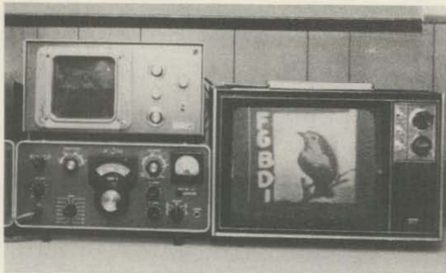
Fig. 4—Test picture received by W2DD from F6BDJ displayed on a 14 inch monitor via scan conversion.
