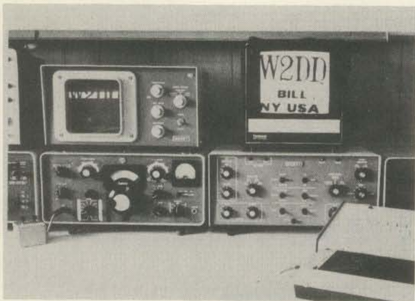
Fig. 2—A station identification picture is shown here as displayed on both SLOW and FAST scan monitors. At the left, the bright sweep of the CRT beam proceeds down the screen. At the right, the complete station "ID" is seen displayed on a Panasonic monitor after scan conversion by the Robot Model 300 Storage Tube Scan Converter.
