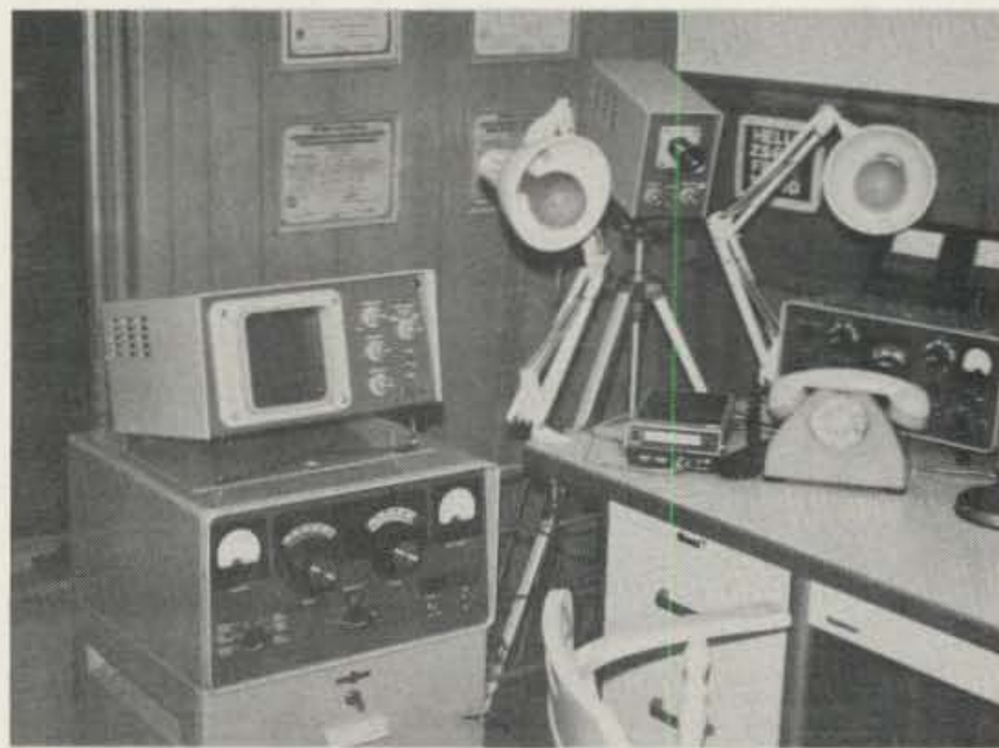
Fig. 1—All the makings for SSTV fun. At the left, a Robot Research Model 70 Monitor for viewing SSTV pictures on a long-persistence radar-like screen. Between the white lamps is a Robot Model 80 camera set up to transmit a picture of the operator. A Sony tape recorder is used to record SSTV "video" as described in the text.
