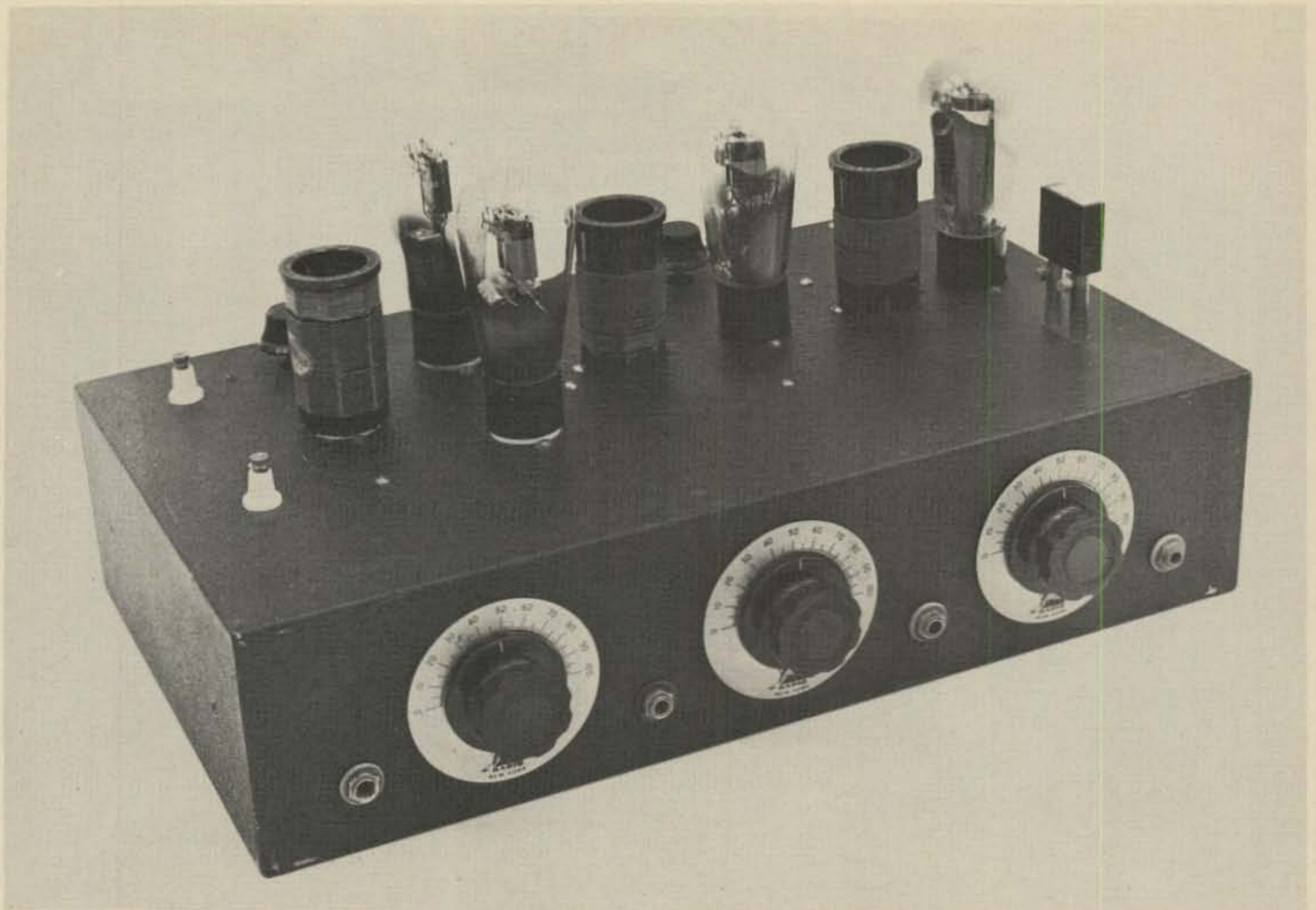
Fig. 1—The Gross CW-25 transmitter. Sold as a kit for $13.95, this simple 50 watt transmitter was used by many beginners and Old Timers alike during the 1933-1934 years of the Great Depression. The transmitter used a 247 crystal oscillator, a 46 buffer or doubler and two 46s in the final amplifier stage. With a 500 volt supply the transmitter ran 50 watts input and delivered about half that power on 160, 80 or 40 meters. On 20 meters, output was down to about 15 watts. One set of plug-in coils came with the transmitter kit, other coils and the crystal were extra. No meters were provided but four panel jacks allowed the operator to measure plate and grid currents. The jacks were insulated from the chassis as they were "hot". Considered very dangerous today, the "hot" meter jack was just one of the hazards of the game in 1934! Antenna connections were left to the ingenuity of the owner, as only a link-coupled winding was supplied for the output circuit. Most amateurs either keyed the B-plus of the buffer stage, or else placed the key in the grid meter jack, J3 of the amplifier to achieve blocked-grid keying.
