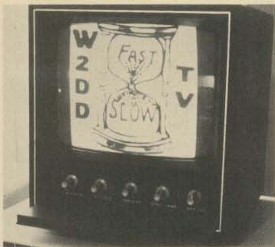
A typical fast scan monitor. This 9 inch diagonal Panasonic Model TR920M is an excellent size for viewing scan converted SSTV.
