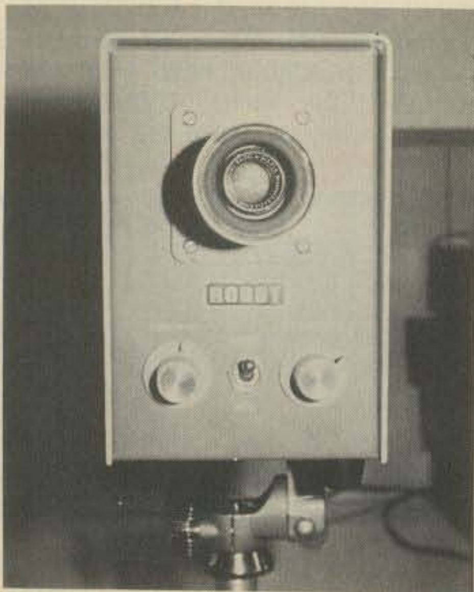
Front view of a Robot Research Model 80 camera showing the brightness and contrast controls.
