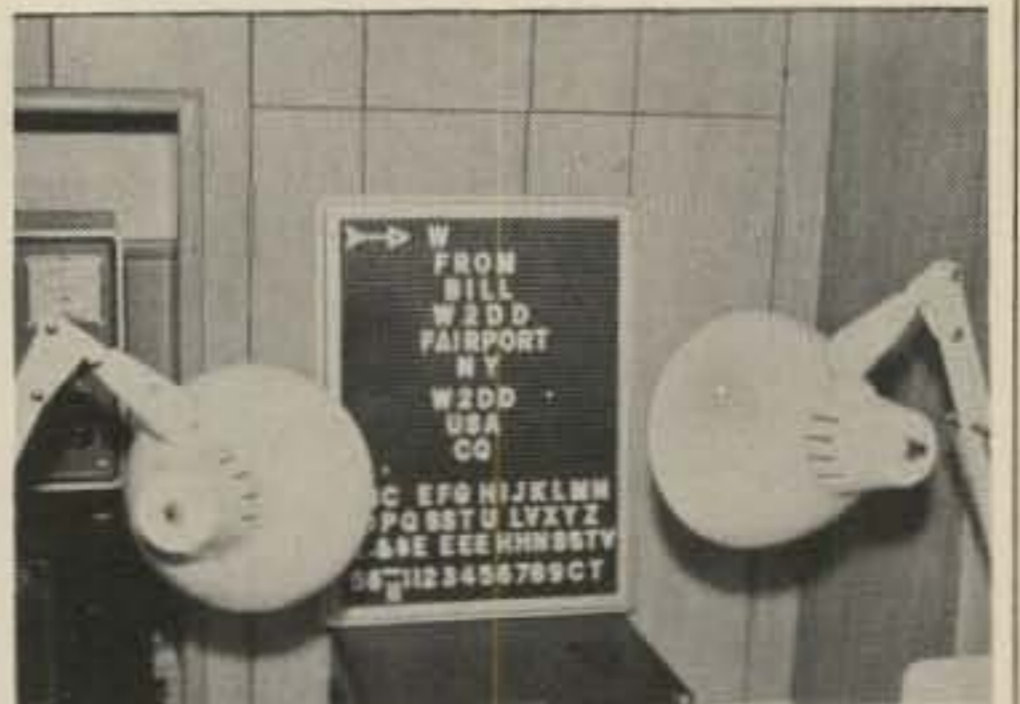
A Typical "menu board" set up for alpha-numeric SSTV transmissions. The onerous task of forming words etc. with hand set letters is completely out of phase with television communications! NOT RECOMMENDED, PERIOD!
