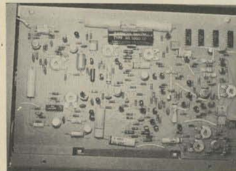
A single circuit board carries virtually all electronic parts of the Model 80 camera.
