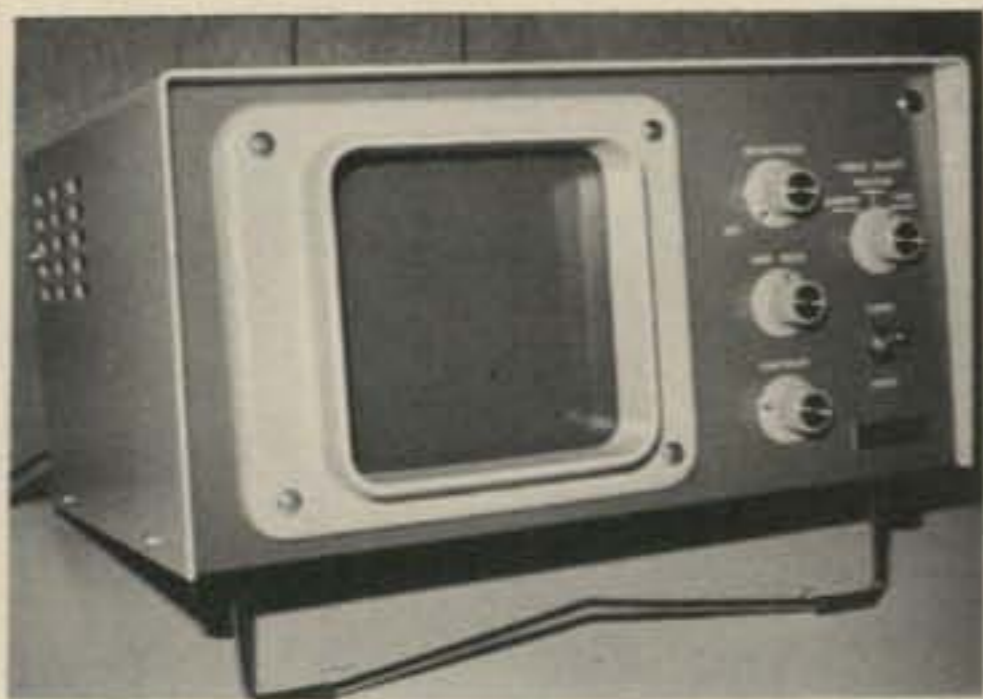
The Robot Model 70 monitor. Without a doubt the most popular and widely used P-7 monitor ever made.
