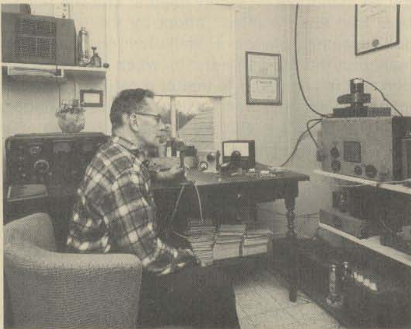
This is the 75-meter a.m. station W3CIC in Edgewater, Maryland, and the operator Lawrence A. Laser. The final is a pair of 813's in push-pull modulated by a pair of Class B 805's. The receiver is an SX-28.
