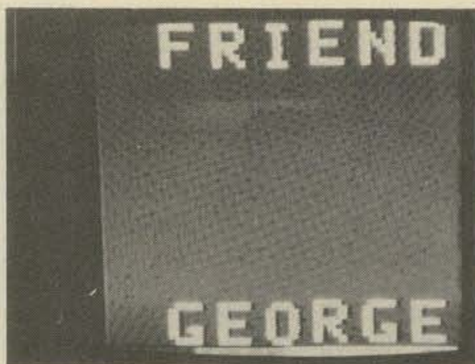
Fig. 10—Use Lines 1 and 5 of your SSTV Keyboard to get this effect. Blank out Lines 2, 3, and 4 with the space bar.
