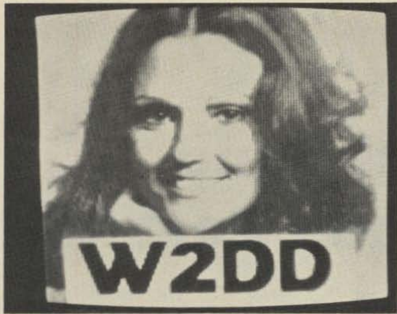
Fig. 9—A tape recorded "portrait type" picture can be used to set up a monitor when no gray scale tape is available. This photo illustrates the effect of too much brightness and too low contrast. Highlights in the flesh tones lack detail and shadow areas in the hair are not very dark.
