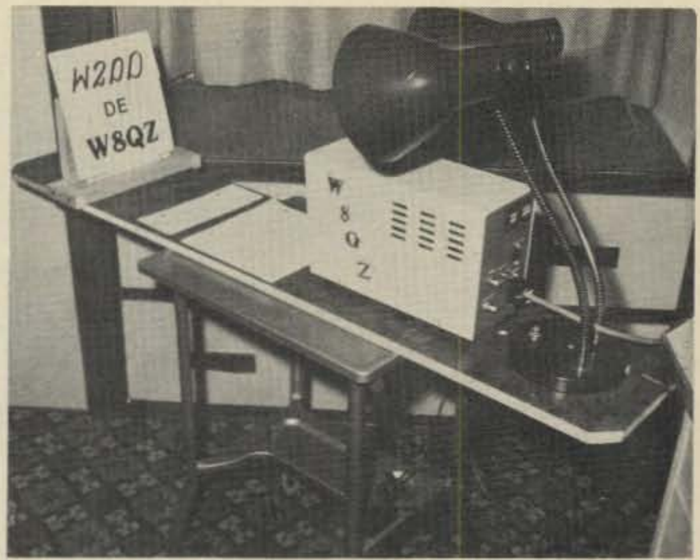
Fig. 3—Pearl "PT" Taylor, W8QZ, uses this simple but effective easel board to televise "flat copy". Note how an inexpensive dual lamp is used to flood the subject with light.
