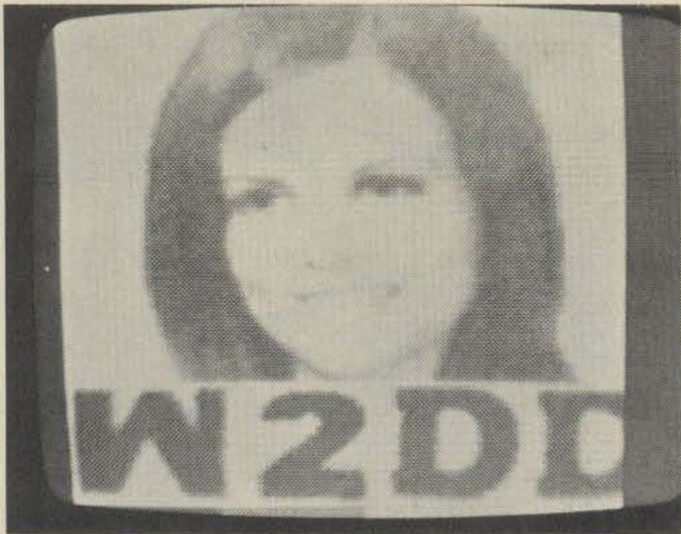
Fig. 5—Appearance of SSTV picture caused by incorrect tuning. Here, the pitch of the received signal is too high with resulting loss of blacks and a washed-out look.
