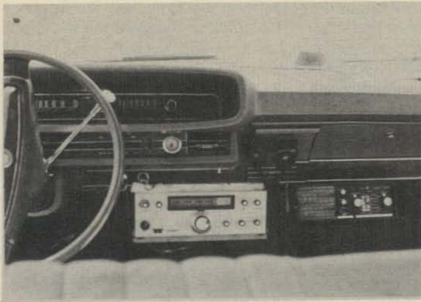
Mobile installation of the Argonaut in OA8V's '69 Ford. It was used during cross-country trip during his 1974 furlough in the U.S.
