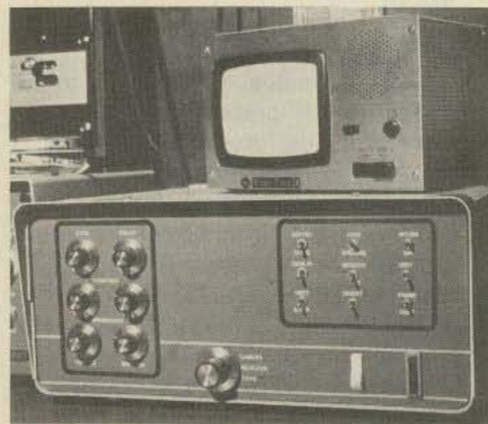
Fig. 3—Front view of W1VRK's version of the WB9LVI scan converter. A very professional looking job. Note the mini-Monitor by Video-Guard on top of the converter.
