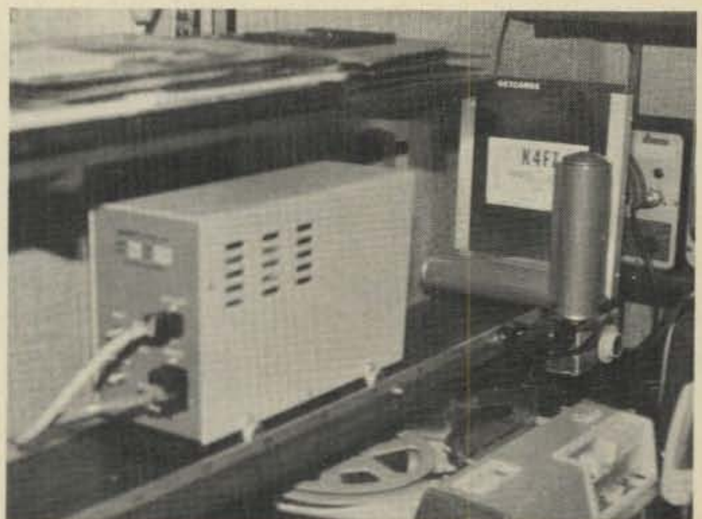
Fig. 4—Bob Weinig, K4FZ, built a track to guide his Robot 80A camera back and forth as necessary for each subject. Note the vertically oriented lamps used by K4FZ to get balanced lighting.
