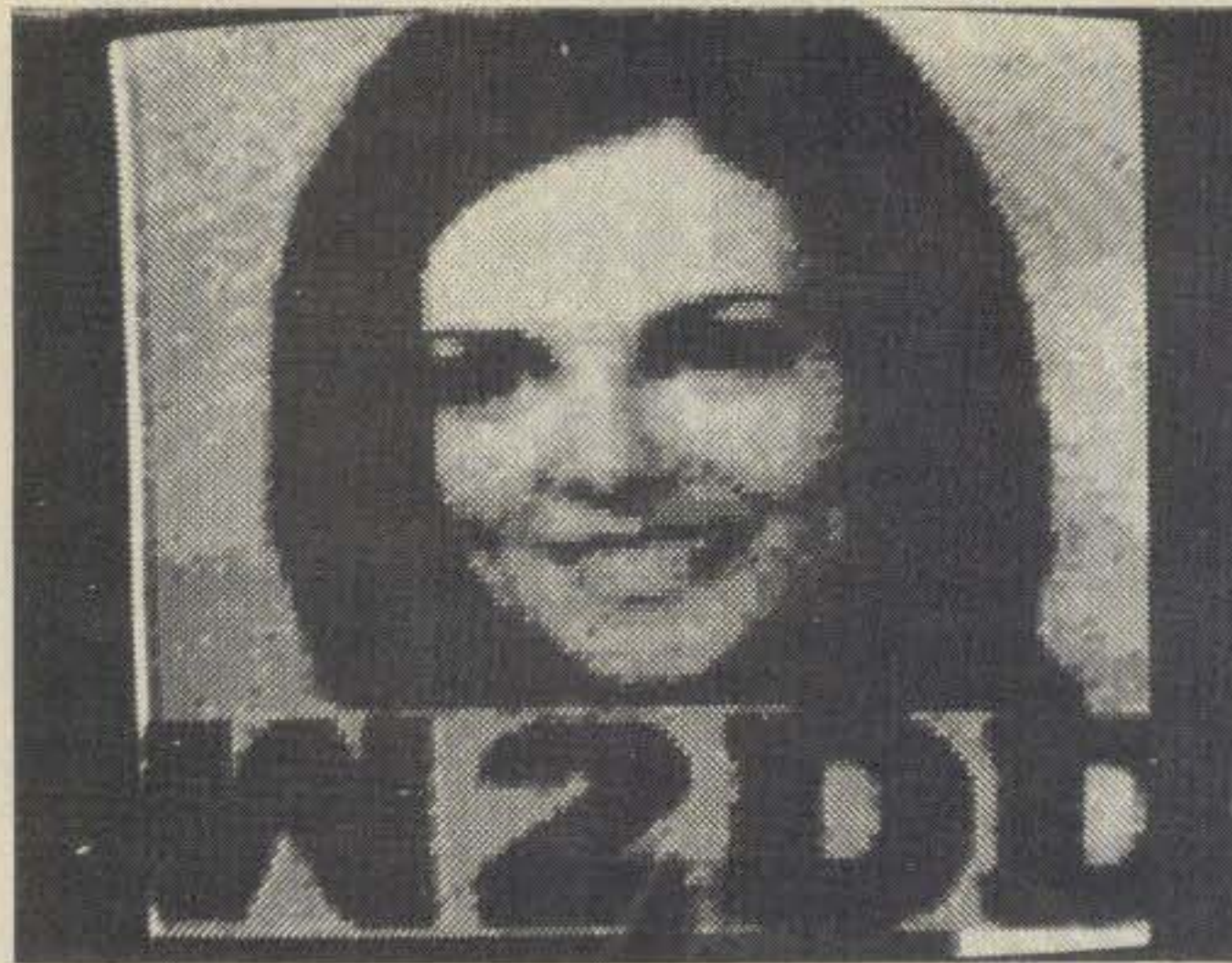
Fig. 7—Appearance of SSTV picture resulting from too low pitched signal. Lack of frequencies above about 1700 Hz. causes loss of whites in picture.
