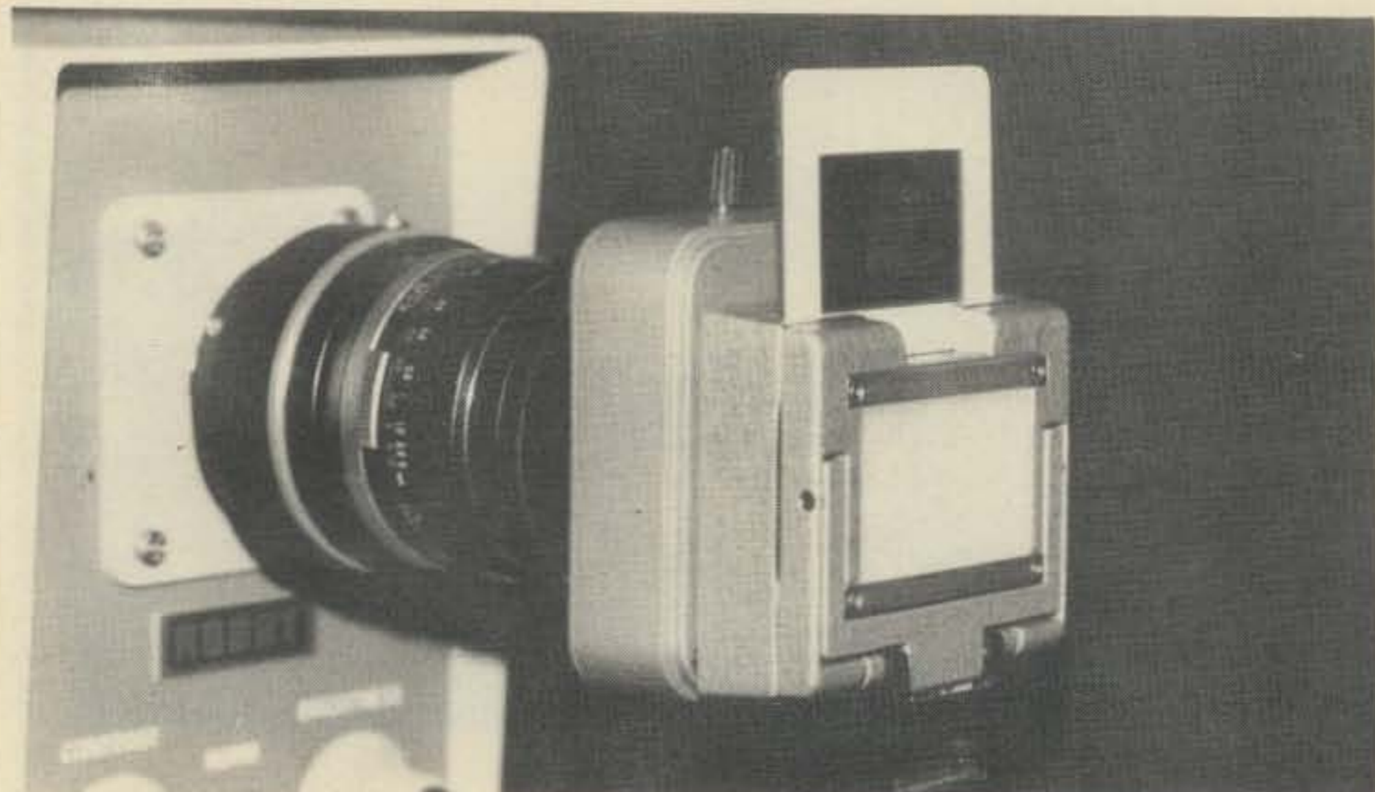
Fig. 8—With the slide duplicator device screwed into the SSTV camera lens, all you need is some backlighting.
