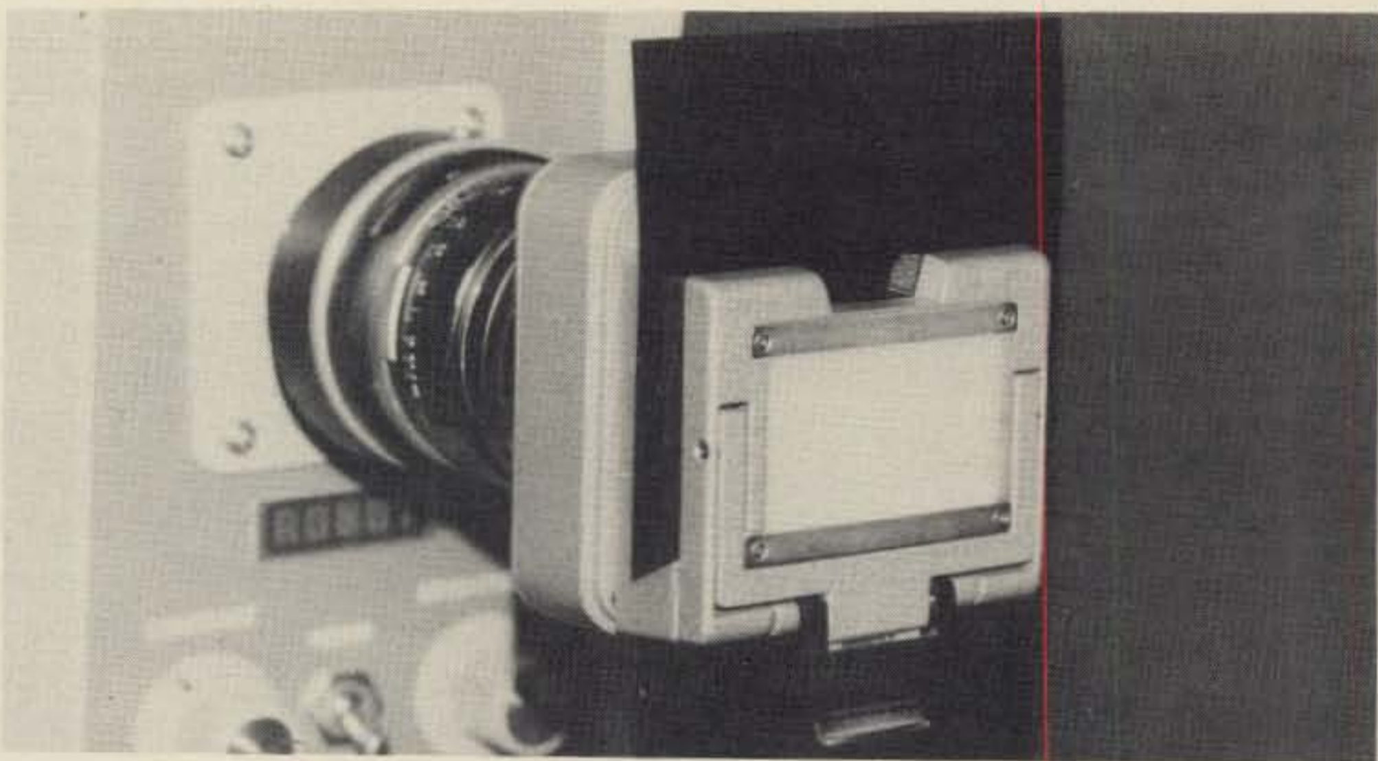
Fig. 11—When F6BDJ transmits color SSTV he uses this simple means of applying the various filters.
