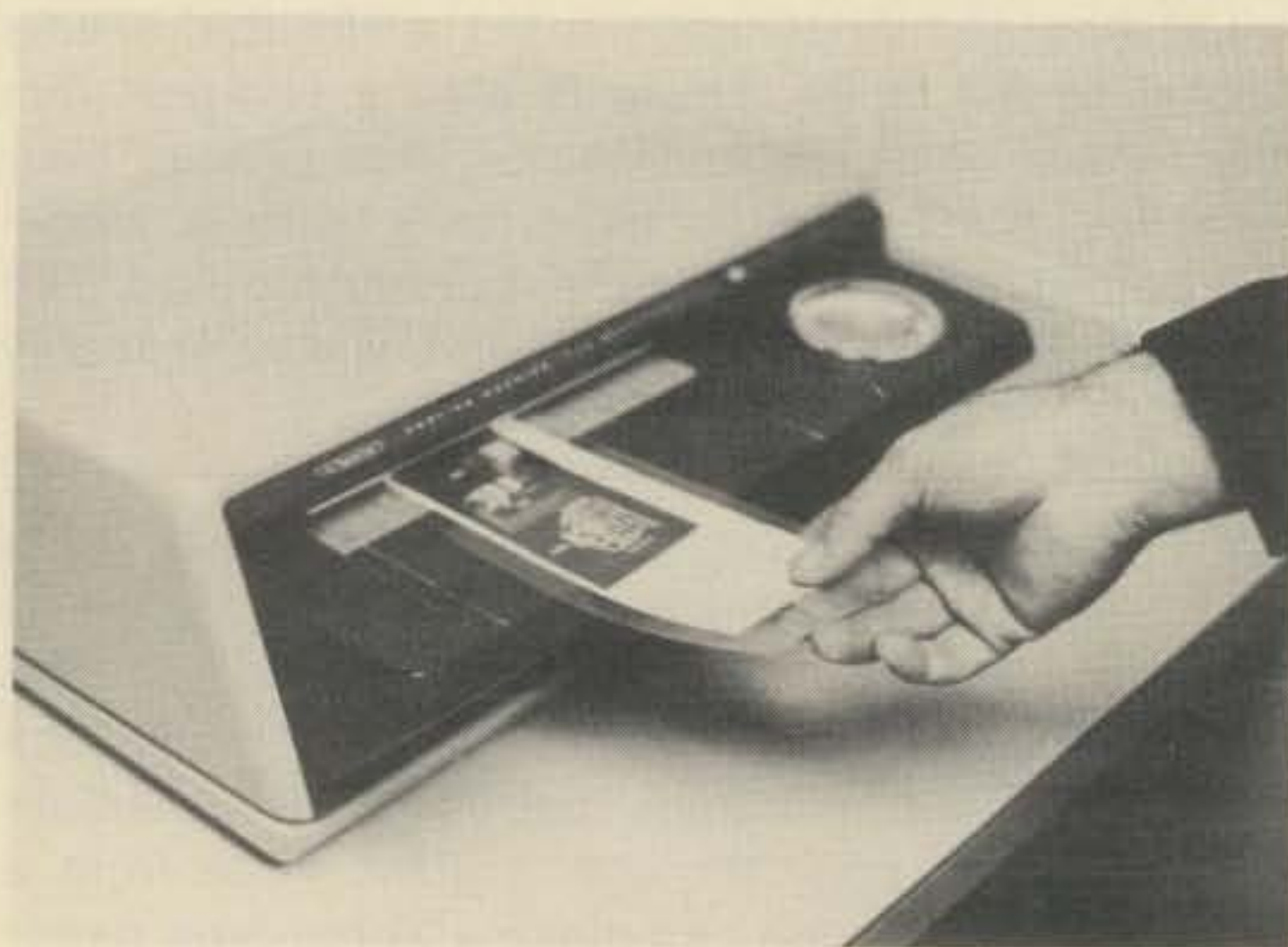
Feeding a circuit board layout cut from a magazine page and a piece of film (about 1/3 sheet to save material) through the "secretary" machine.
