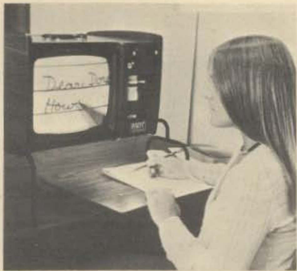
Fig. 2—Visualtek's Miniviewer with 12" screen. "Folded" optics permit viewing flat copy placed on an easel at magnifications up to 40 times. Other features are: easy-to-operate brightness and contrast controls, portability, and image polarity selection.
