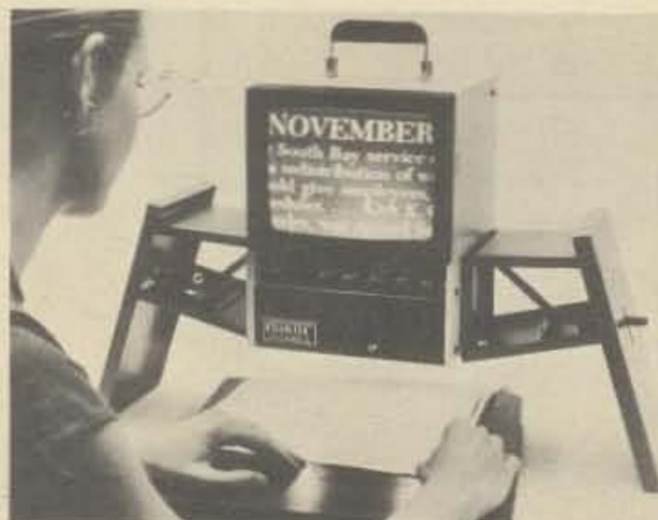
Fig. 3—Featuring a 9" screen, the Visualtek "Commuter" has fold up legs, weighs 21 pounds. Its magnification is limited to 8 times original size.
