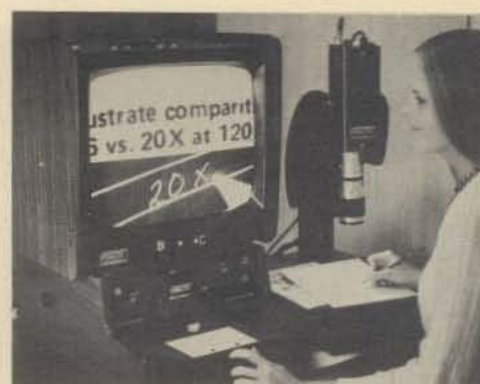
Fig. 4—"Big Daddy" of the Visualtek line is the RS-6 system in which the camera and monitor are separated. Magnification can go to 60 times original size! The camera/lens combination of the RS-6 would be the answer to a Slow Scanner's dream!
