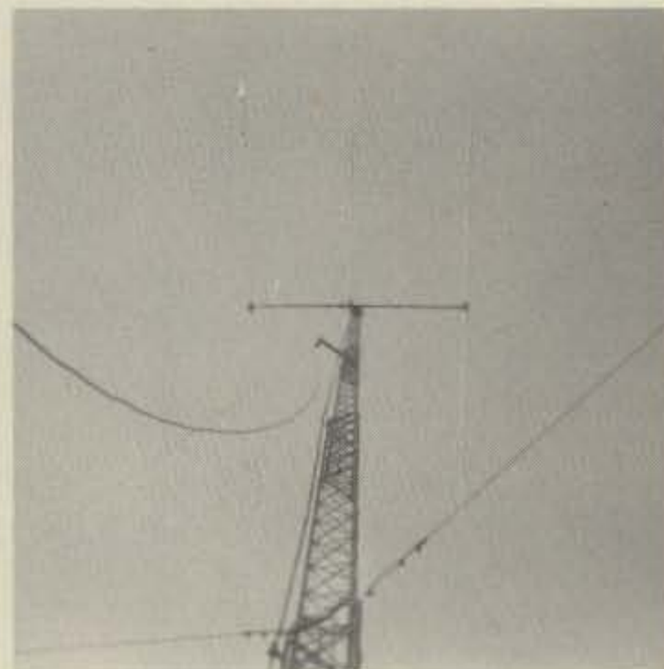
A shot of W6PQZ's TH3 Jr. at 70 ft. A 40m inverted Vee is supported part-way up the tower.
