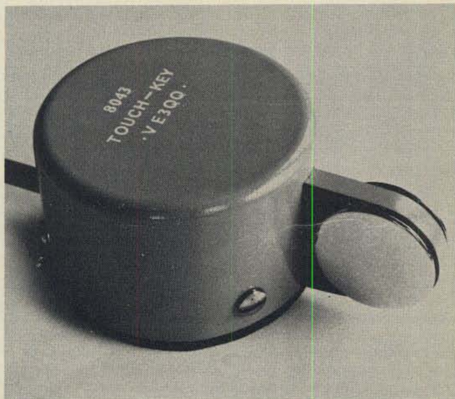
Here is the touch-control in the operating position. The cover is a paint-can top, and the unit works equally well with the 8044 chip.
