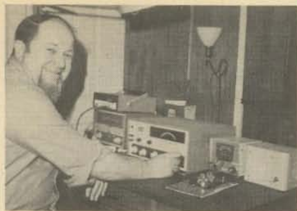
Bill Burns, Novice, WB9TDV, Reedsburg, Wisconsin, uses a Heath-Schlumberger frequency counter to keep his signals in the Novice bands! His Heathkit HW-16 transceiver and HG-16 variable frequency oscillator have teamed up with separate 80- and 40-meter dipoles for 27 states, confirmed. A Heathkit R.F. wattmeter completes his equipment. We are sending WB9TDV a one-year subscription to CQ for sending this winning photo in our Monthly Photo Contest.
