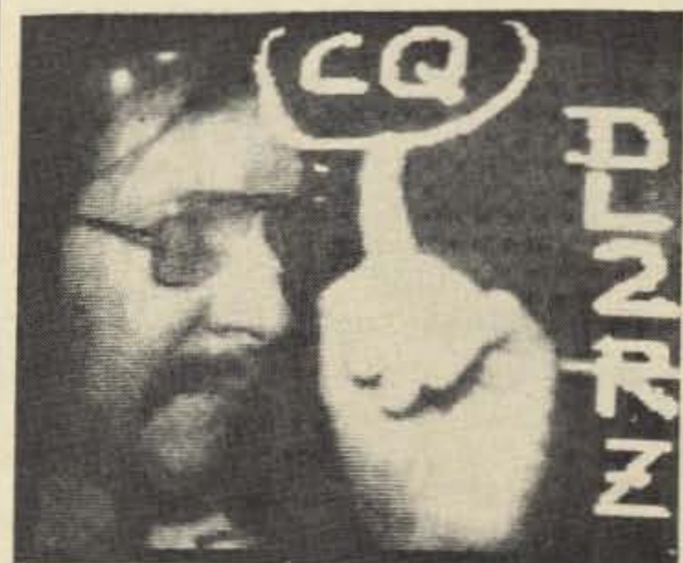
Fig. 11—Now you can put the frosting on the cake! An "electronic pencil" or "light pen" offered for sale with the SC-420 will permit you to "write on the screen" as demonstrated here. The writing can be either black or white. (This device works only with its parent equipment.)
