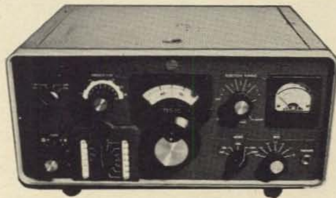
75S-3C RECEIVER $2504.00 Sharp selectivity. SSB, CW and RTTY. Single control rejection tuning. Variable BFO. Optional mechanical filters for CW, RTTY and AM. 2.1 KHz mechanical filter. Zener regulated oscillators. 3-position AGC.
