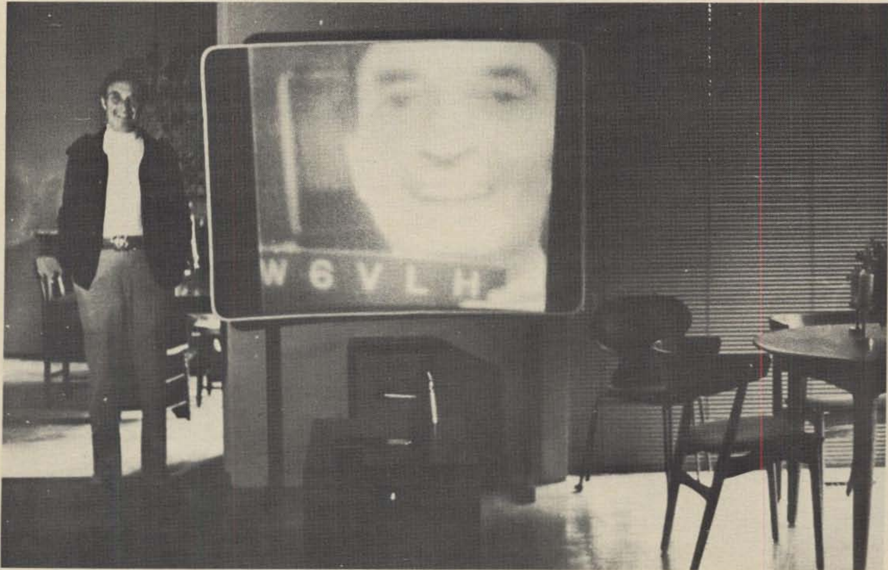
Fig. 2—At close range Mel is further dwarfed by his own image. As mentioned in the text, the three gun projection system seems to minimize the appearance of TV lines. Photo by Ms. Joiner.
