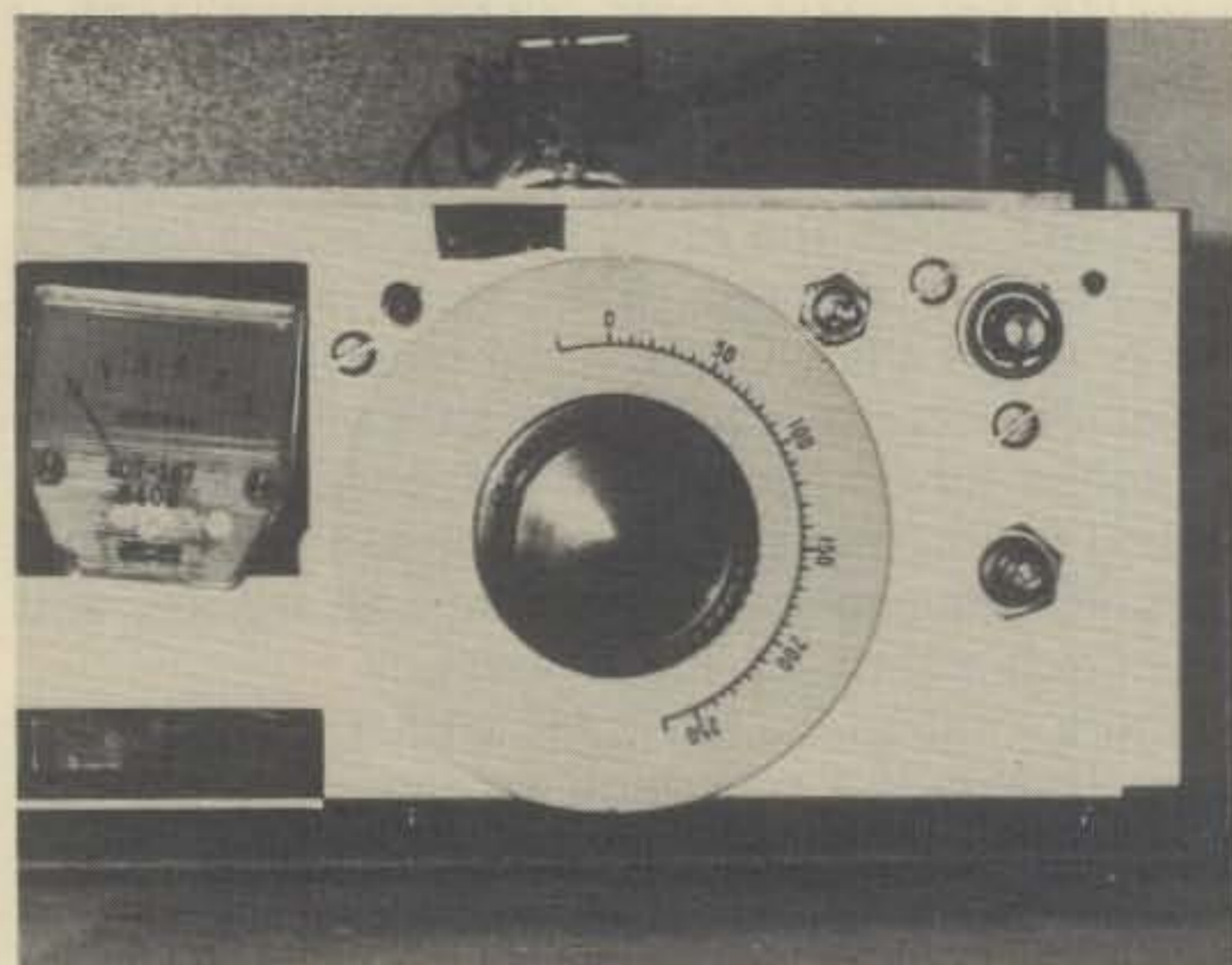
Position of R5 RIT tuning pot to provide about 1/2 inch clearance between nut and dial plate.
