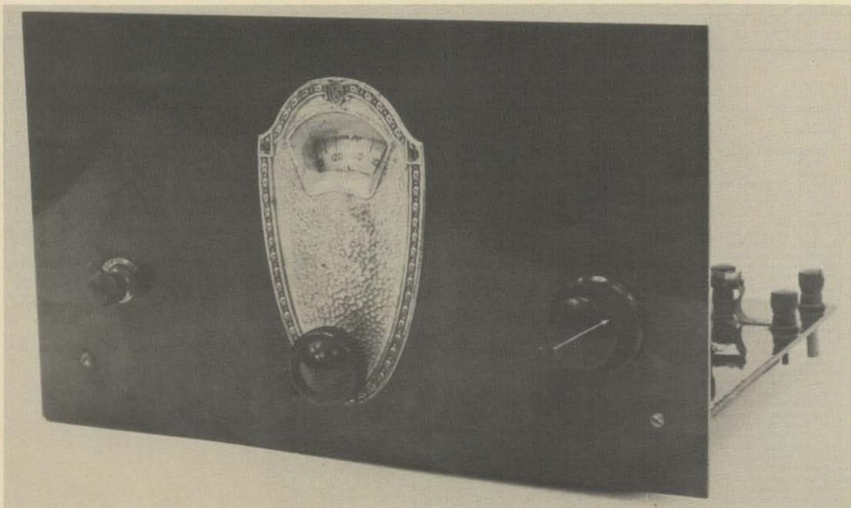
Fig. 1—The two tube National SW-2 receiver, the "Godfather" of the famous SW-3. This simple regenerative receiver was primarily designed for high frequency television reception which enjoyed a vogue in the 1928-1930 era. The receiver was battery operated and had an untuned r.f. stage followed by a regenerative detector. To the left of the main dial is the filament switch and to the right is the regeneration control.
