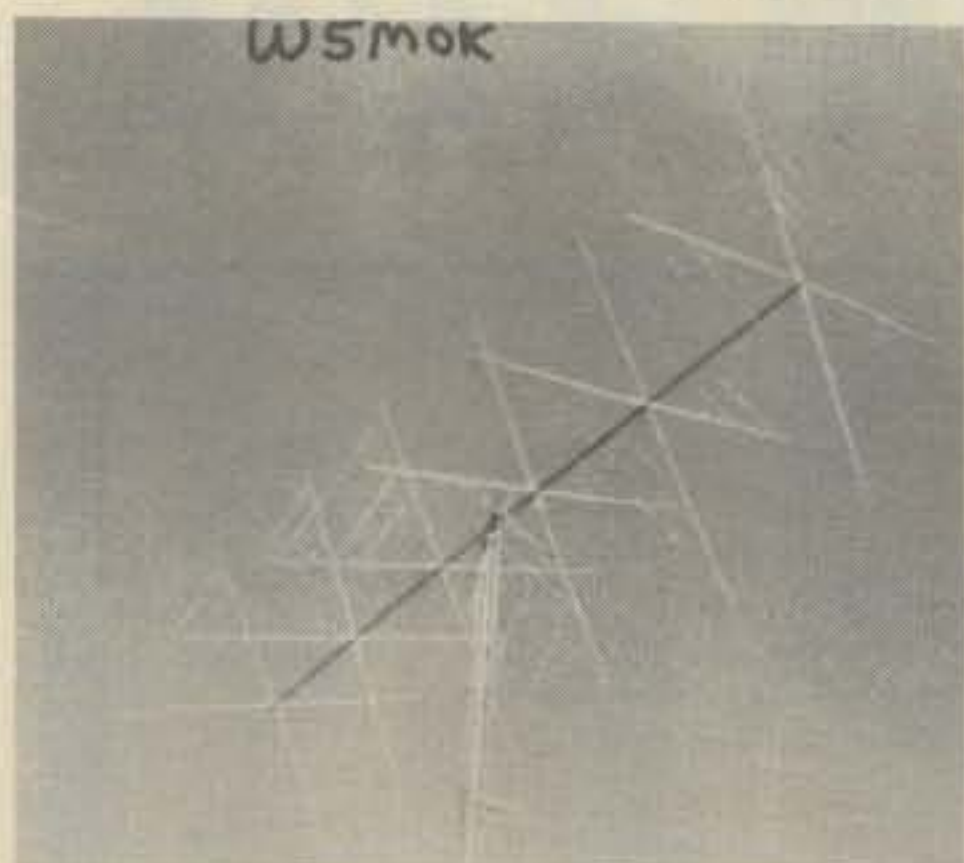
Fig. 2—The six element Quad of W5MOK is mounted on a 50 foot boom. The boom is mounted in a sleeve that permits the antenna to rotate along its axis for ease of maintenance and tuning. Antennas are fed with separate coaxial lines.
