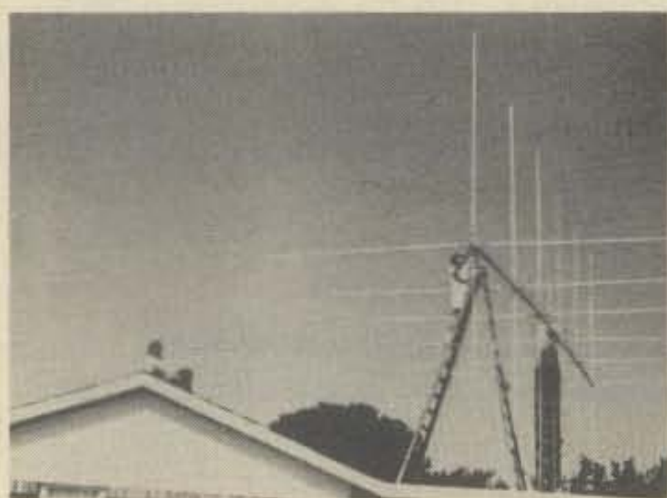
Fig. 1—The six element, three-band Quad of W5VGE. A 52 foot boom is used and the array is mounted on a 72 foot, heavy-duty crank-up tower. WB5NJK at left supervises antenna adjustments, which are made from the top of a step ladder on the roof.
