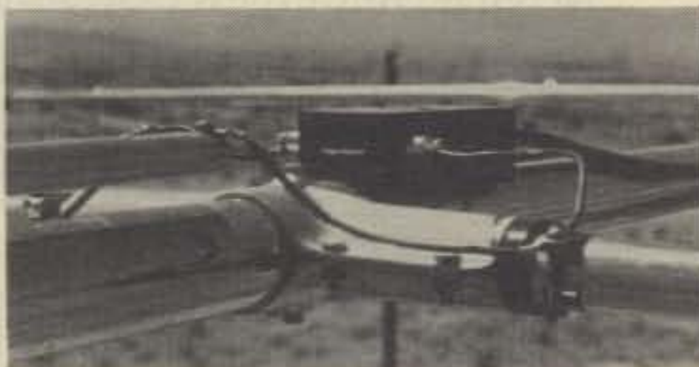
INSULATED DRIVEN ELEMENT WITH PRECISION BETA MATCH AND HEAVY DUTY ELEMENT MOUNTS
