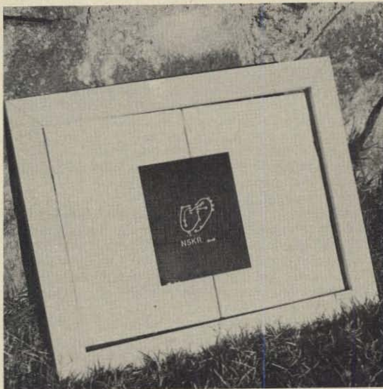
Fig. 4—Front view of the N5KR contact printer, exposing a small circuit board by solar power!
