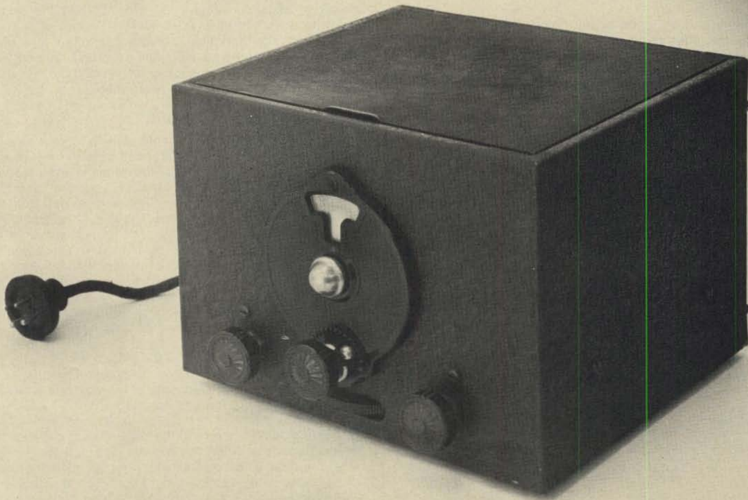
Fig. 1—The popular SW-3 receiver by National Co. This three tube, pre-war beauty is today's hot collector's item. Using plug-in coils, the SW-3 covered all frequencies between 30 MHz and 90 kHz. Panel controls (left to right) are: R-f trim, tuning and regeneration. Below the main tuning dial is the horizontally mounted r-f gain control, calibrated in signal strength units. Receiver required external power supply.
