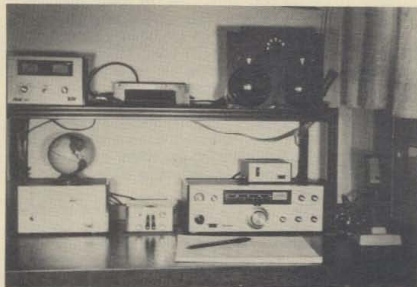
The match box is shown as an integral part of this fine QRPp station. The large knobs on the match box help to make fine adjustments.
