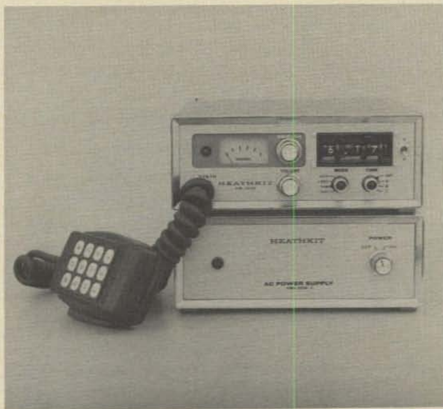
Front view of the HW-2036 as it looks sitting on the HW-2036-3 a.c. supply.
