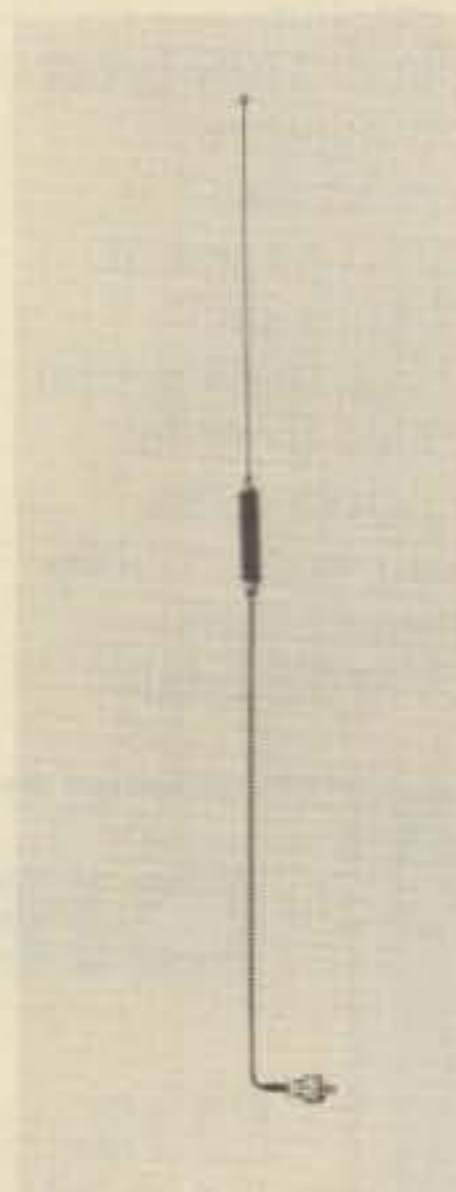
This "back-of-set" indoor CB antenna can be adapted for 2-meter operation in a few minutes simply by unscrewing the loading coil and top section. A 9½" section of stiff wire or bus bar is clipped to the top by an alligator or crocodile clip to make the antenna a resonant quarter-wavelength. (Photo courtesy Radio Shack)
