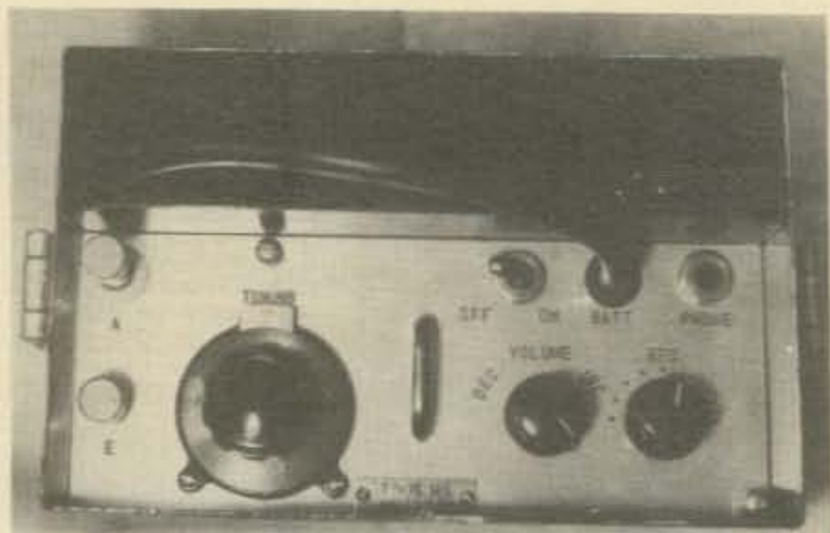
The front panel of the RSK-253 receiver. Note that the frequency tuning dial is scaled from 1-100. See fig. 2 for dial indication to frequency conversion.
