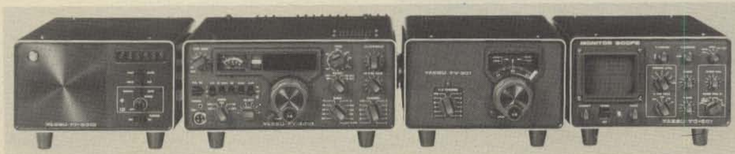
Left to right: FP-301D power supply, FT-301D transceiver, FV-301 v.f.o., YO-301 monitor scope.
