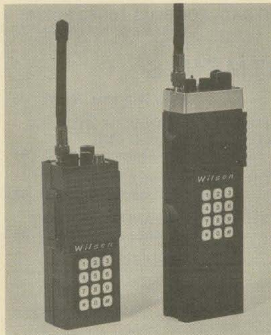
FOR SIZE COMPARISON, THE NEW MARK IV IS ILLUSTRATED NEXT TO WILSON'S 1405SM SWITCHABLE 1 & 5 WATT RADIO.
