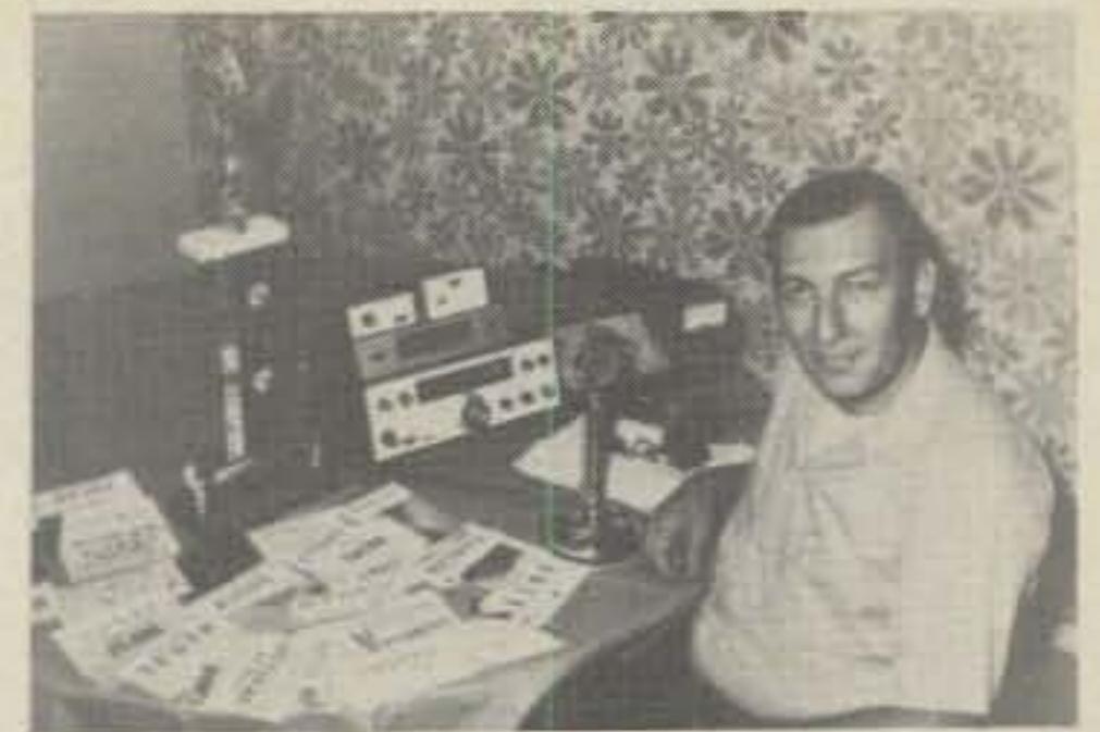
W8ILC at the operating position. The Argo 509, factory-converted for 1 watt input, is topped by a digital readout, and power supply and audio filter. DXCC MILLIWATT #1 stands to the left of the Argo, and some of Ron's exotic cards are spread on the table—such things as VK4, TF5, FO8, CE0, 7KI, VS7, TU2, HV3, and FO0 are visible.
