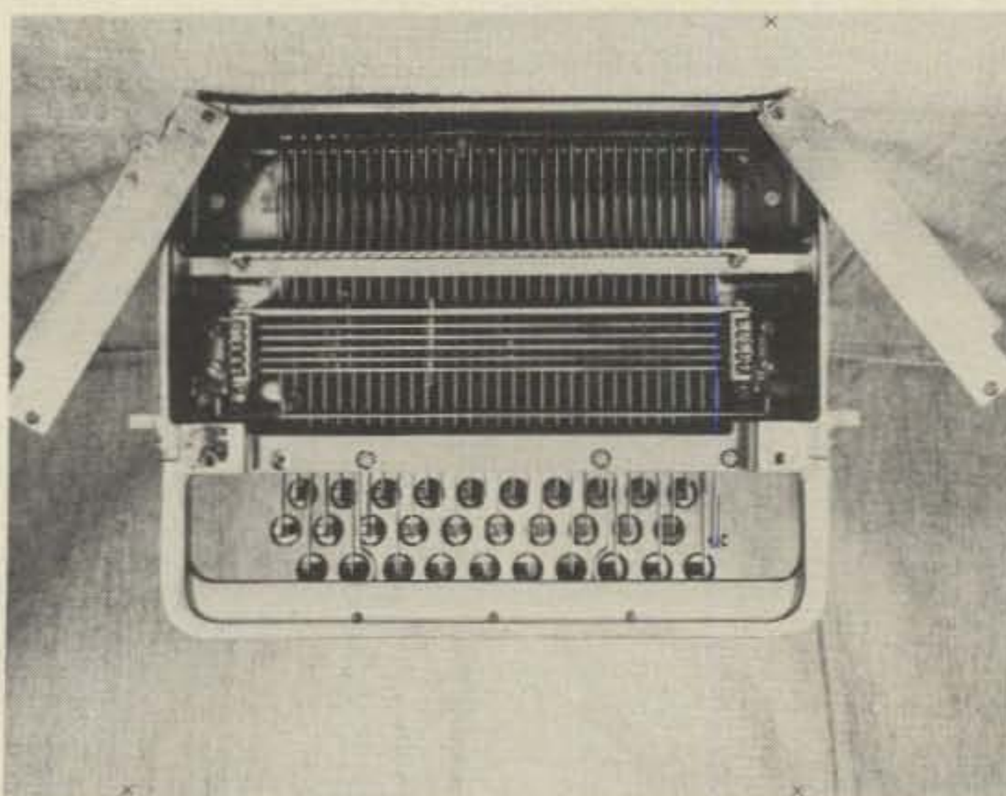
Fig. 6 - The underside of a (typical) keyboard. The five crossbars are seen perpendicular to the key levers.
