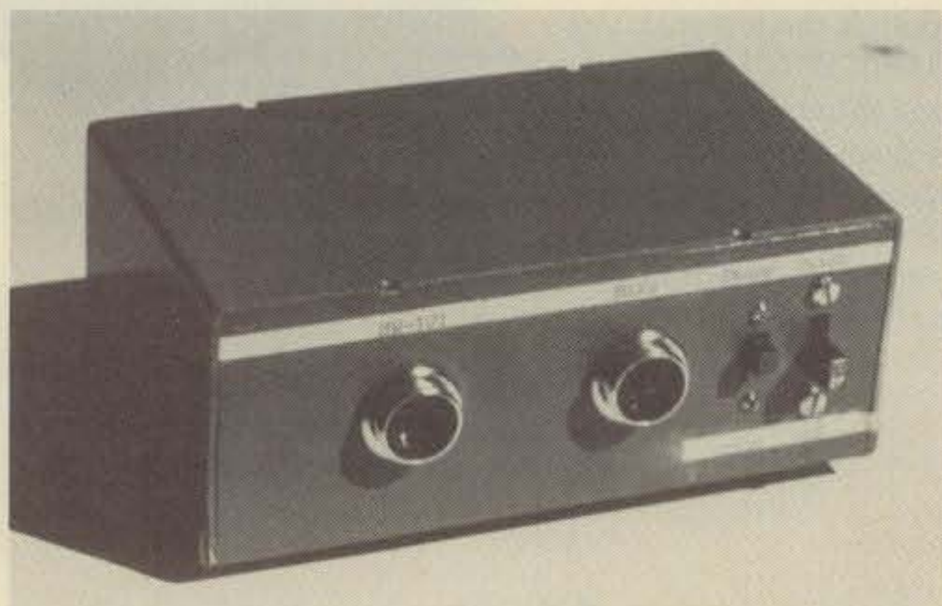
A simple patch for p.t.t. operation uses an original high-quality transformer.
