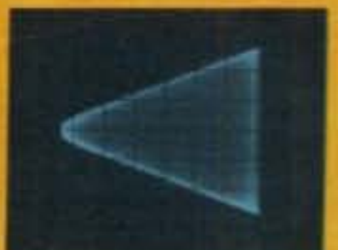
Wave Envelope shows full SSB voice modulation, with processor on (full compression), and "clean signal" at full power.
