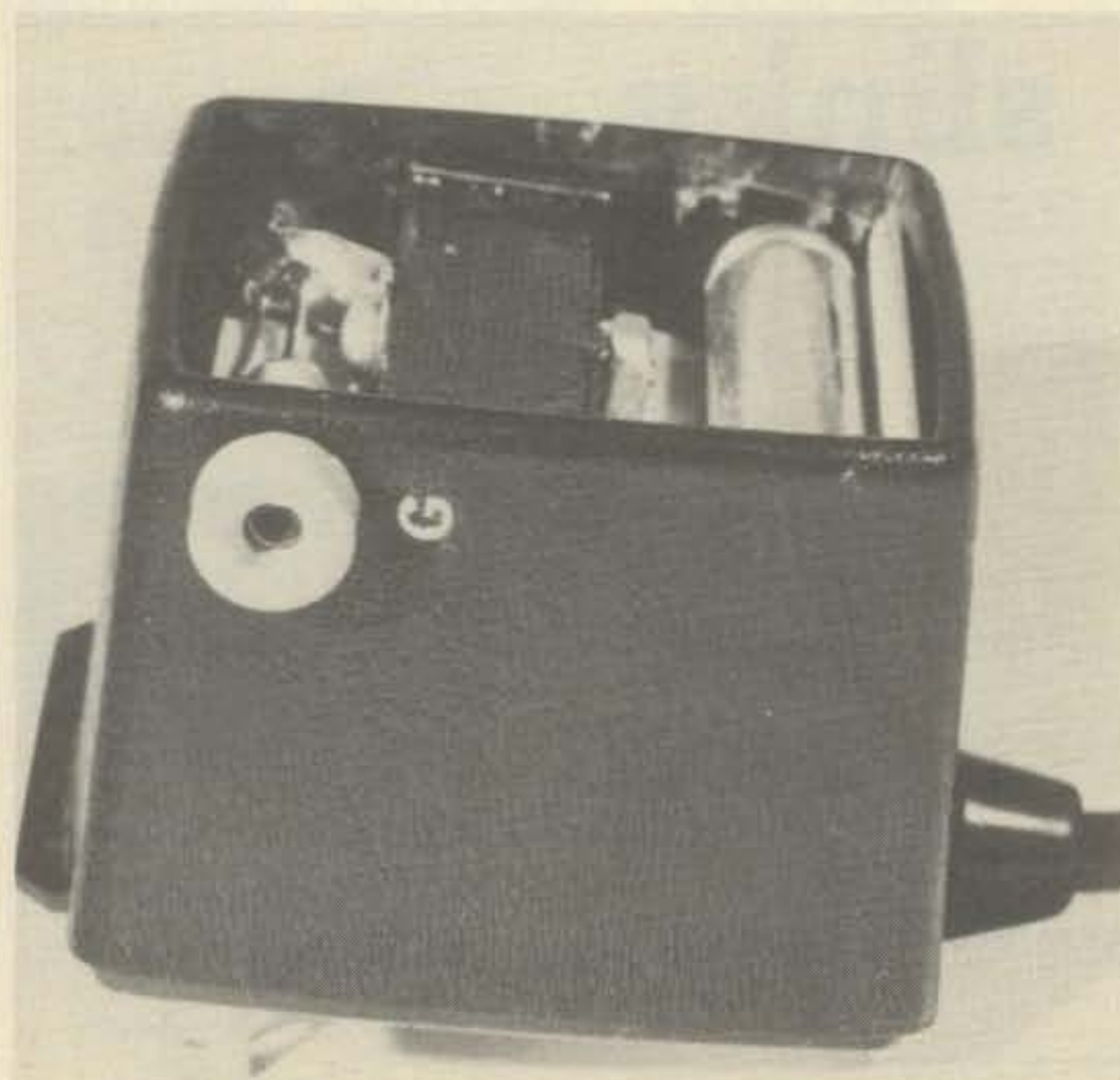
This shows the a.c. line r.f. filter and connections.
