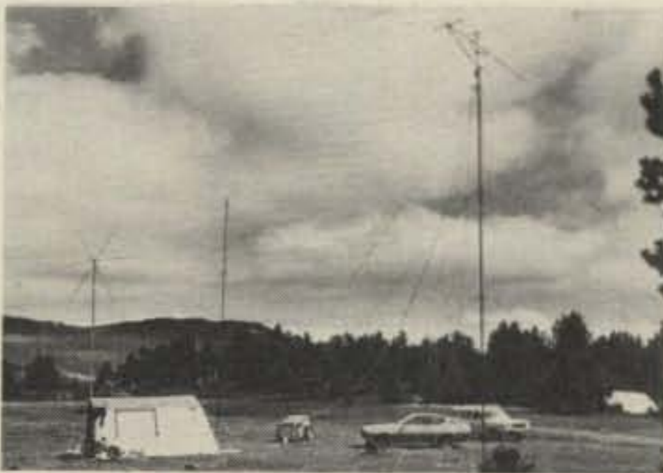
Site of the C31 DXpedition, 6,600 ft. a.s.l. Left the quad, in centre the mast for the dipoles, and the mast with the 10 meter dipole plus 10 elements on 144 mHz at right.
