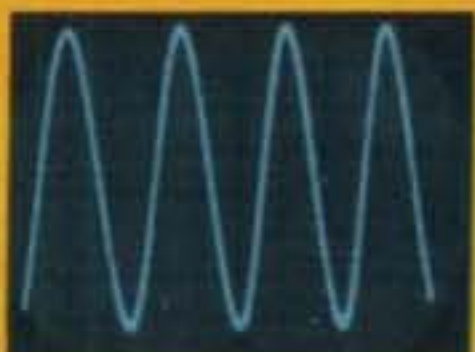
Oscilloscope Operation (1 kHz) Oscillator function allows Sine, square wave, Lissajous patterns for testing or design work.
