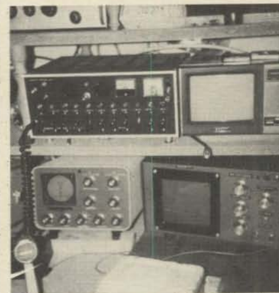
Fig. 2 - At the lower right is VK3LM's homebuilt EXACT copy of a Robot 70 monitor. At the upper left is a homebrewed control unit described in the text.
