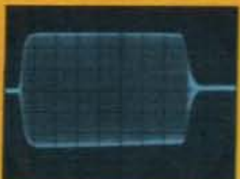
Keyed Waveform Shows detail of CW keying. Use to monitor the quality of your CW note. (Photo shows ideal waveform produced by TS-820S.)
