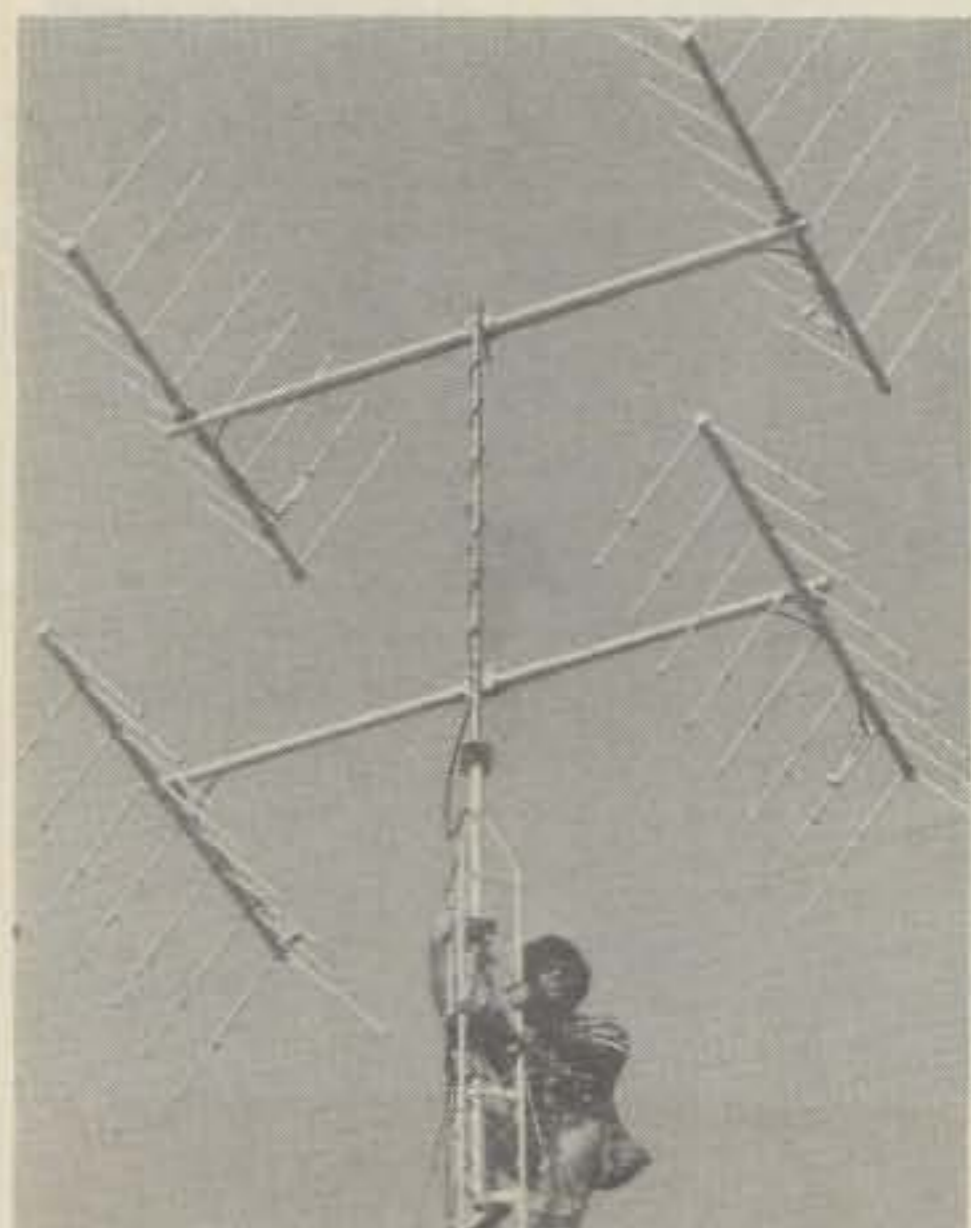
Fig. 8 - A four-bay Delta Quad built by WB0TEQ and W0MBP. Terry, WB0TEQ atop the tower. A total of 32 elements in this array.
