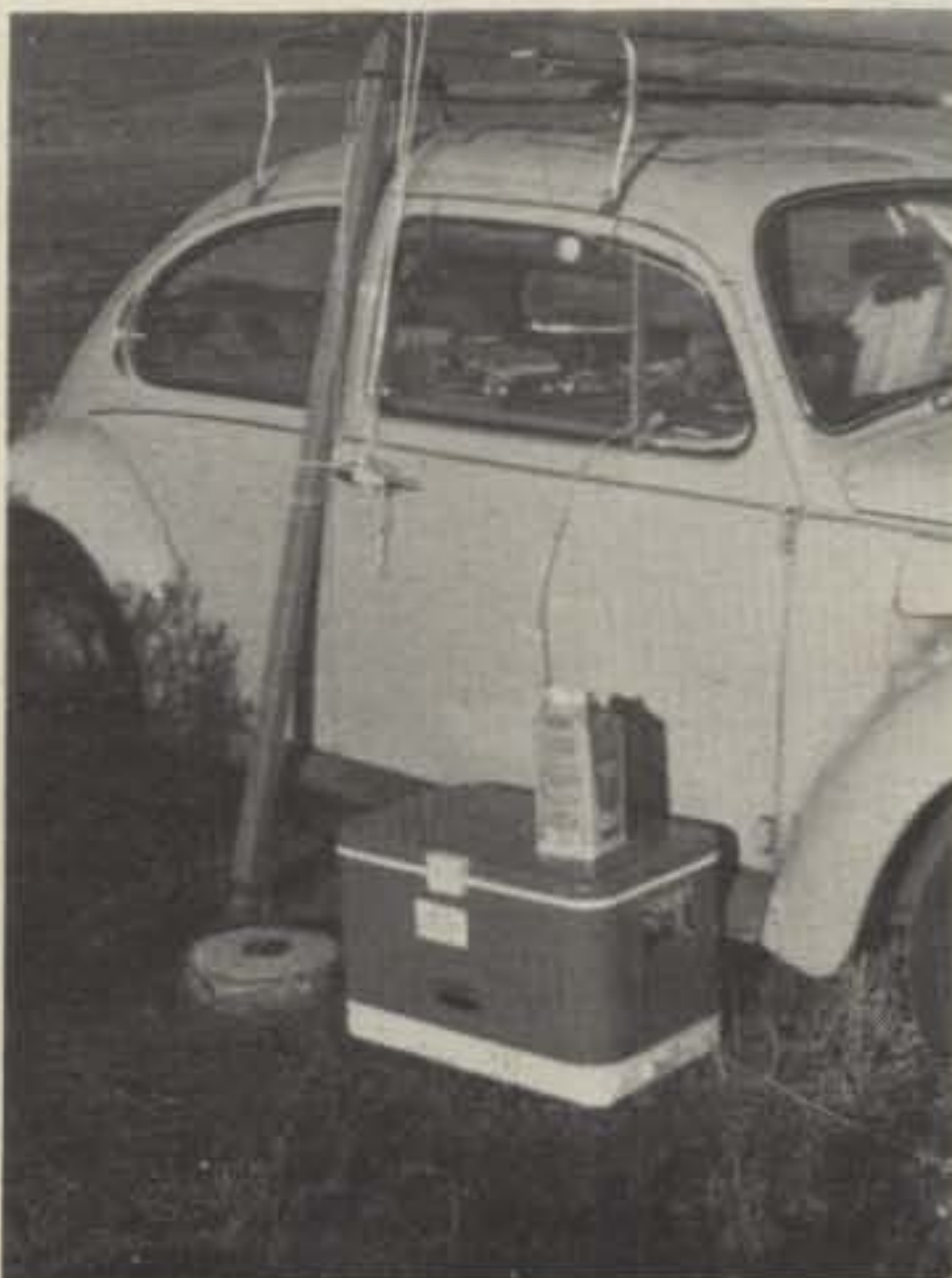
Looking southwest at the foothills of the Sierra Nevada Range in Calif. The border marker is between the base of the pole and the food chest. The car is in California. The cable coming out of the little window goes to a storage battery under the rear fender. The antenna is end fed and the car body is the ground system. All sleeping was done on the back seat.
