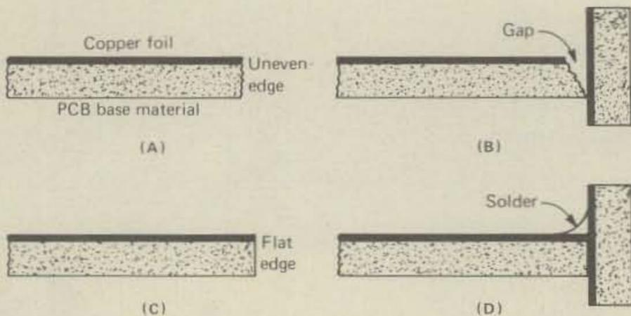
Fig. 1 - Joining printed circuit board stock. See text for a complete description of how this is done.
