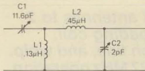
Fig. 2 - Target values of the network. The  $C_1$  shown was an obsolete JFD type VCJ2555 1-40 pF capacitor which may be replaced here with JFD NMC623TT (about \$10.55). A 3-30 pF mica trimmer or air capacitor should be ok, as final adjustments measured various values between 10 and 20 pF.
