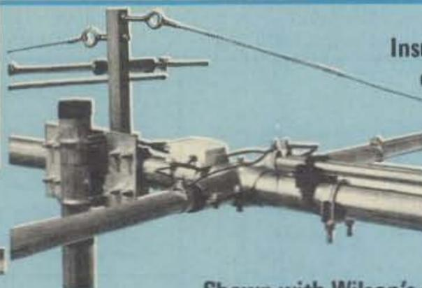
Insulated driven element with precision Beta match and heavy duty element mounts.
