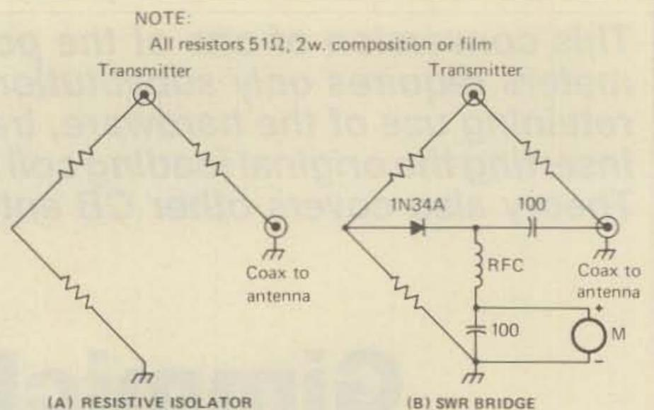
Fig. 4 - (a) "Isolator" prevents xmtr load from falling below 33 ohms or rising above 100 ohms, reducing chance of transmitter damage. (b) Addition of four parts and 0-1 mA meter changes the isolator to s.w.r. bridge.
