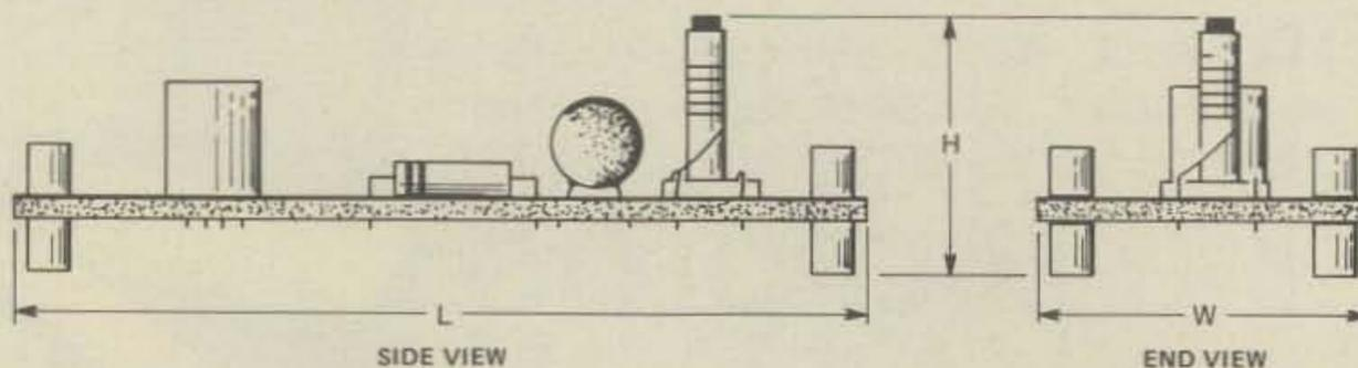
Fig. 3 - The size of an enclosure is a function of the dimensions of the printed circuit board with the components mounted on it. This figure shows how to make the measurements.
