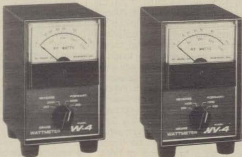
The Drake wattmeters shown here measure actual r.f. power output as well as reflected power. They can also be used to indicate radiated power (forward power minus reflected power) by means of a special nomogram provided with the units. The Model W-4 at left handles 2 kW to 54 MHz, while the WV-4 is rated at 1 kW to 200 MHz. (Photo courtesy R. L. Drake Co.)
