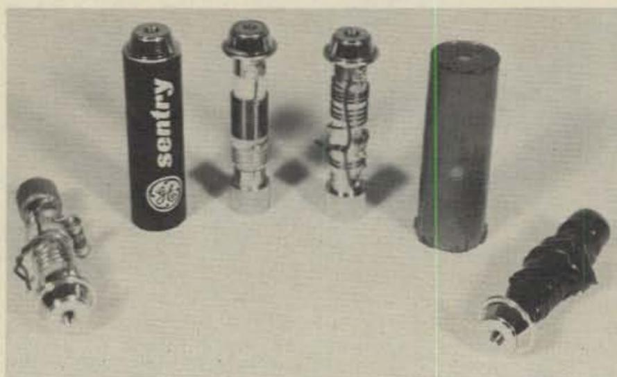
(L-R, rear) An unmodified loading coil, loading coil with cover removed, modified loading coil, pill bottle cover for completed unit. (Left side) Modified loading coil with external C<sub>1</sub>. (right side) Same type with electrical tape protection.
