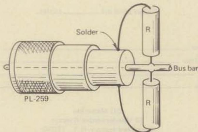
Fig. 1 - The "Poor Man's Dummy Load."
