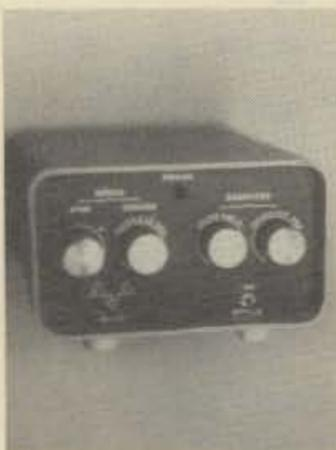
Positioning of simultaneous notch filter is continuously variable from 300 to 1400 Hz with FINE and COARSE position controls. Notch depth is fixed at nominally 30 dB. Notch tuning is independent of bandpass tuning and may be completely disabled.
