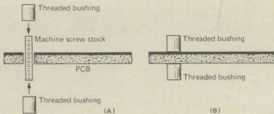
Fig. 2 - Using a machine screw and threaded bushings to mount a printed circuit board.
