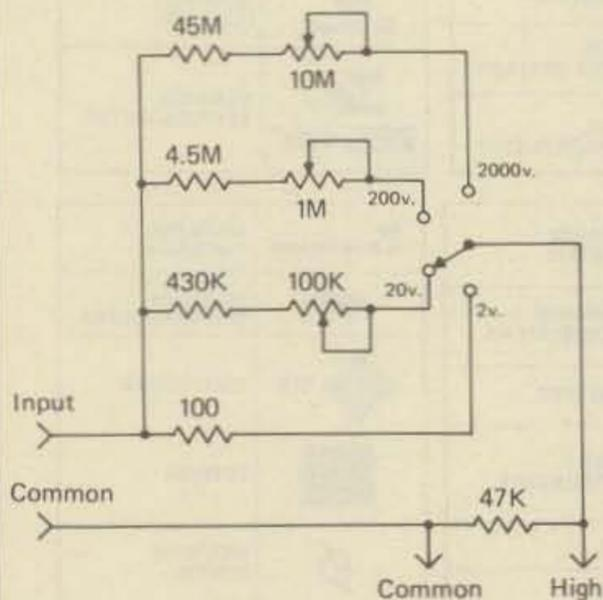
Fig. 2— Modifying the input as shown results in a multi-range instrument.
