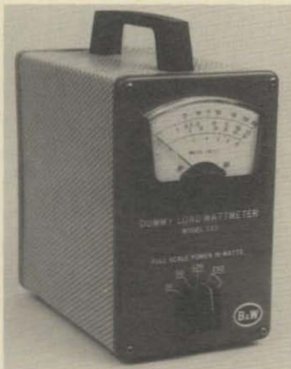
This lightweight, air-cooled Barker and Williamson dummy load/wattmeter will handle power output levels to 250 watts. It presents the transmitter with an s.w.r. of less than 1.3 to 1 up to 230 MHz, and it can be used as high as 300 MHz. Note the four selectable wattmeter ranges—10, 50, 125, and 250 watts. The low-range selection makes it useful in checking QRP rigs, CB transceivers, and v.h.f. handi-talkies in addition to Novice-powered h.f. transmitters. (Photo courtesy B&W).
