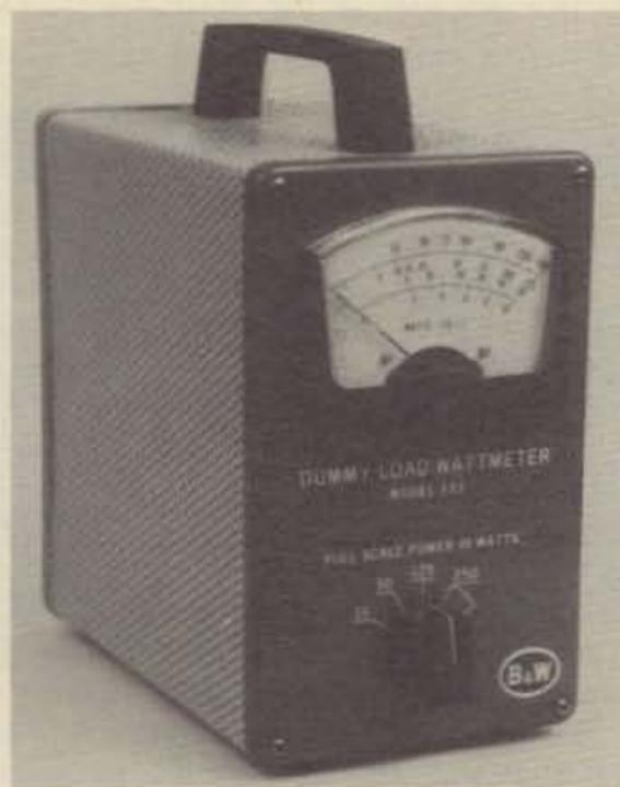
This lightweight, air-cooled Barker and Williamson dummy load/wattmeter will handle power output levels to 250 watts. It presents the transmitter with an s.w.r. of less than 1.3 to 1 up to 230 MHz, and it can be used as high as 300 MHz. Note the four selectable wattmeter ranges—10, 50, 125, and 250 watts. The low-range selection makes it useful in checking QRP
