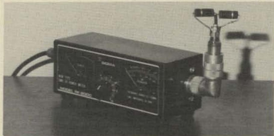
Home-made low-power v.h.f. dummy load is shown mounted to the side of Sigma RF-2000 s.w.r. bridge/wattmeter. The dummy load shown in the photo differs slightly from that of fig. 1. In this one, it is actually mounted on an RCA-type phone plug which in turn slips into an RCA-to-coax-connector adapter. Thus, the little dummy load can be used both with transceivers having RCA or standard coax fittings.
