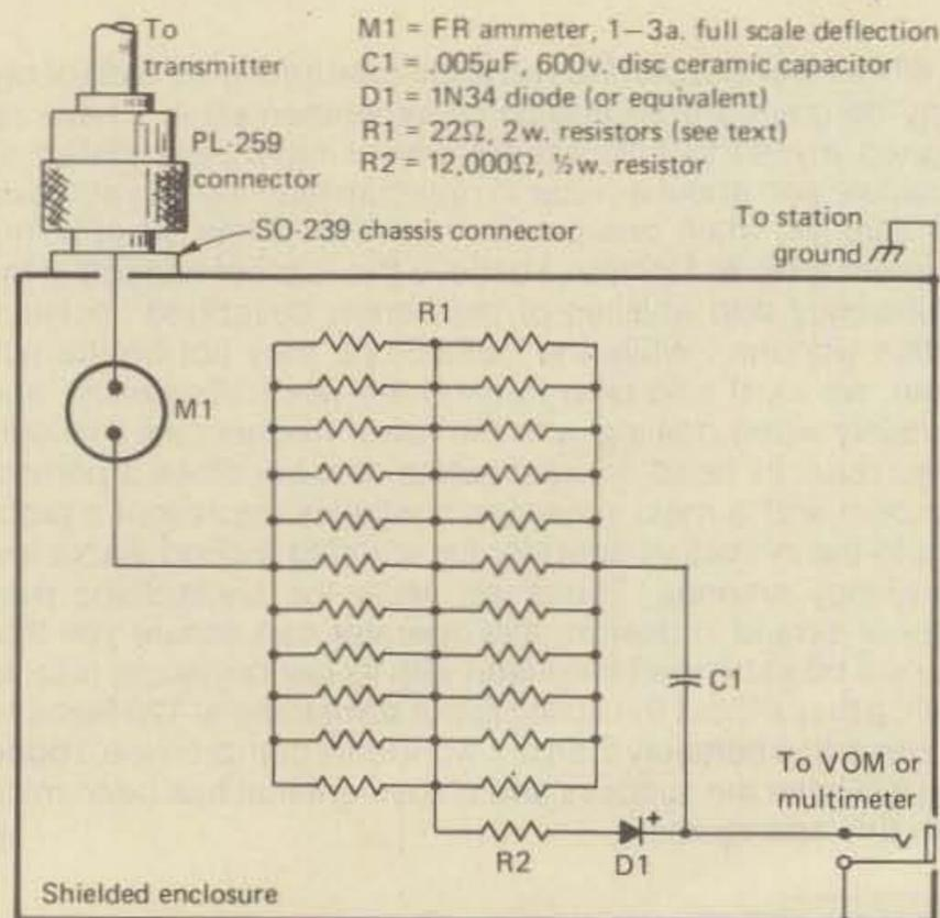
Fig. 2 - A 100-watt dummy load.
