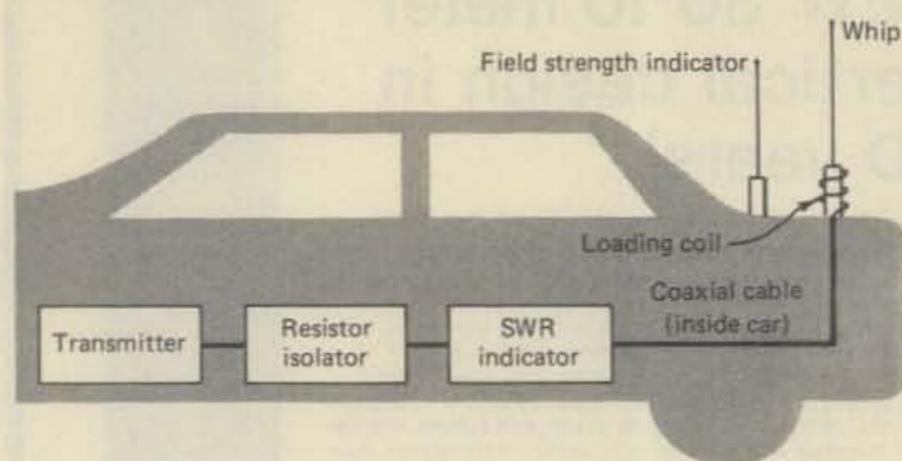
Fig. 5 - Transmission line, transmitter, s.w.r. bridge, and isolator should be inside the car during adjustments.
