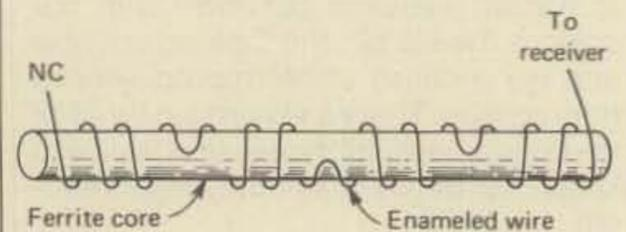
Fig. 4— The v.h.f. ferrite rod antenna as described in the Jan. 1978 issue of Electronic Design.
