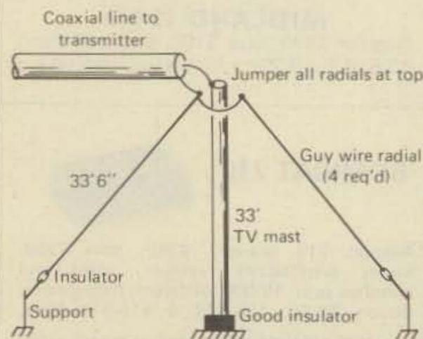
Fig. 4 - The K6WG "inverted vertical" antenna for 40 or 80 meters is an upside down ground plane, fed at the apex.
