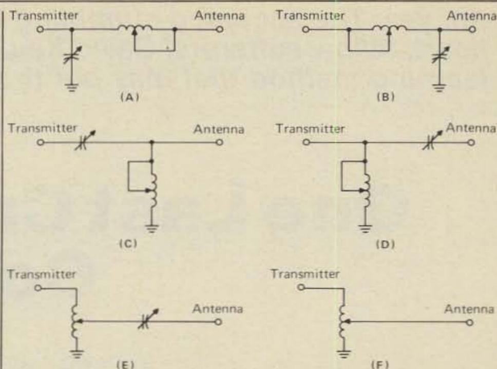
Fig. 2 - These are the main networks which can be formed by interconnections of the binding post matrix.
