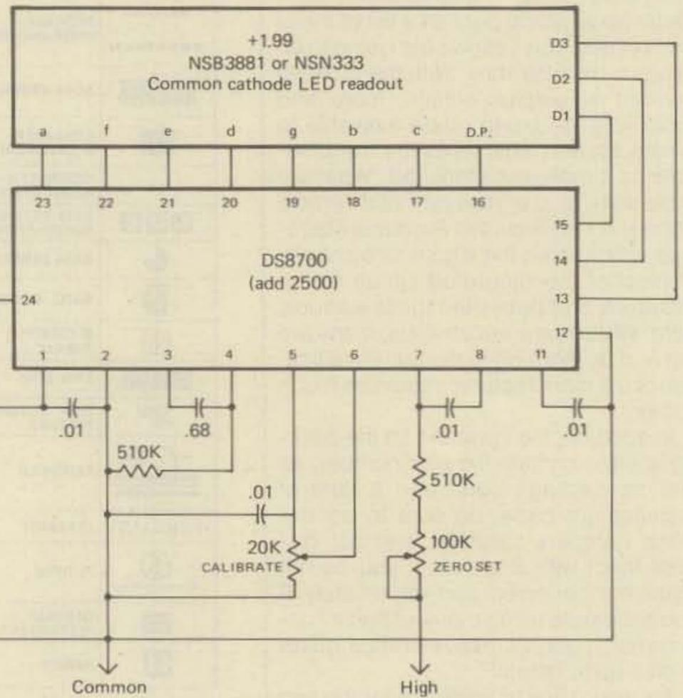
Fig. 3— By adding three components, the meter will measure a.c.
