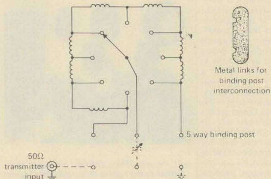
Fig. 1 - A binding post matrix is the key to the versatility offered by the antenna tuner.
