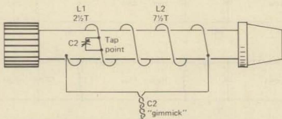
Fig. 3 - Layout of the coil. Solder is puddled into the hole in the coil form to contact the "tap point."
