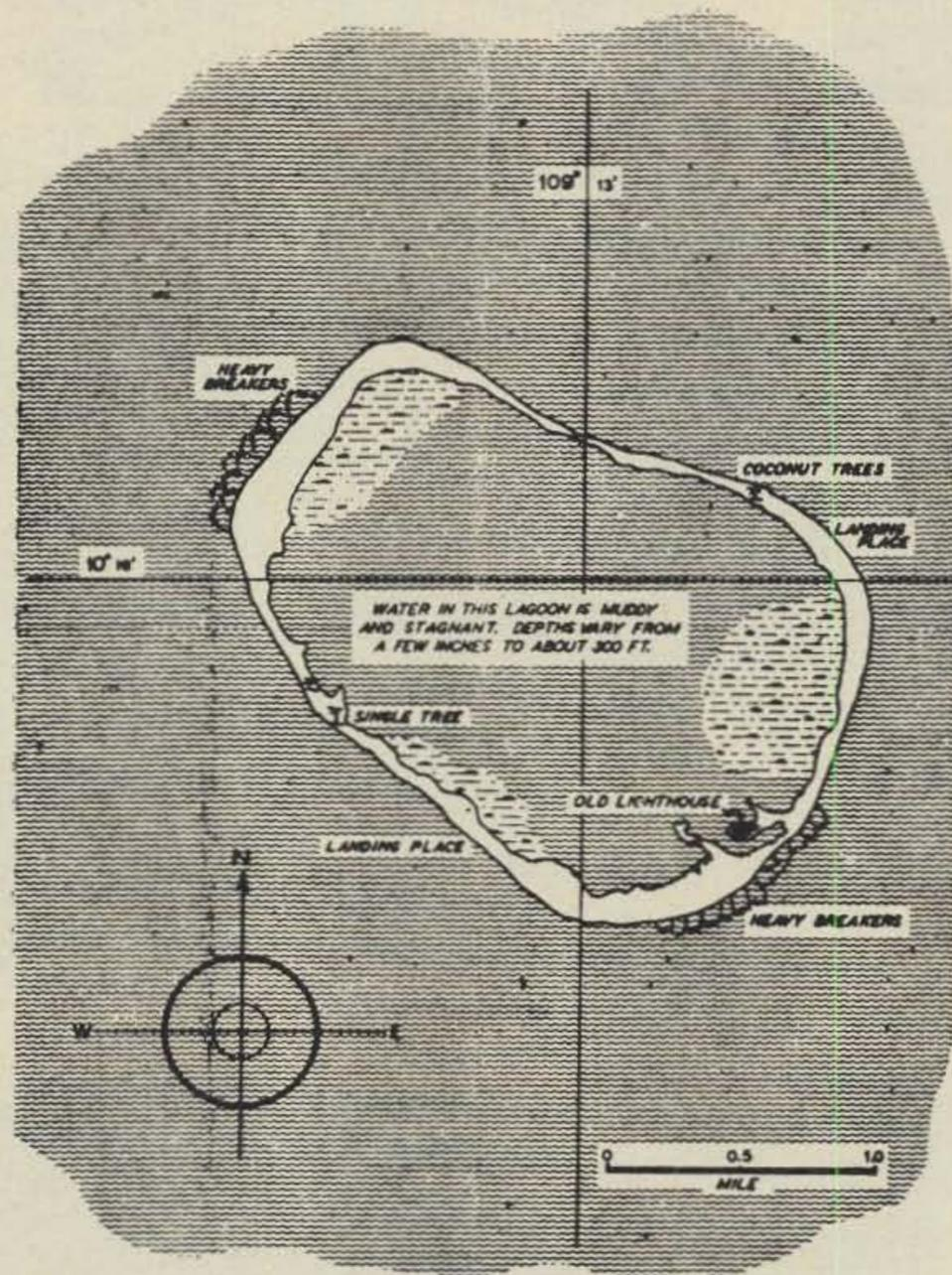
*A hydrographic chart of Clipperton Atoll. The water in the completely enclosed lagoon is muddy and stagnant, and ranges in depth from a few inches to about 300 feet. The "island" is the top of an active volcano, whose sides fall precipitously to a maximum depth of over 3,100 feet. This, in addition to the reef-like framework of the atoll, which is surrounded by heavily breaking surf, makes anchorage and landing very difficult.*
