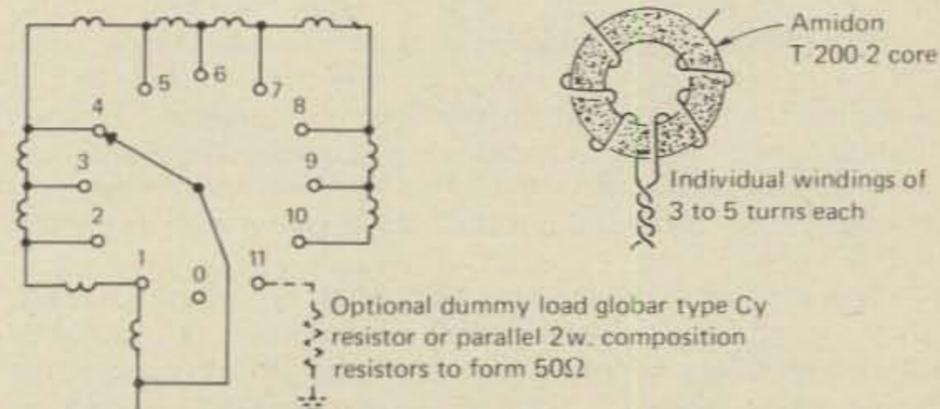
Fig. 3 - Details of winding the tapped, toroid inductor. Further information is given in the test.
