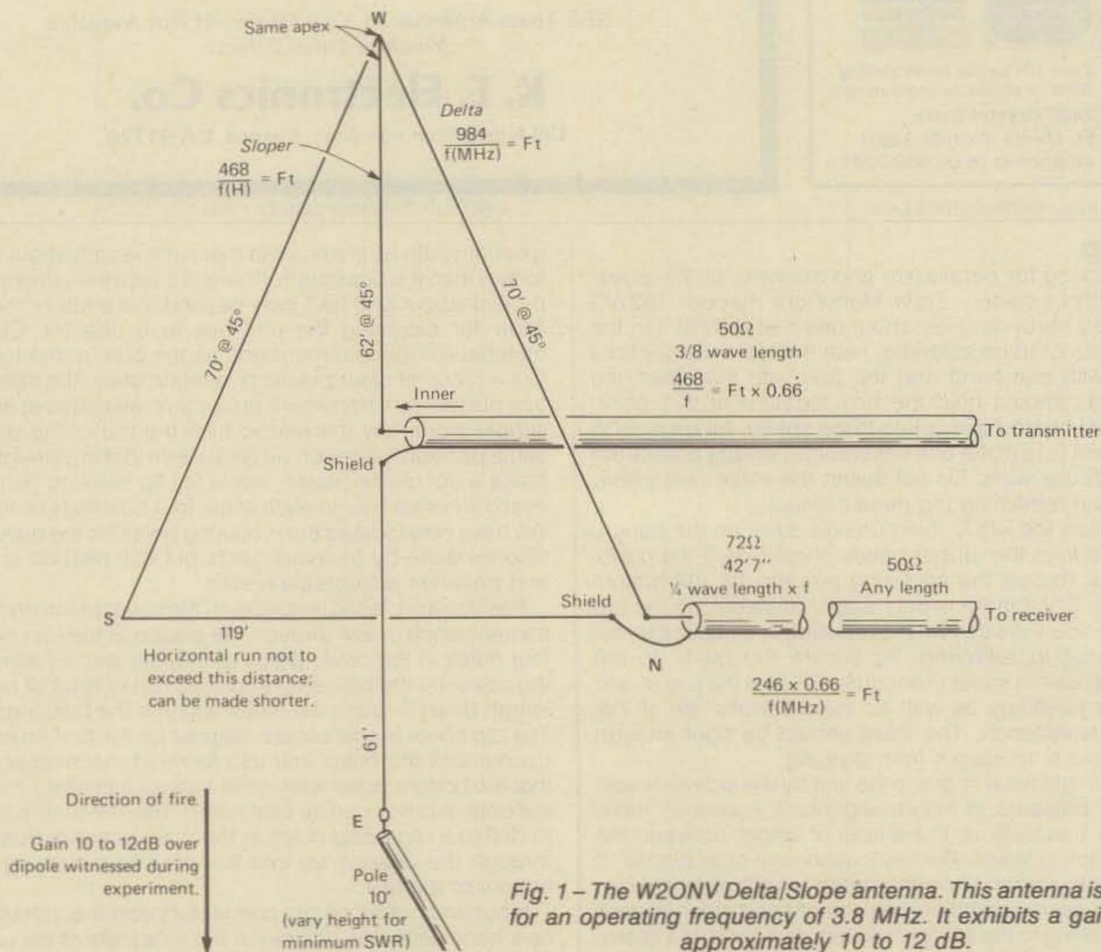
Fig. 1 - The W2ONV Delta/Slope antenna. This antenna is cut for an operating frequency of 3.8 MHz. It exhibits a gain of approximately 10 to 12 dB.
