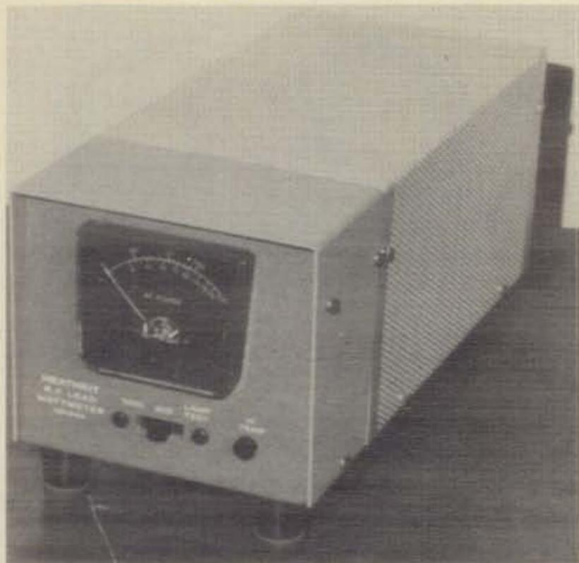
Heath HM-2103 (now discontinued) combines the functions of the dummy load and the r.f. wattmeter. This air-cooled load handles power levels to 1000 watts, and allows r.f. wattmeter readings of transmitter power output on either a 200- or a 1000-watt scale, depending on the range selected. At the heart of the unit is a 50-ohm heavy-duty, non-inductive carbon load resistor. The unit is protected against overloading or overheating by means of a thermal switch.
