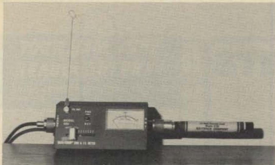
CB s.w.r. bridge and field-strength meter shown here works well up to at least 2 meters in both applications. The Raytrack 10-watt dummy load was designed for 27 MHz CB and commercial use, but the author has found it useful as a 2-meter dummy load. It fills the gap between the small 5-watt CB-type dummy loads and the heavy-duty, high power loads designed for h.f. transceiver loading; I use it with a Yaesu FT-221R 2-meter transceiver, which has a power output of about 12-14 watts.
