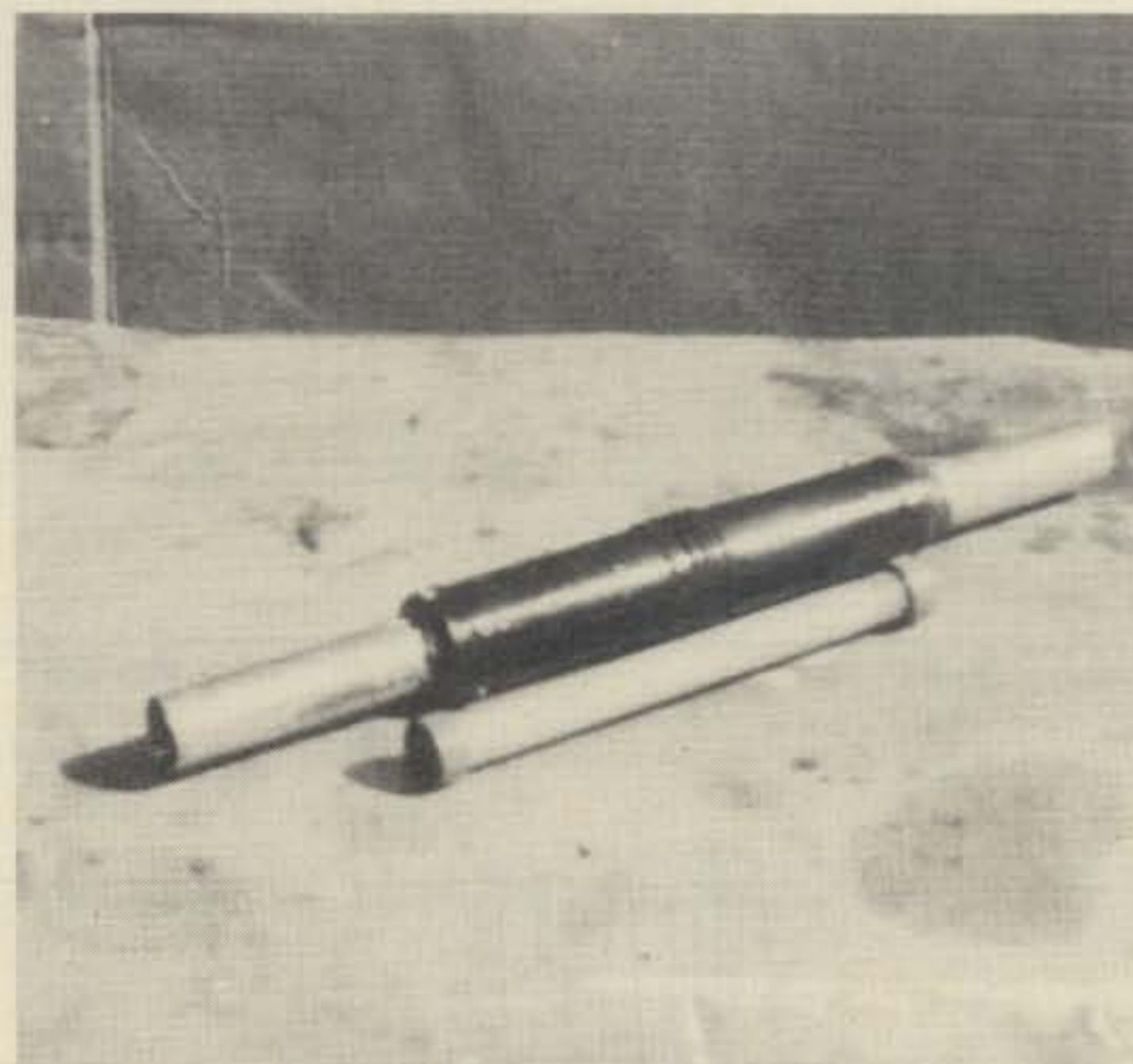
A typical trap coil and the "capacitor" tube that fits inside the coil section.
