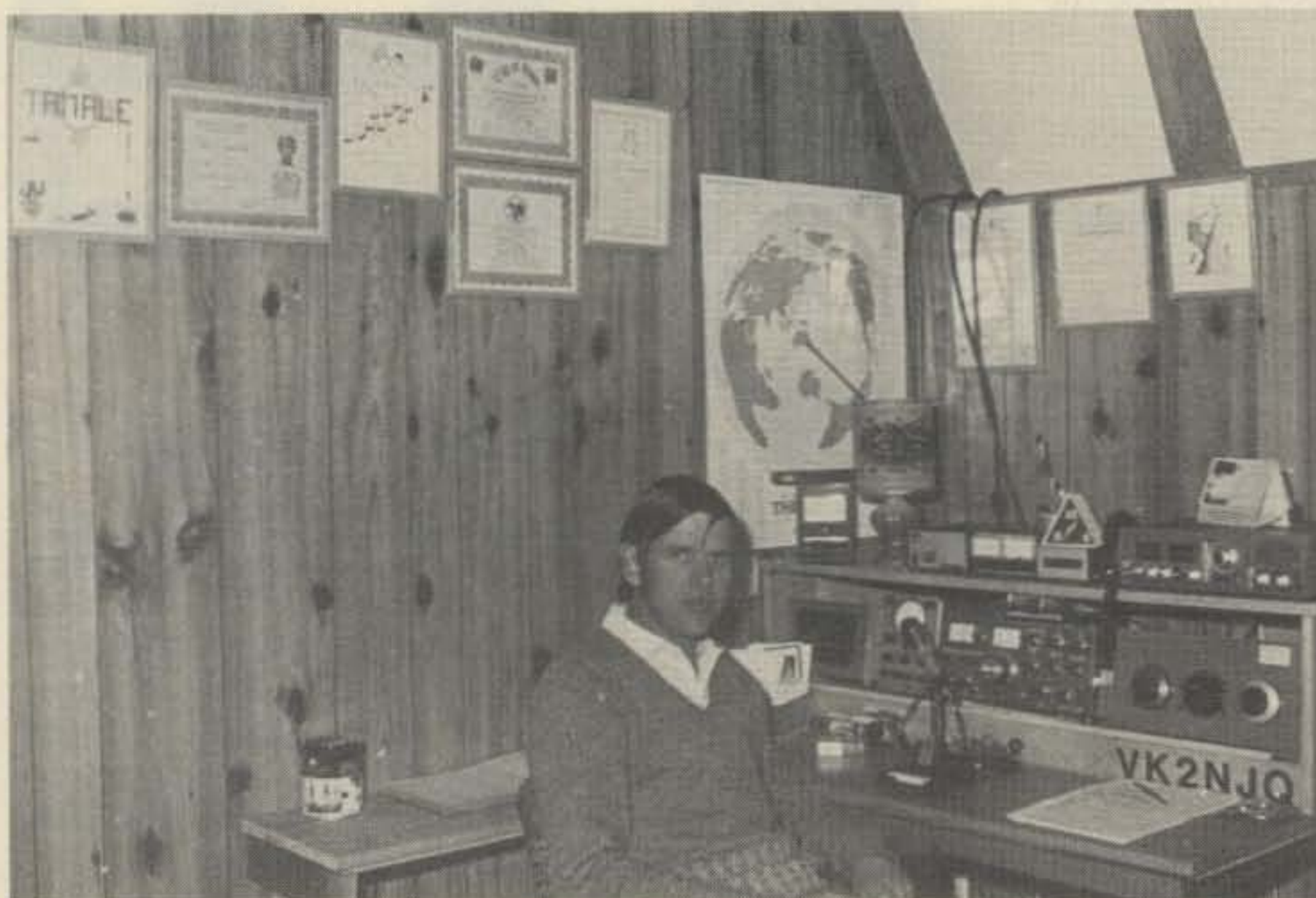
This is Australian Novice Peter Jeffery (VK2NJQ) of Bullaburra. The main item in his station is the Kenwood TS-520 and his antenna system includes a quad for 10 and 15 meters. VK2NJQ uses the 10 meter Australian Novice band (28.1-28.6 MHz.) to work American and other DX. He works many European amateurs on the 15 meter Australian Novice band (21,125-21,200 kHz.) and he uses his 80 meter band (3525-3775 kHz.) to work Australian, New Zealand, and other closer contacts.
