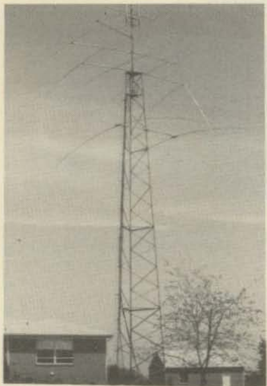
Fig. 5 — Another view of the K3WX antenna system. In this view Tony has added an inverted-V for 40 meters at the end of the 20 meter boom, plus a two element log-periodic antenna at the 85 foot level for 80 meters.
