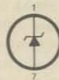
Fig. 6 - A Zener regulator which replaces an OA2 or OB2.
