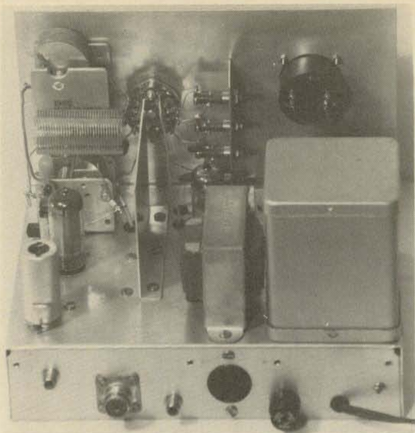
An alternate rear view of the transmitter, also showing parts placement. Along the rear edge of the chassis are, from left to right, the receiver antenna jack, the antenna coax jack, the v.f.o. input jack, the auxiliary power socket, fuse, and line cord.
