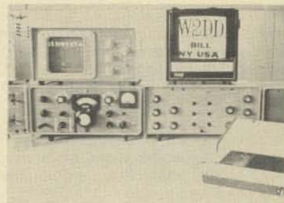
Fig. 4 - A side by side comparison further illustrates the difference between viewing an SSTV picture via a P-7 monitor (on the left) versus the scan converted image shown on the conventional monitor (at the right). The scan converter in this picture (under the monitor) is no longer manufactured Robot Research Model 300 scan converter which uses a cathode ray storage tube.
