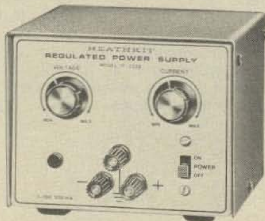
A small, regulated power supply is useful for bench checkout of d.c.-powered kits and for servicing of low-voltage solid-state equipment. This particular unit can be built from a kit and provides voltages from 1 to 15 v.d.c. at one-half ampere. (Photo courtesy Heath Co.)
