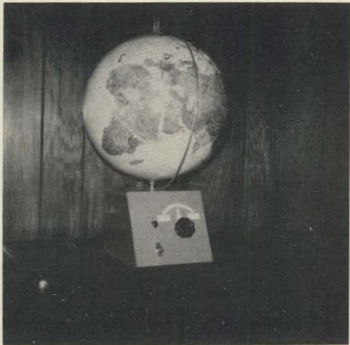
The direction indicator, showing the path of the beam from top to bottom.
