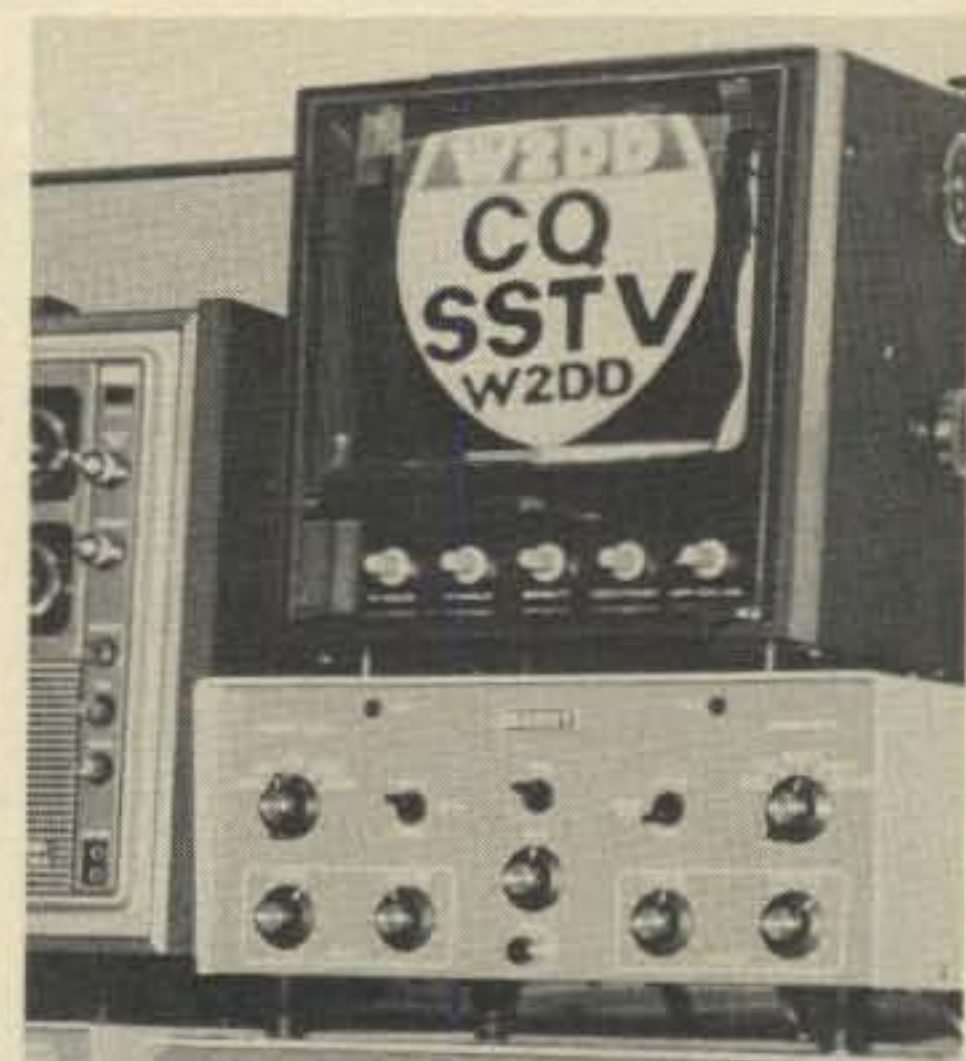
Fig. 5 - The compact gray box under the TV monitor displaying W2DD's CQ is the current Model 400 Digital Scan Converter by Robot Research Inc.
