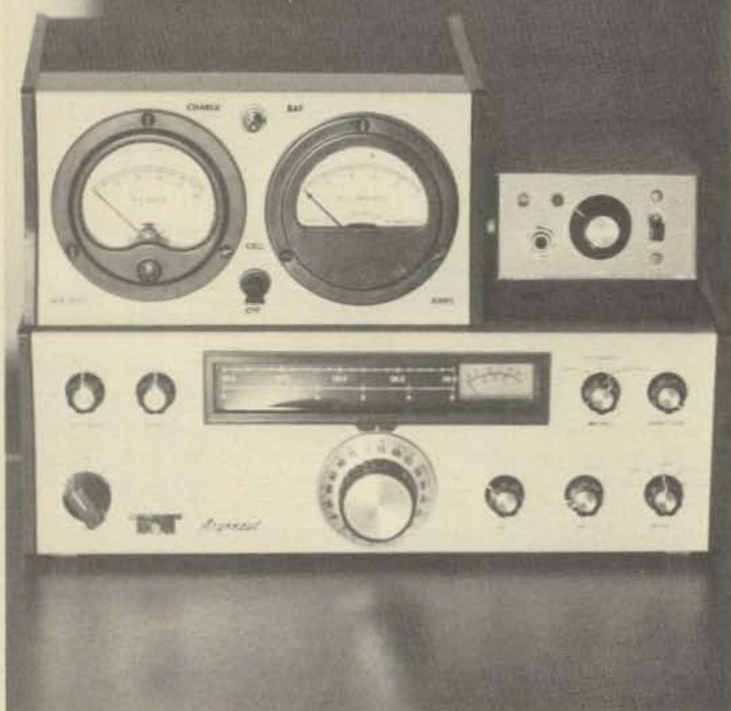
The complete QRP solar-powered amateur station. The regulator is on top of the Argonaut; the small unit to the right is the VOMAX SBP-3 speech processor.
