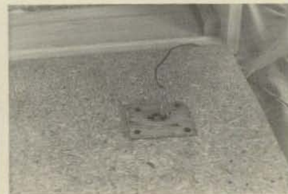
The phono jack is attached to a piece of 1/8" plywood and glued over the inside of the panel opening.
