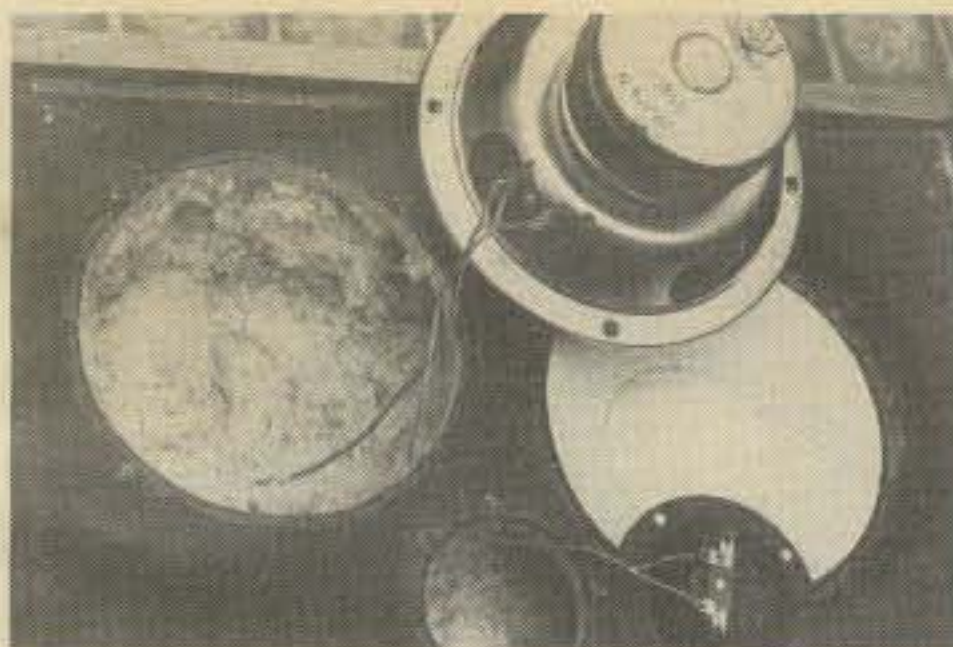
The zip cord from the enclosure is attached to the woofer and an additional length joins the woofer and tweeter. Note the absorbant material in the enclosure.
