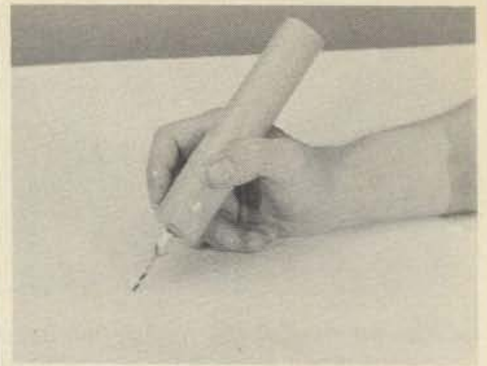
A precision rechargeable high-speed drill is useful in cleaning up holes in p.c. boards and in repair work, too. A unit such as the Radio Shack drill shown above can also be used for jewelry working, models and other hobby purposes. The drill speed is rated at 28,500 r.p.m.
