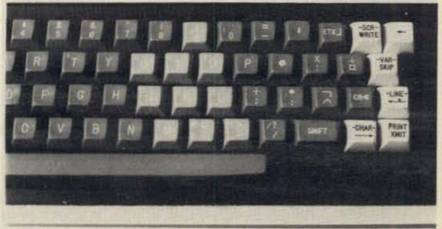
A computer terminal's keyboard has several added keys you won't find on an ordinary typewriter. Otherwise it's similar. An important key always used is the CR or Carriage Return key, shown at right.
