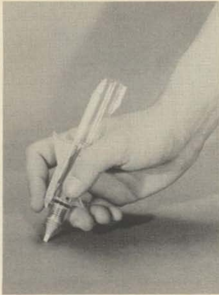
Make a wiring mistake on a fragile p.c. board? This mini vacuum pump makes it easy to desolder and correct mistakes without making a mess. (Photo courtesy Radio Shack)
