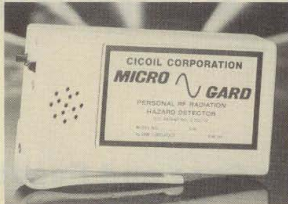
Belt-attachable r.f. radiation monitoring device (Cicol Co., Chatsworth CA). If r.f. power density incident exceeds a factory set level, an audio alarm is actuated within the unit. Its dimensions are 4.2 x 2.2 x 0.84 inches.
