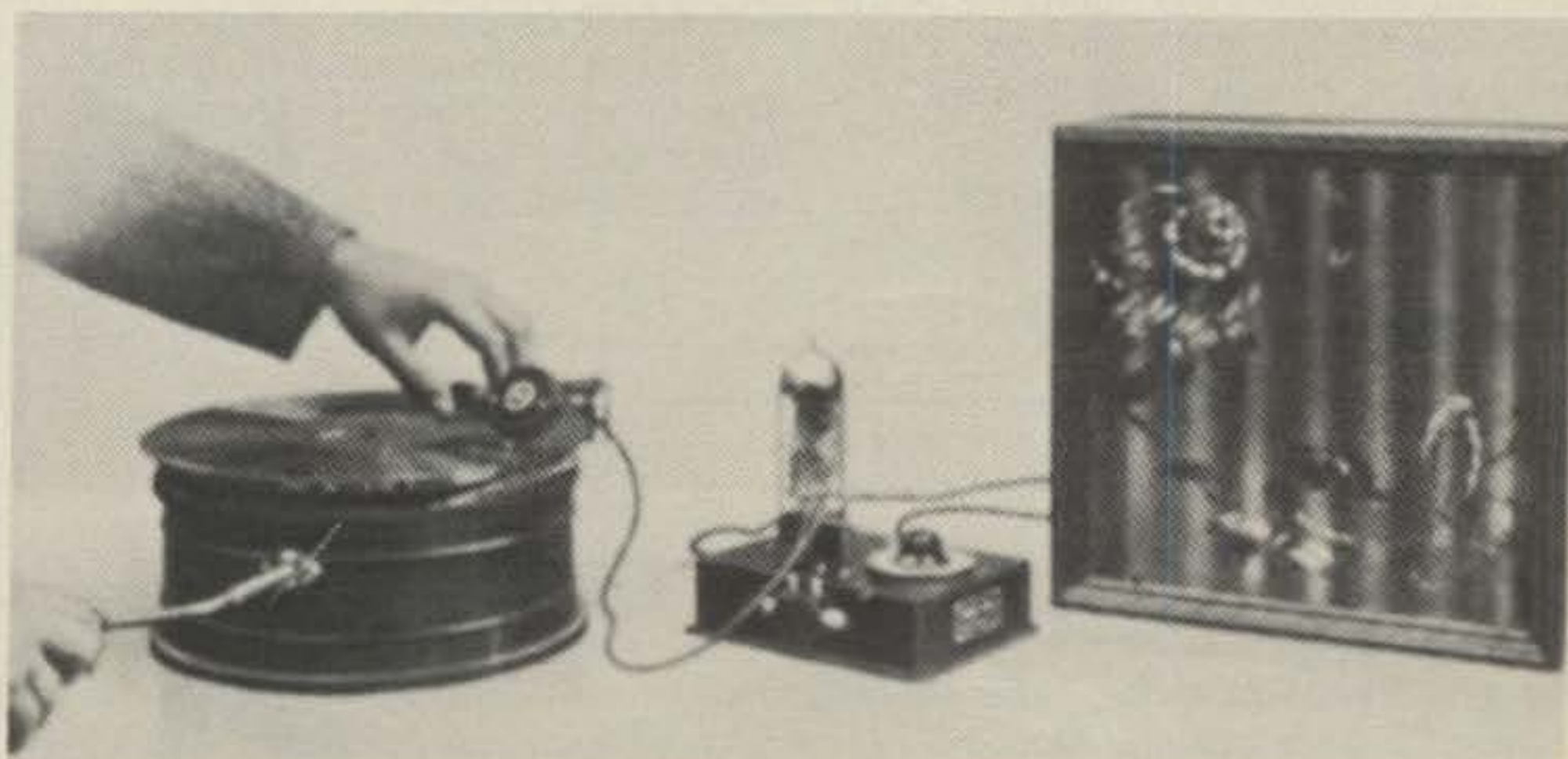
Fig. 4-A 1928 version of the OE333 in use as an amplifier for record playing equipment. Note the hand-cranked turntable.
