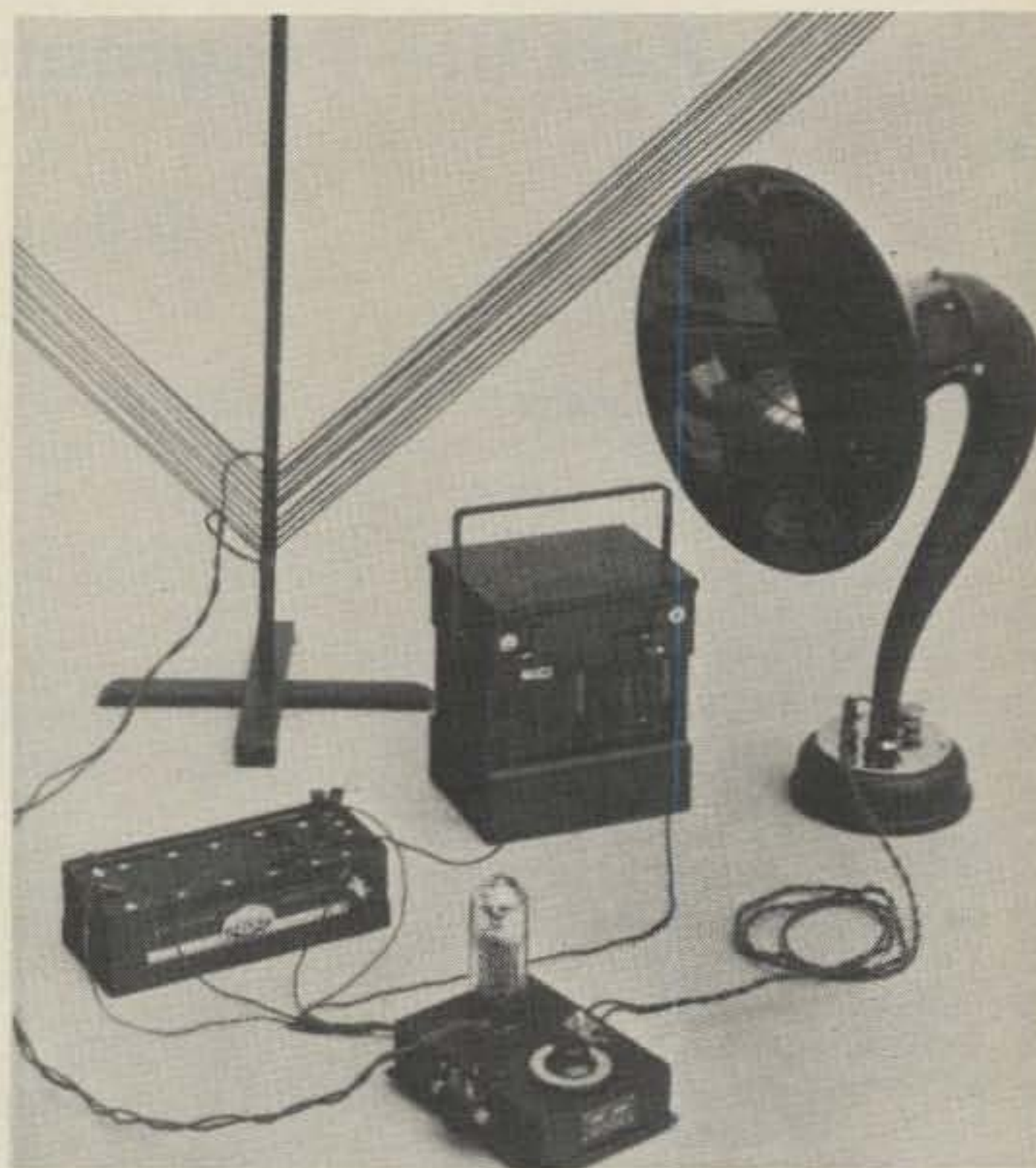
Fig. 3-The Loewe OE333 IC radio with batteries, frame aerial and speaker.
