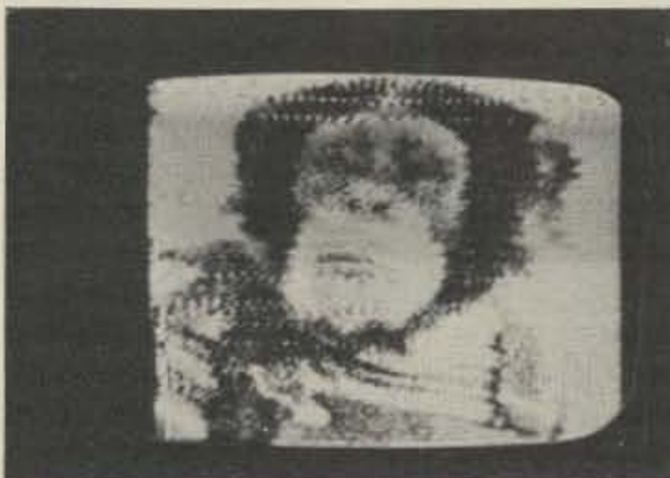
The QRM level during the reception of this picture was 20 dB above the desired signal. Interference is more severe from the nearby voice signal which was splattering over. The offending station was about 10 kHz wide and had products throughout the band; but, as you can see, the picture came through. One of the nice things about SSTV and digital scan converters is the ability to punch through under all but the worst conditions.
