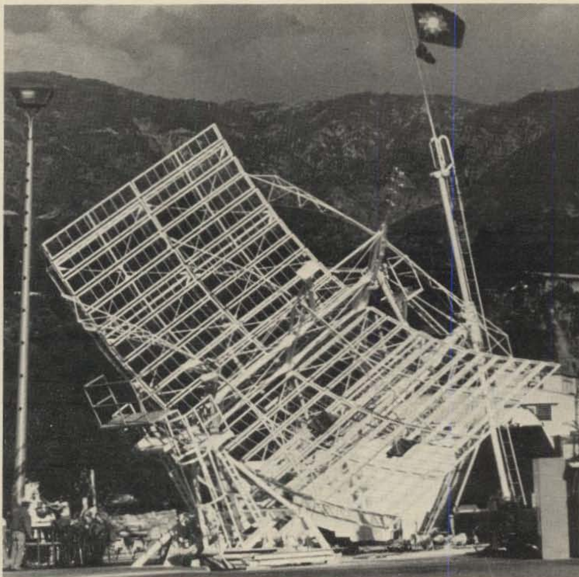
The Sunfire Project takes shape in the form of a solar thermal electrical generator at JPL.
