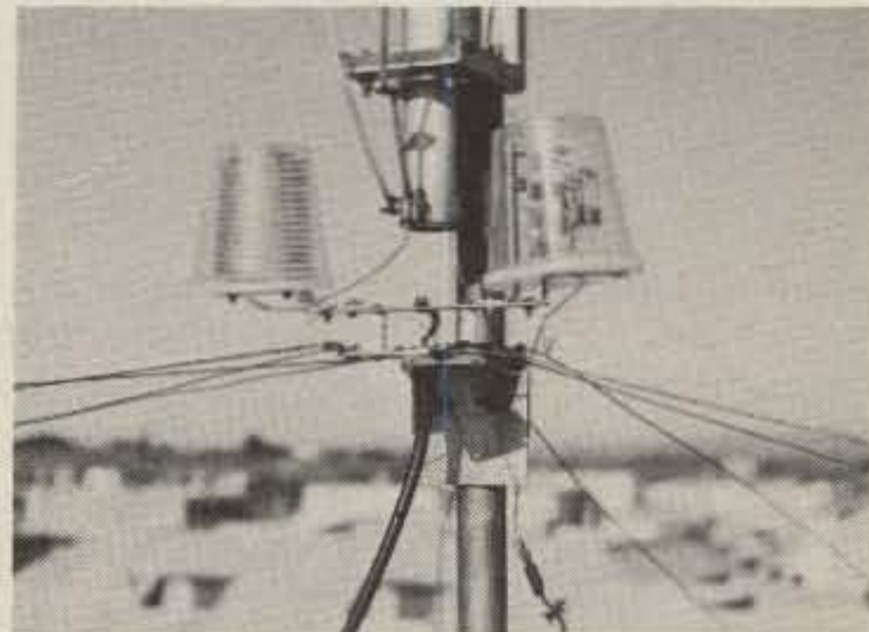
Fig. 5-The base loading coil of the vertical antenna is placed in a plastic cup as is the relay which places the coil in the circuit. Francesco reports good DX with this antenna on all high frequency bands: 80 through 10 meters.
