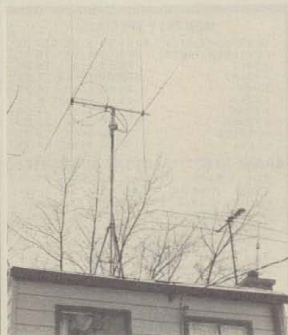
Fig. 2 — The dual-polarity Avanti 10 meter Quad at WD9ABG. This novel antenna provides either horizontal or vertical polarization at the flick of a switch. Matching sections are folded into a loop at the center of the director. Switchable polarization is very useful for DX work says Marty.
