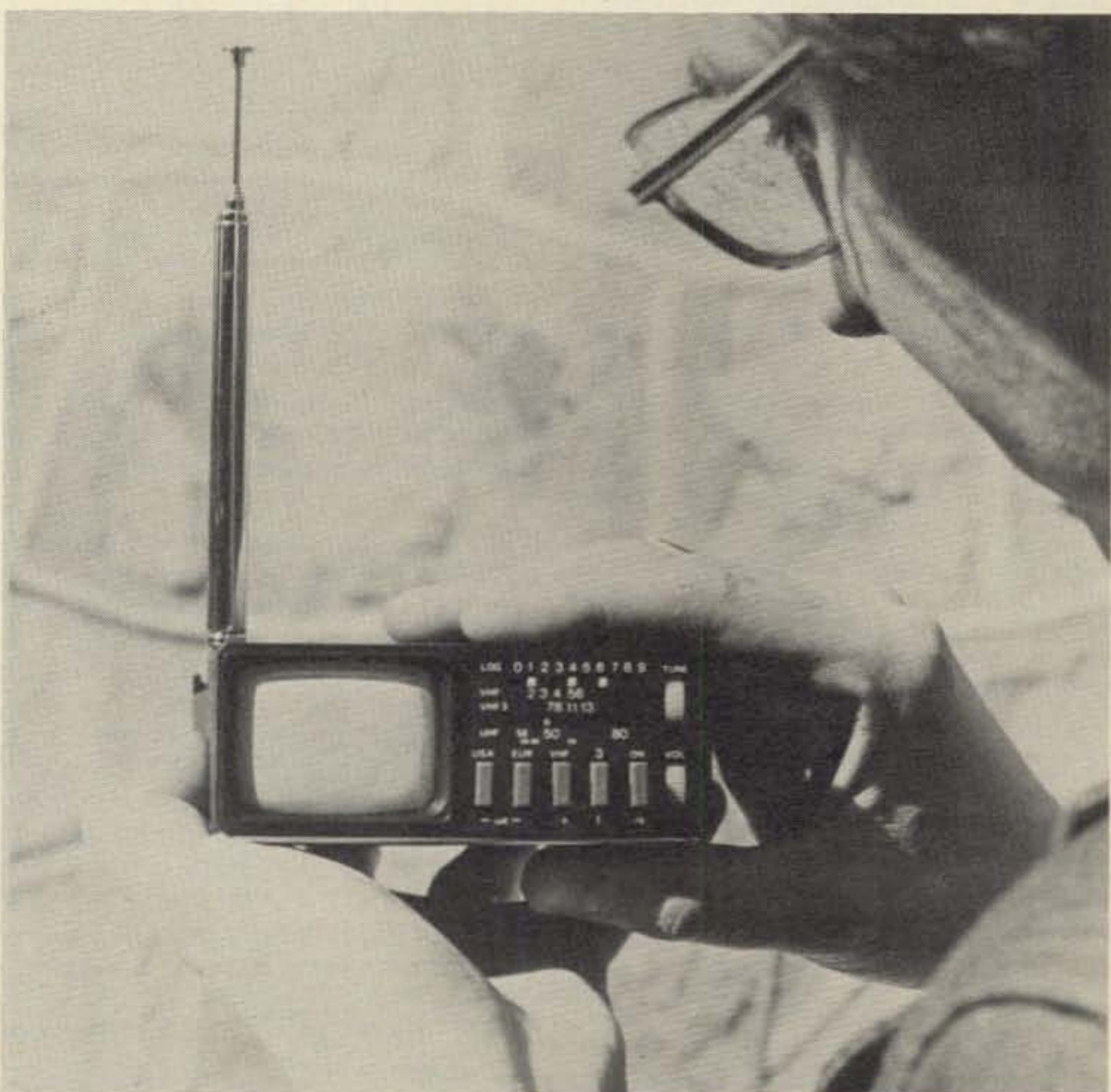
A true palm-of-the-hand television receiver, including the internal battery pack.
