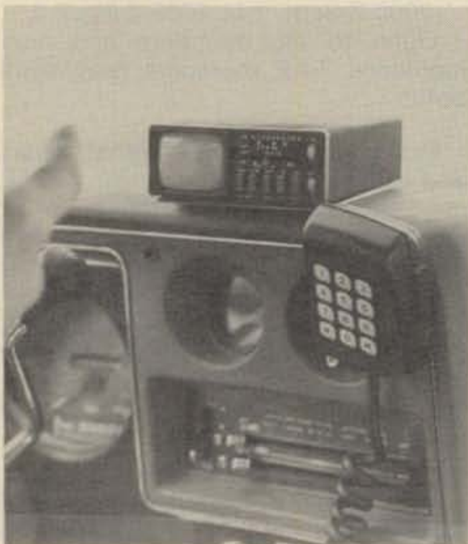
The microtelevision is easily mounted above the dash for mobile testing and TVI search purposes.
