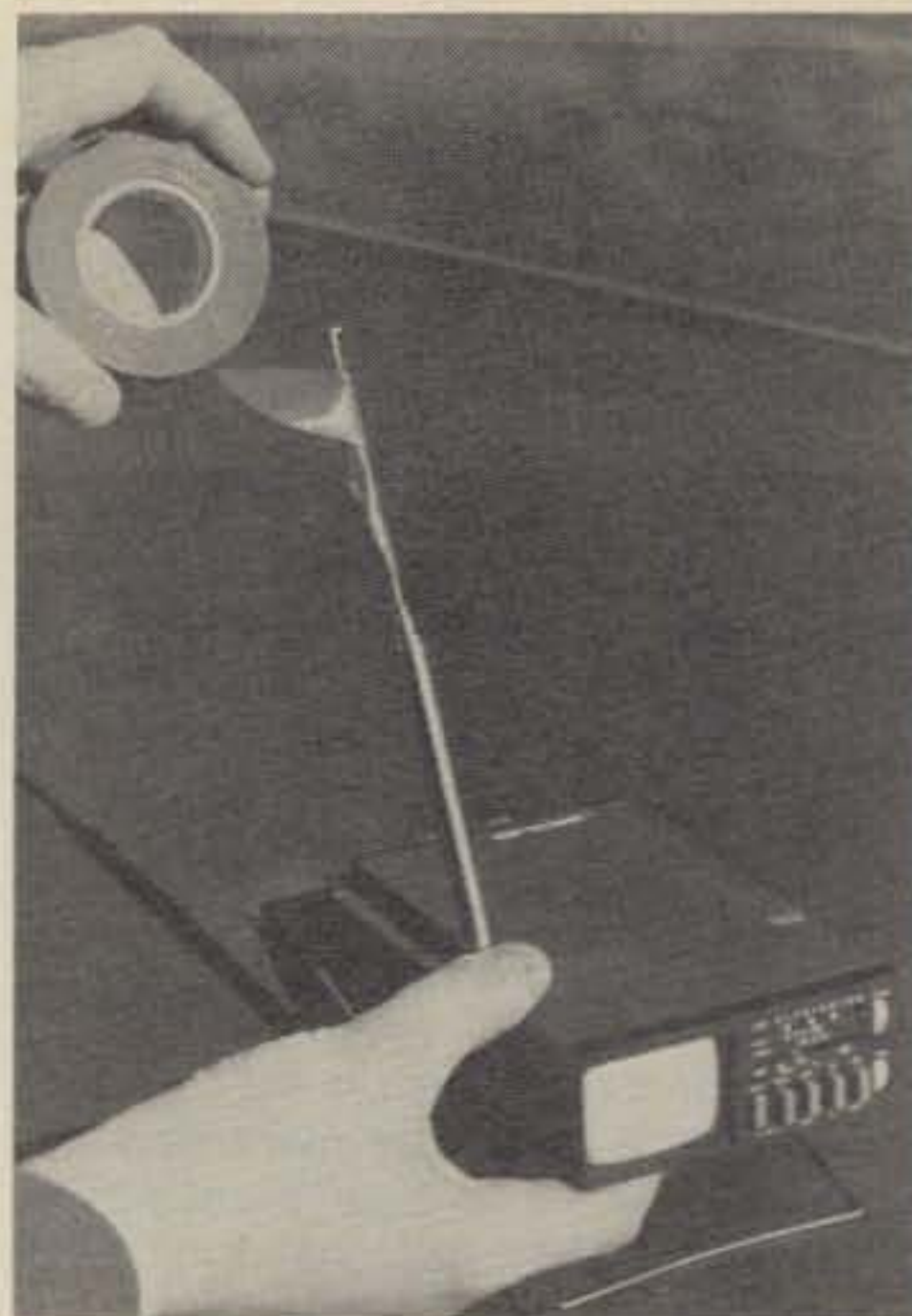
The whip antenna is wrapped with electrical tape to form a d.c. insulated probe.
