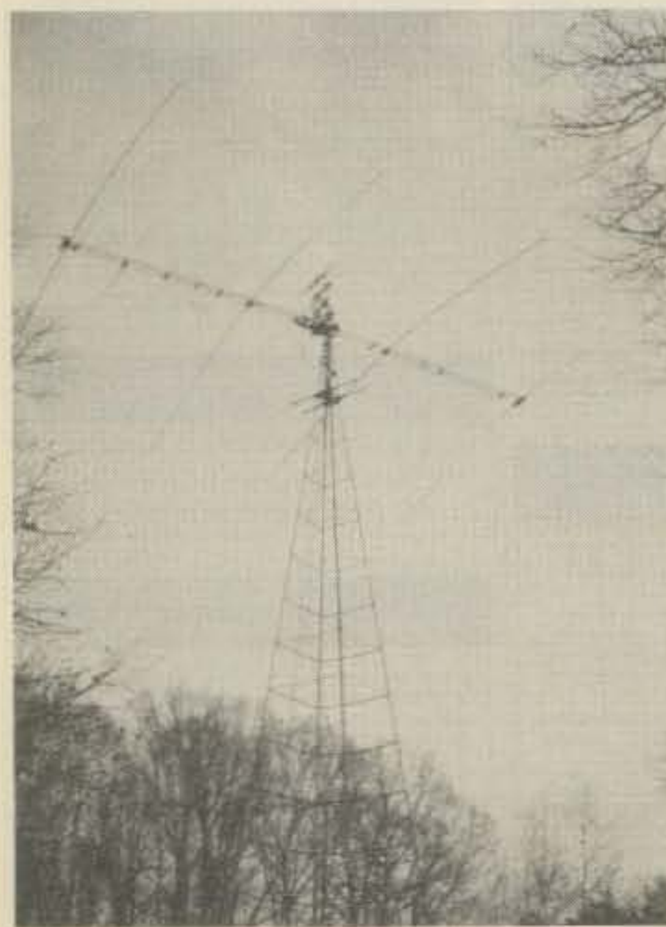
Fig. 1-The antenna farm at DXer W3GRF. A four element 40 meter beam with eight interlaced 10 meter elements on a 70-foot boom (photo by K4VX).
