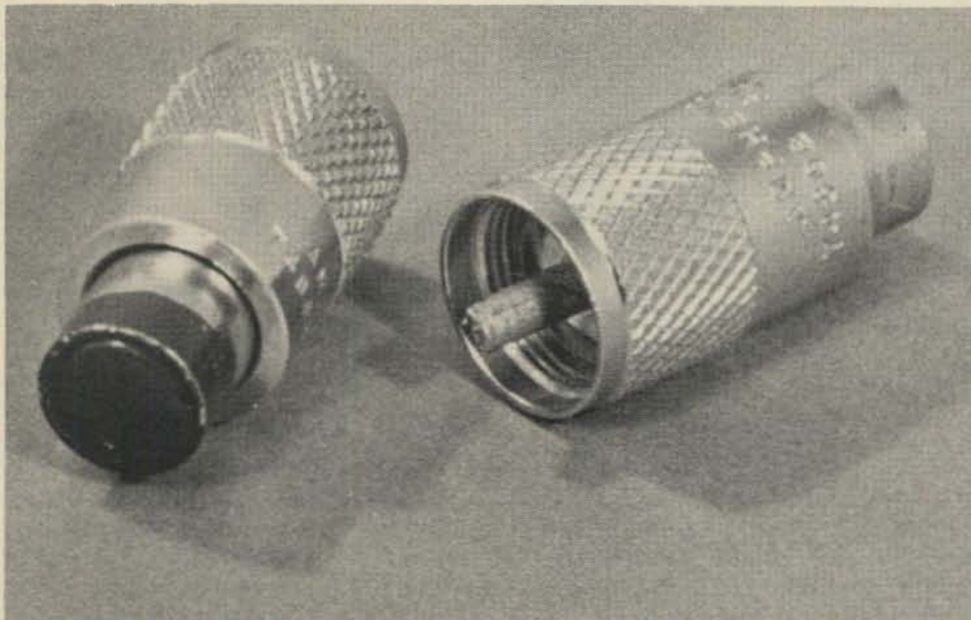
Test loads are easy to make out of two-watt resistors and PL-259 antenna connectors. The load at the left is made with a 100-ohm resistor and lets the s.w.r. bridge "see" a 2.0:1 mismatch. The load at the right is 50-ohms and lets the s.w.r. bridge "see" a 1.0:1 match. It is used for checking low powered transmitters.
