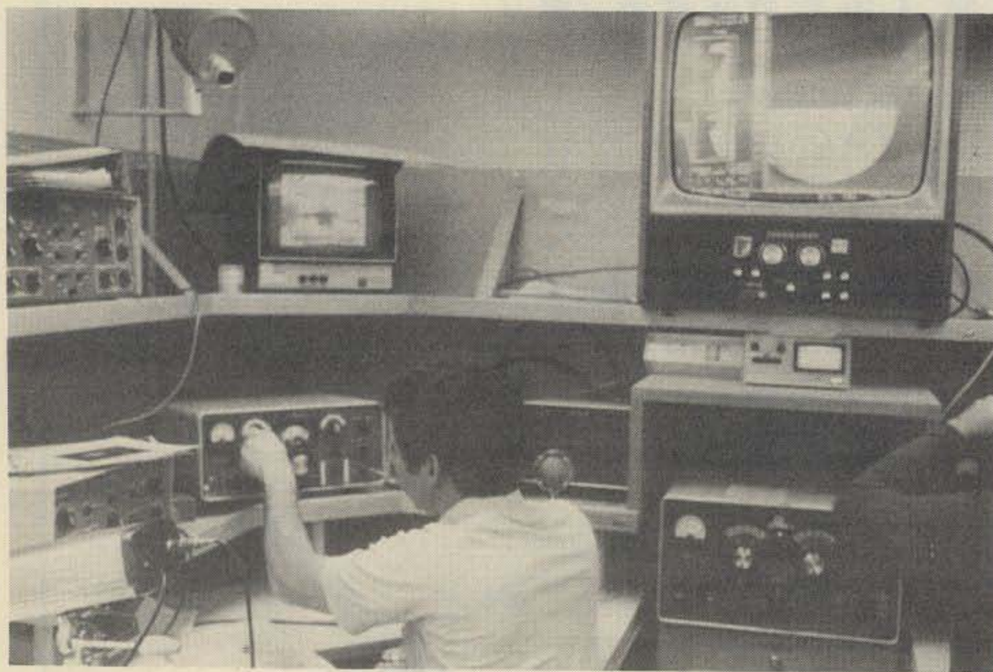
Mike Griffin, N6WU, operates s.s.t.v. On the left is the JPL Voyager monitor; on the right the s.s.t.v. monitor.
