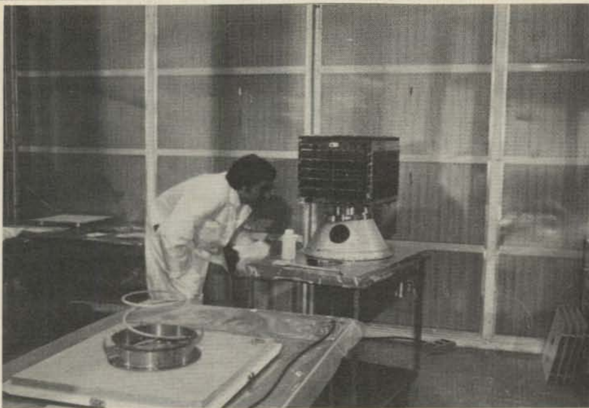
Jan King examines the OSCAR-8 spacecraft during preparation for launch. The release spring is in the foreground.
