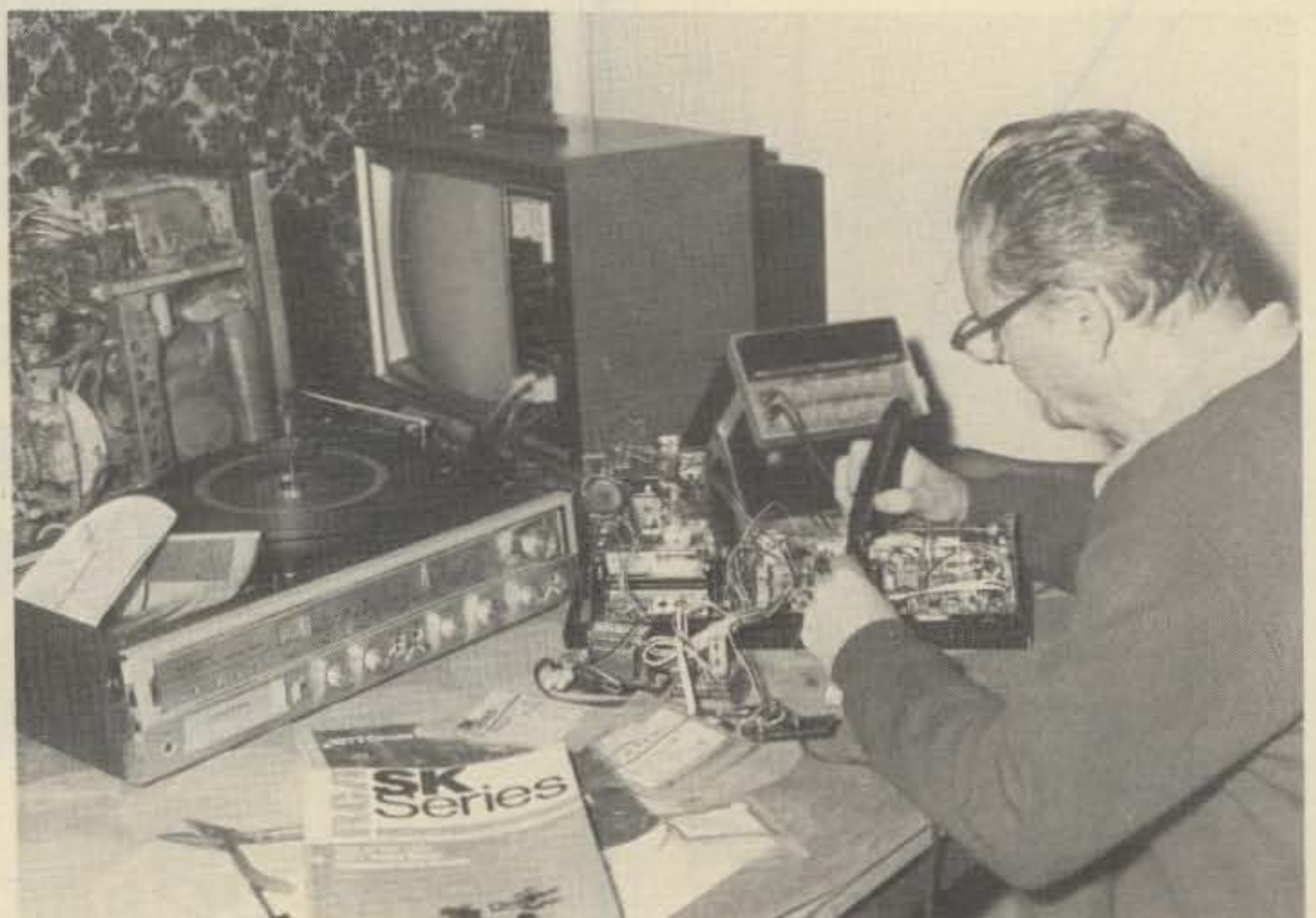
Photo 1 - Before the unit can be placed into operation, the defective transistor must be located, removed, tested, a replacement found and installed properly. Here, we find an electronic technician soldering in a transistor of a radio chassis.
