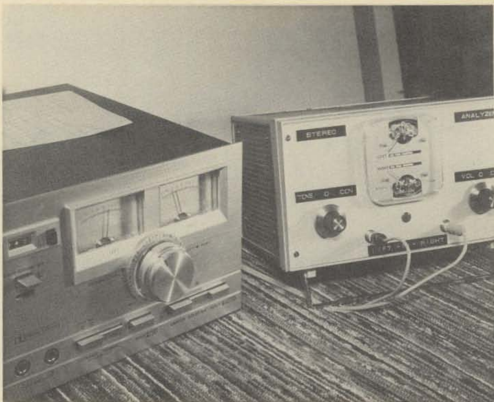
Photo 4 - Besides regular test equipment a stereo or separate amplifier may be used to locate a defective audio transistor stage.
