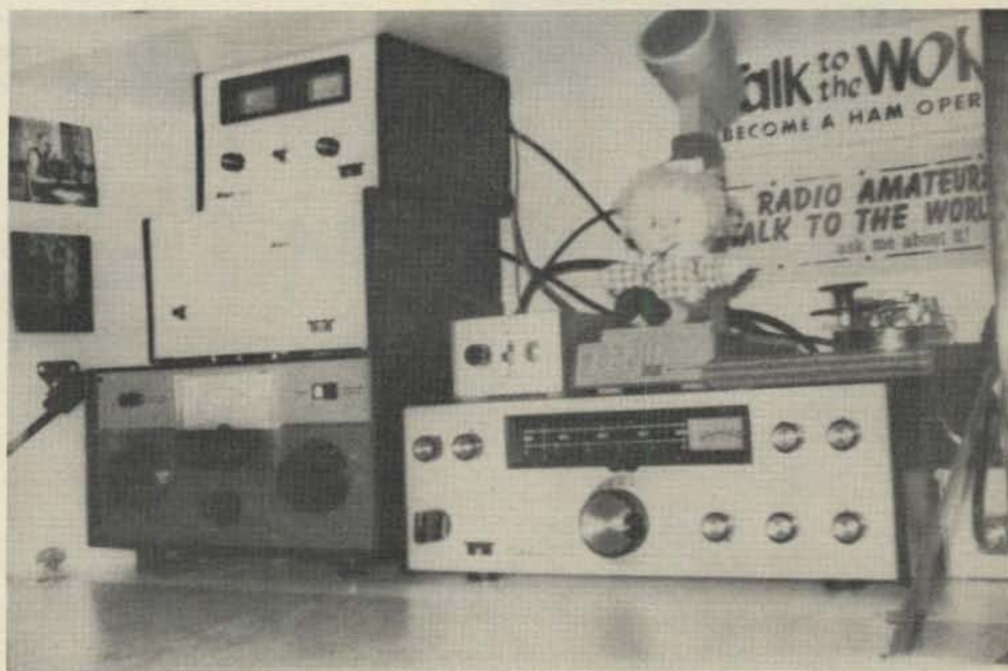
Here is a shot of WB2JII's neat QRPp station. Atop the Argonaut are a straight-key for c.w., a mike and MFJ speech processor for s.s.b., and the shack mascot. The Drake MN4 matchbox is topped by the TenTec power supply and 405 linear. A couple of CQ bumper stickers are on the back wall. The console should be of interest to those of you with problems with a decor-minded XYL who objects to "all that radio junk in my living room." The complete station is located inside a wooden cabinet, and the front panel of the cabinet is lowered to form a desk top when operating, closed to simulate furniture when not operating. Slick!!
