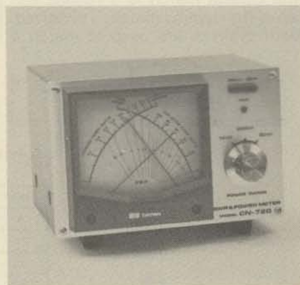
Fig. 5-The Daiwa Model CN-720 dual s.w.r. and power meter. A dual pointer meter provides instantaneous readings of forward and reverse power. The point the meter pointers intersect shows s.w.r. on a third scale. Meter operates at power levels up to one kilowatt.
