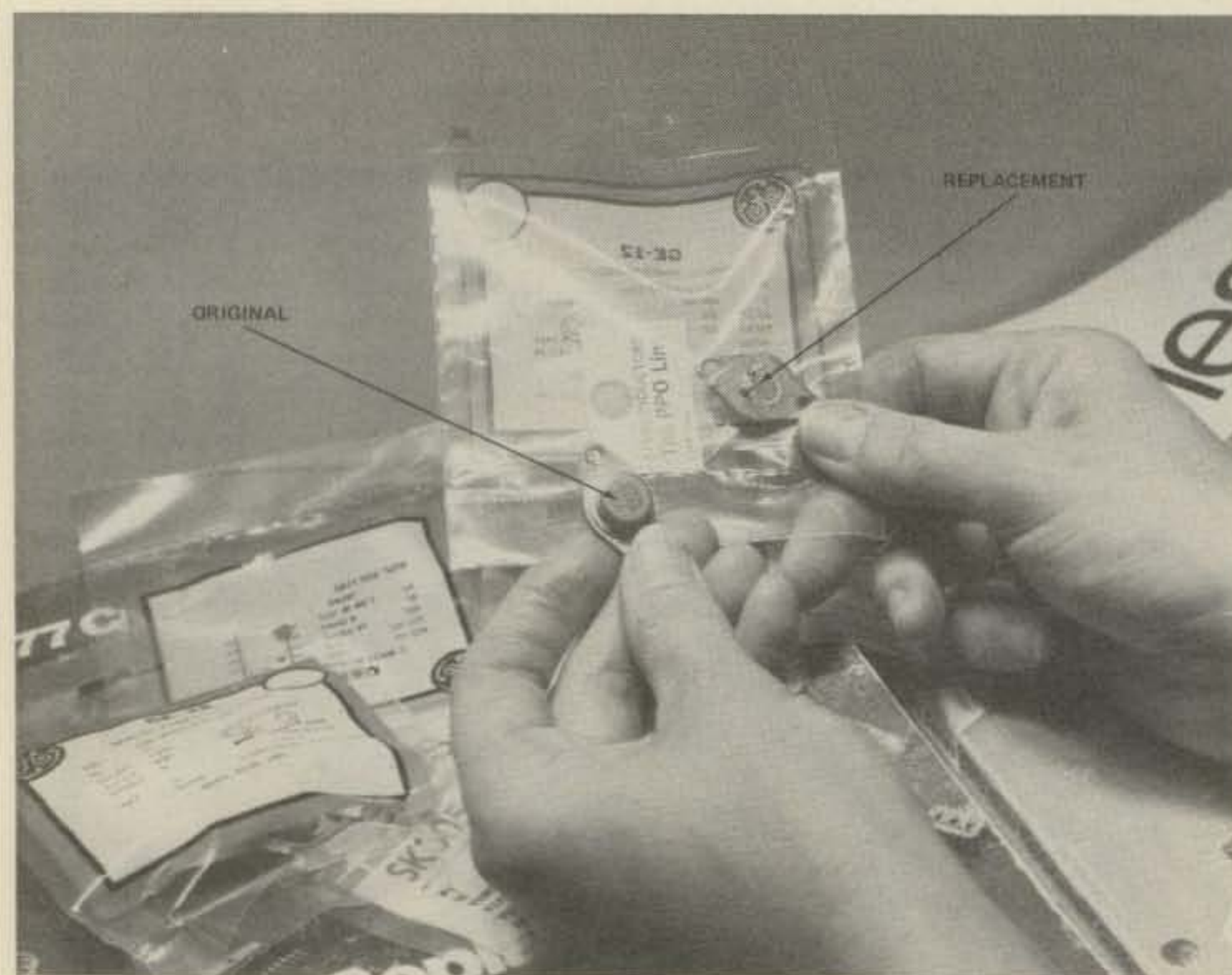
Photo 9 - When the original transistor is not available, most transistors can be replaced with a universal replacement. Check the original numbers within the universal transistor replacement guide.
