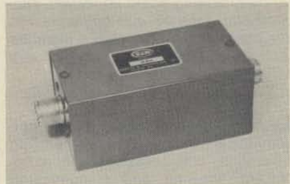
Lowpass filter attenuates h.f. signal harmonics that, if radiated, could interfere with local television reception. B&W unit shown here handles 100 watts r.f. and has a cutoff at 30 MHz. (Photo courtesy Barker and Williamson)
