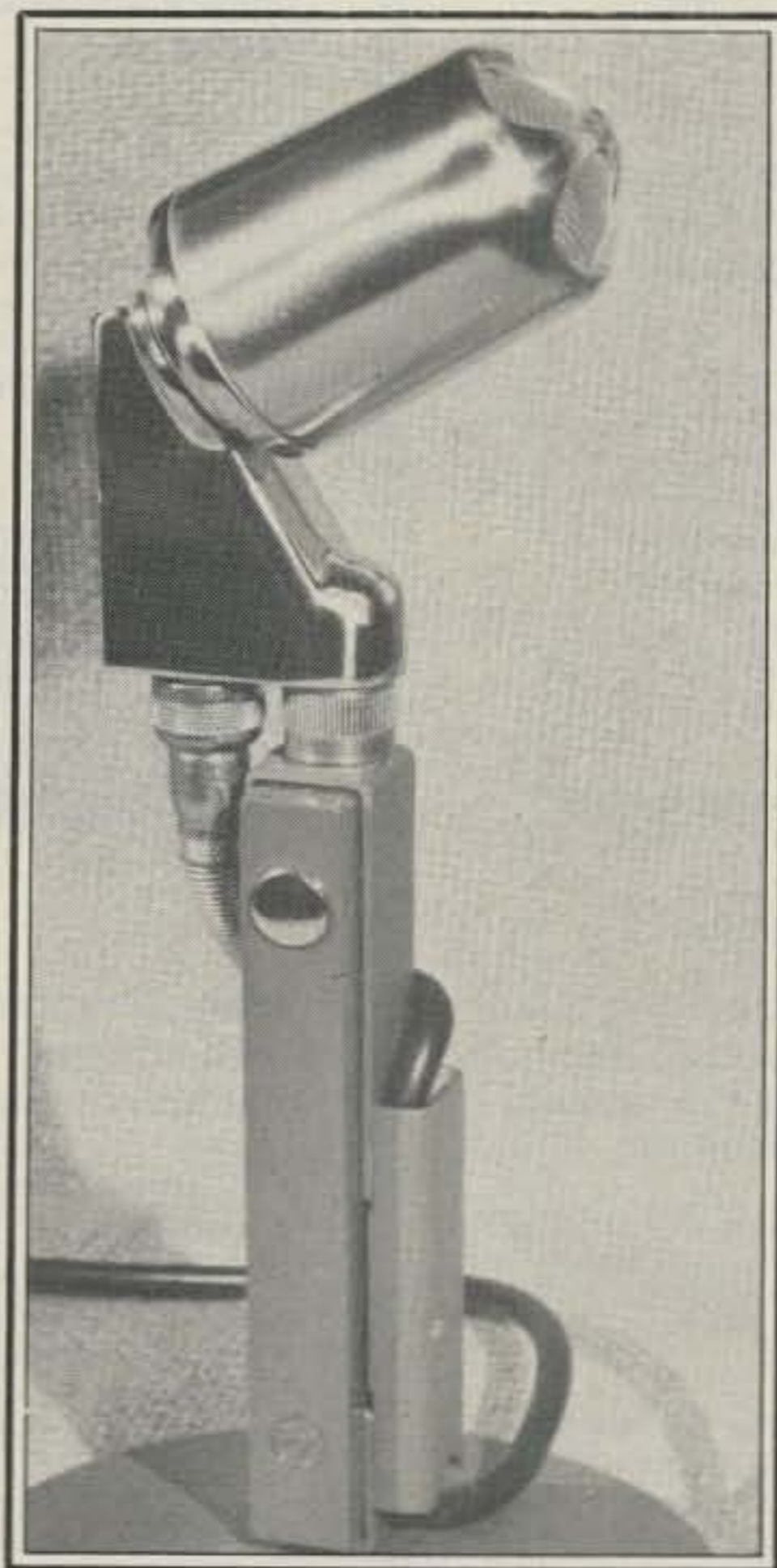
The Electro-Voice stand and microphone, with the touch-button installed near the top of the press-bar. Body capacity activates the control circuit, and the button and bar are stationary.
