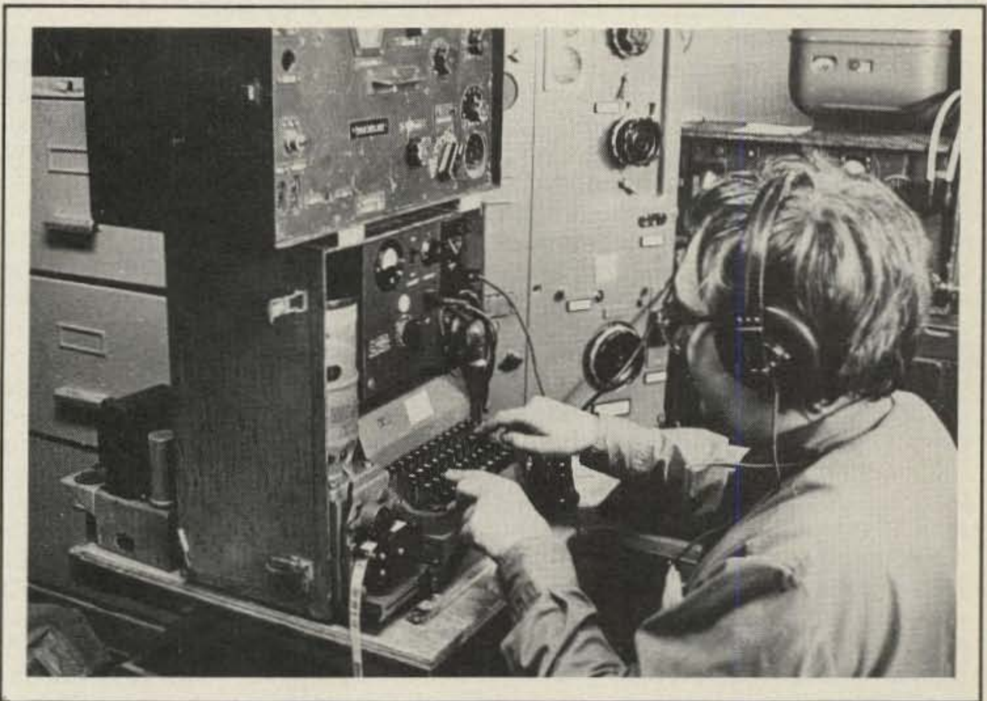
Photo 2- Here PA0AOB is typing on a "Hellschreiber," an ingenious system of teletyping over radio. The system was extensively used by the German forces during WW II. It is now commercially obsolete. But a group of enthusiastic European amateurs have revived the system and are using it in regular skeds on the h.f. and v.h.f. bands.
