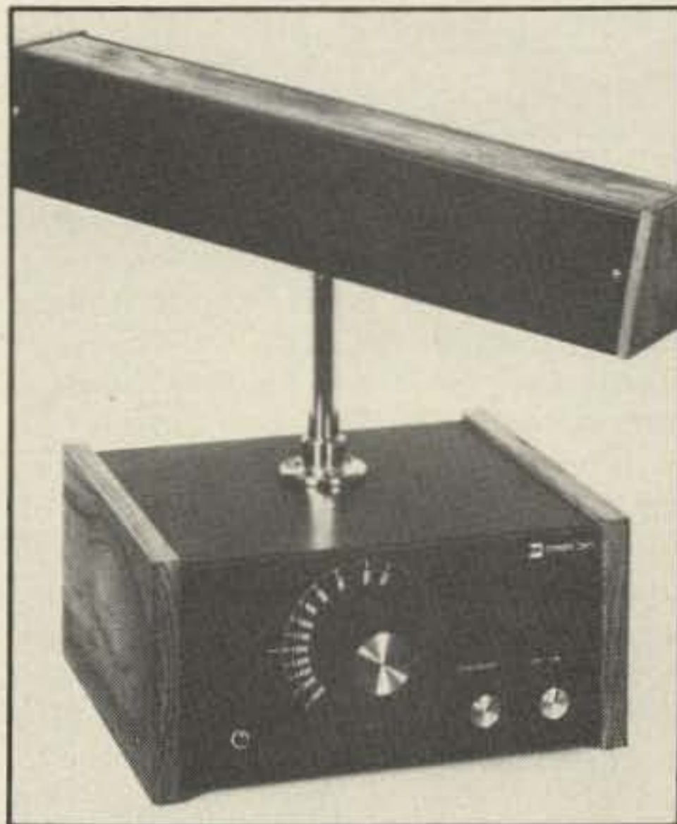
A close cousin to the dipole is the ferrite rod directional loop, especially popular as an m.f./h.f. receiving antenna. McKay Dymek loop shown here contains a FET two-stage amplifier and it's designed to minimize interference and background noise prevalent in m.f. reception. This particular antenna is designed for broadcast band use, but higher-frequency versions are also available. Commercial quality receiving loops are also sold by Palomar Engineers. (Photo courtesy McKay Dymek)
