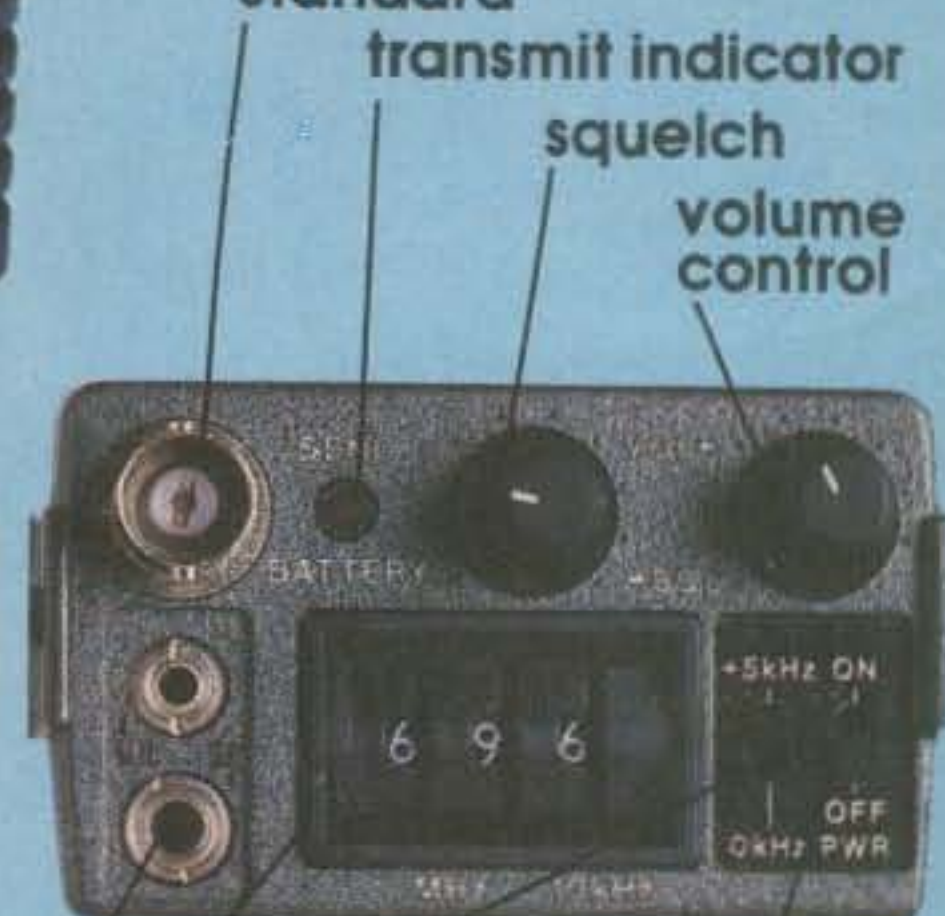
transmit indicator squelch volume control on/off 5 khz channel selection 10 khz channel selection speaker/mic jack
