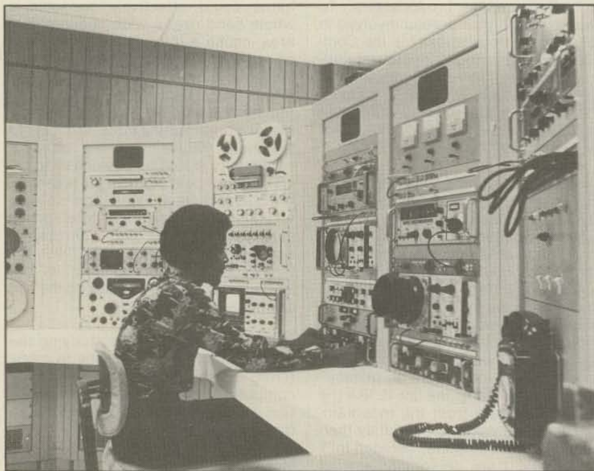
A monitoring technician makes measurements using a v.h.f./u.h.f. receiver and oscilloscope.
