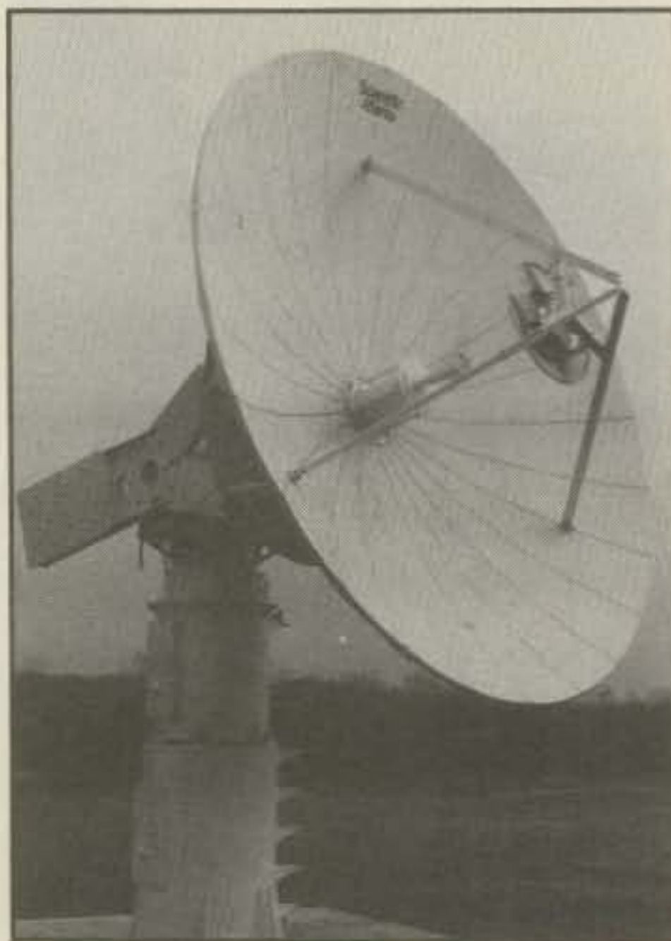
The FCC's satellite monitoring facility at the monitoring station in Laurel, Maryland is equipped with a 5 meter dish antenna capable of receiving signals from 1 to 12 GHz.
