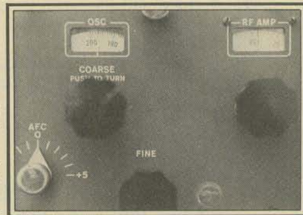
Fig. 4- Dial calibration is in channel designators; add 199.5 for MHz.
