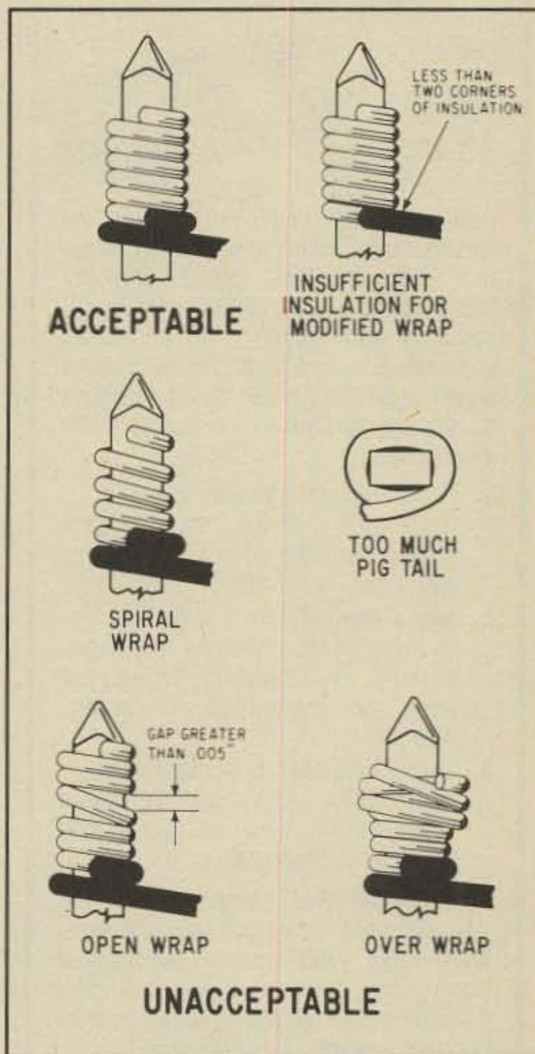
Fig. 2- The acceptable methods of a modified wrap along with the unacceptable methods of wire wrapping.
