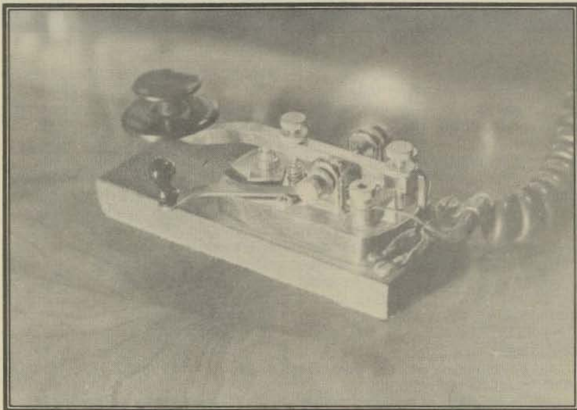
The modified Nye telegraph key as described in the text.
