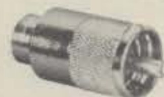
Model 370-9 PL-259 Connector for use with RG-8 Coax Cable. Mates with SO-239 Connectors. UHF Type.
